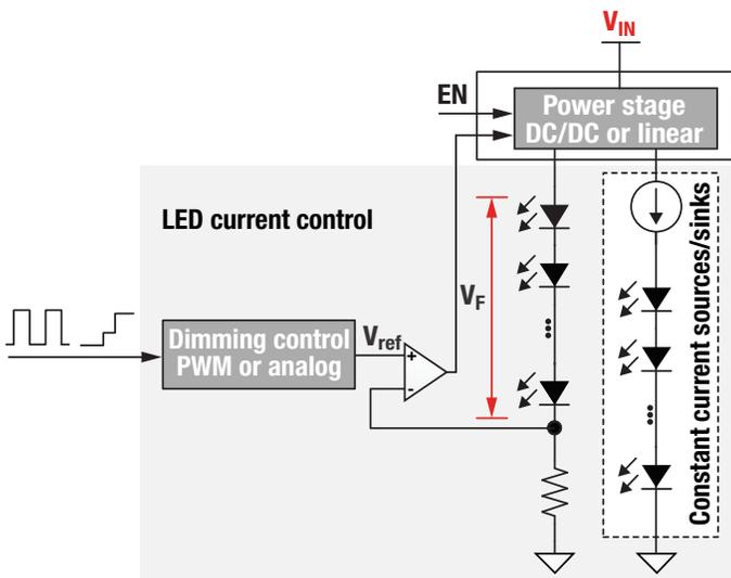
Figure 7. Typical block diagram for LED illumination.
