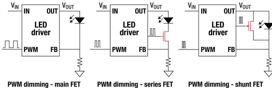
Figure 10. LED illumination PWM dimming methods.
