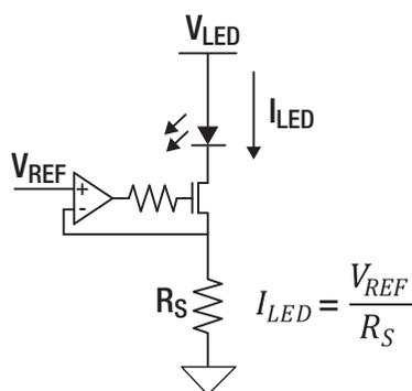
**Figure 4.** An LED driving circuit with constant current.
