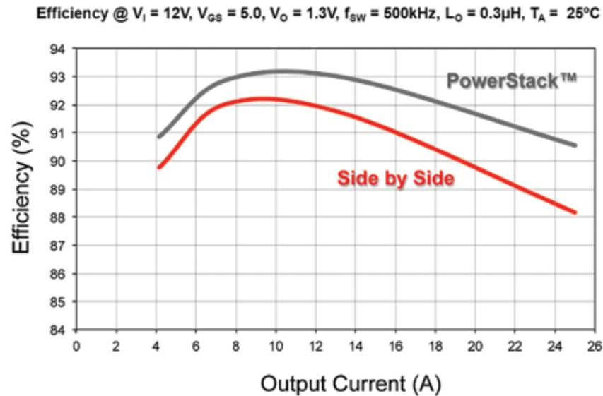
Figure 5: Power efficiency curves for PowerStack and a discrete two-MOSFET implementation.
