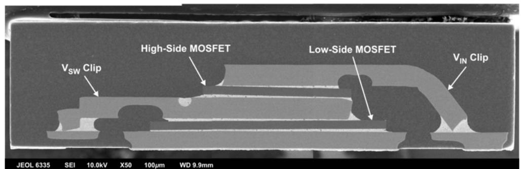
Figure 2: A cross-section of a device using a PowerStack package.
