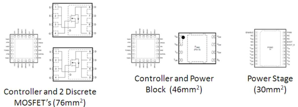
Figure 3: Board space savings for a typical circuit resulting from PowerStack.
