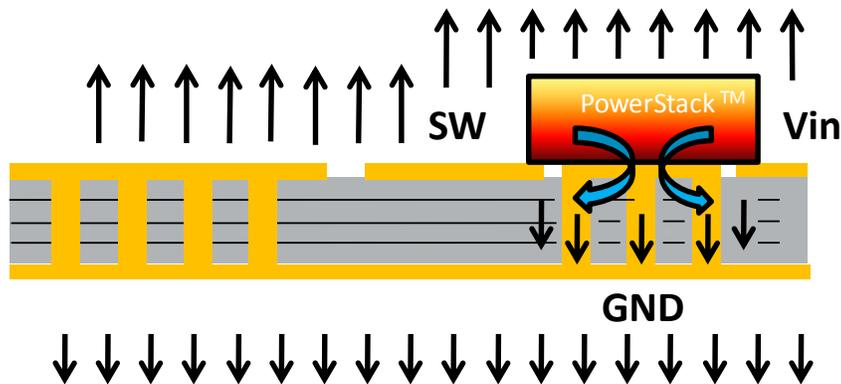
Figure 6: Optimal thermal path through grounded thermal pad of PowerStack Package.
