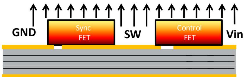
Figure 7: Limited thermal path through SW node and Vin node of side by side MOSFET's.
