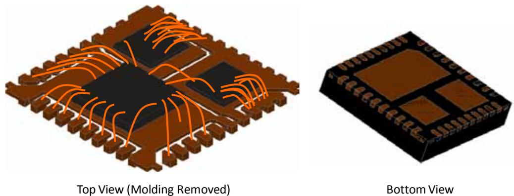
*Figure 1: A side-by-side implementation of two MOSFETs with a controller IC*
