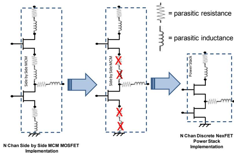
Figure 4: PowerStack delivers low parasitic losses to support high current levels and high switching frequency.
