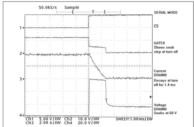
Figure 4b. Power During Off Time
