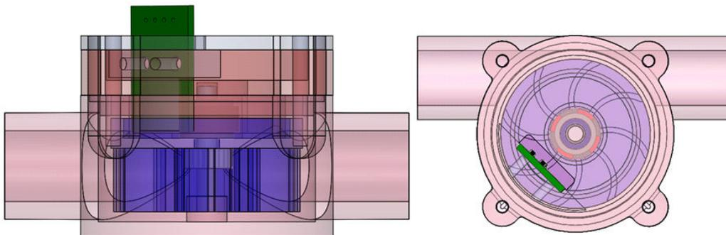
**Figure 3-8. Vertical PCB Mount**
