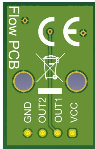
Figure 6-3. PCB Bottom Rendering
