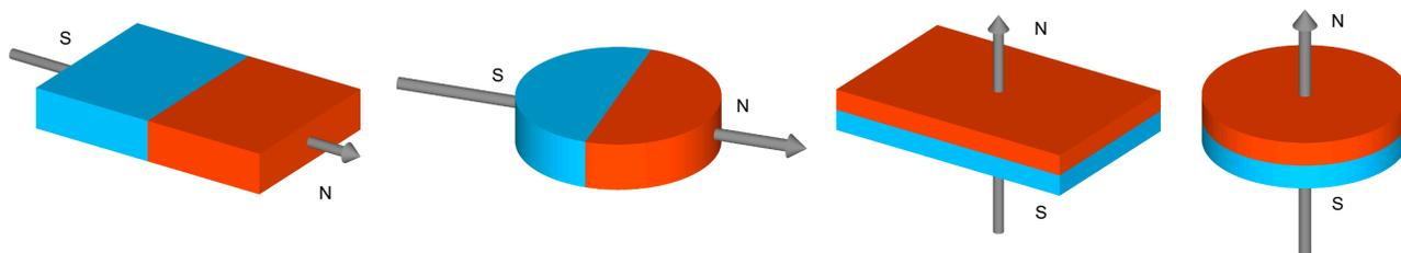
**Figure 2-1. Cylinder and Block Magnet**
