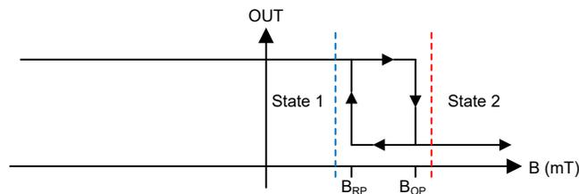
**Figure 2-3. Unipolar Switch Operation**
