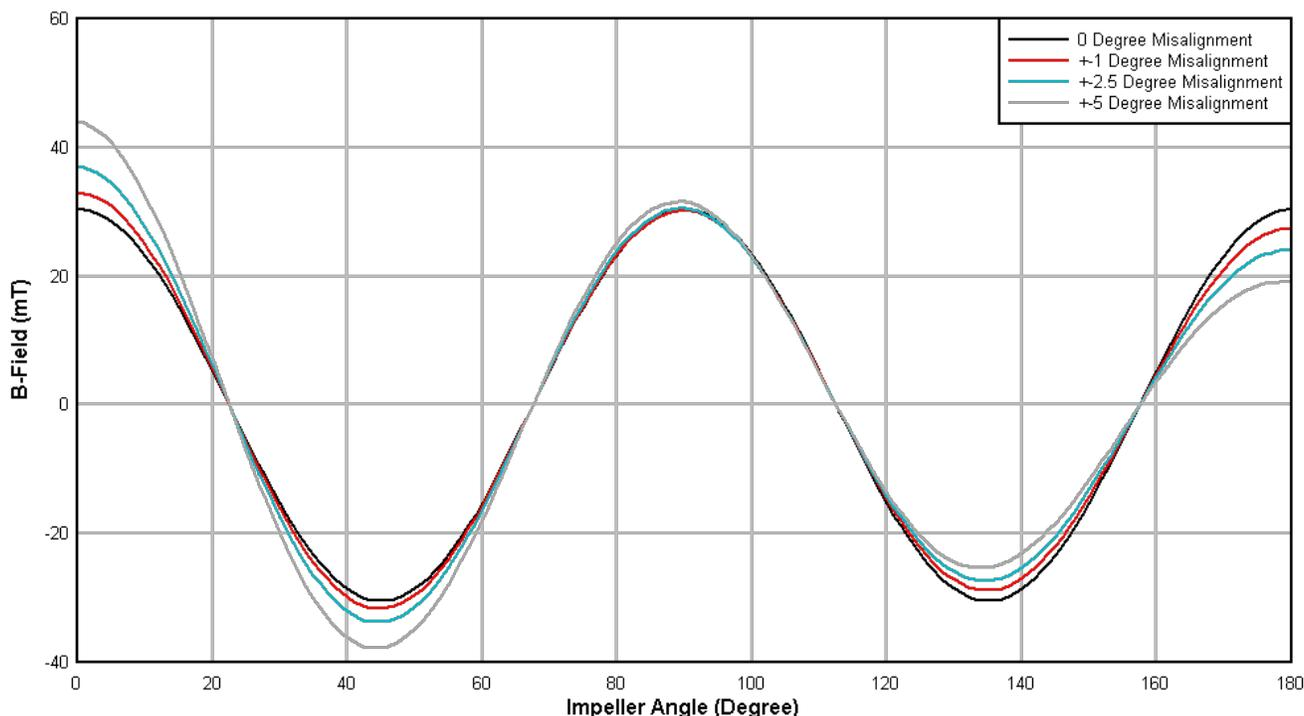
Figure 5-1. Misalignment Simulation
