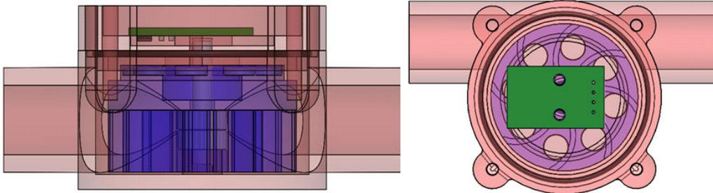
**Figure 3-7. Horizontal PCB Mount**
