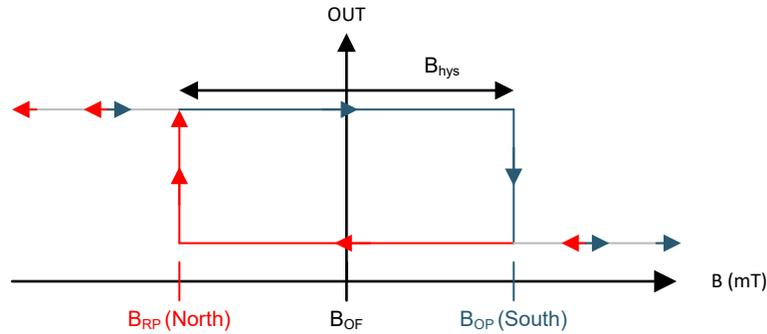
Figure 2-5. Latch Operation
