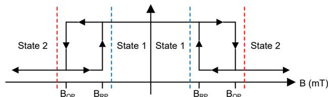
**Figure 2-4. Omnipolar Switch Operation**
