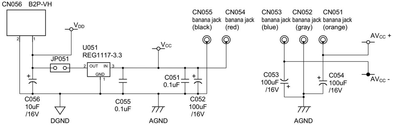
Figure 2-2. DEM-DAI1808 Regulator and Connector
