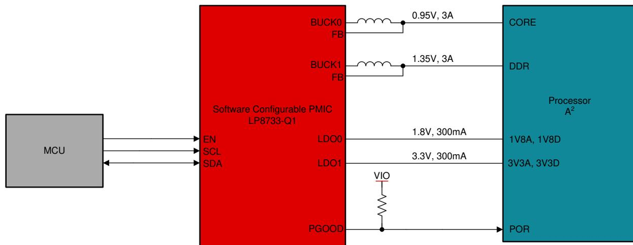
Figure 6. Higher Current PMIC Processor Power
