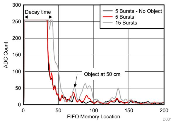
Figure 1. Burst Count Comparison for Object at 50 cm
