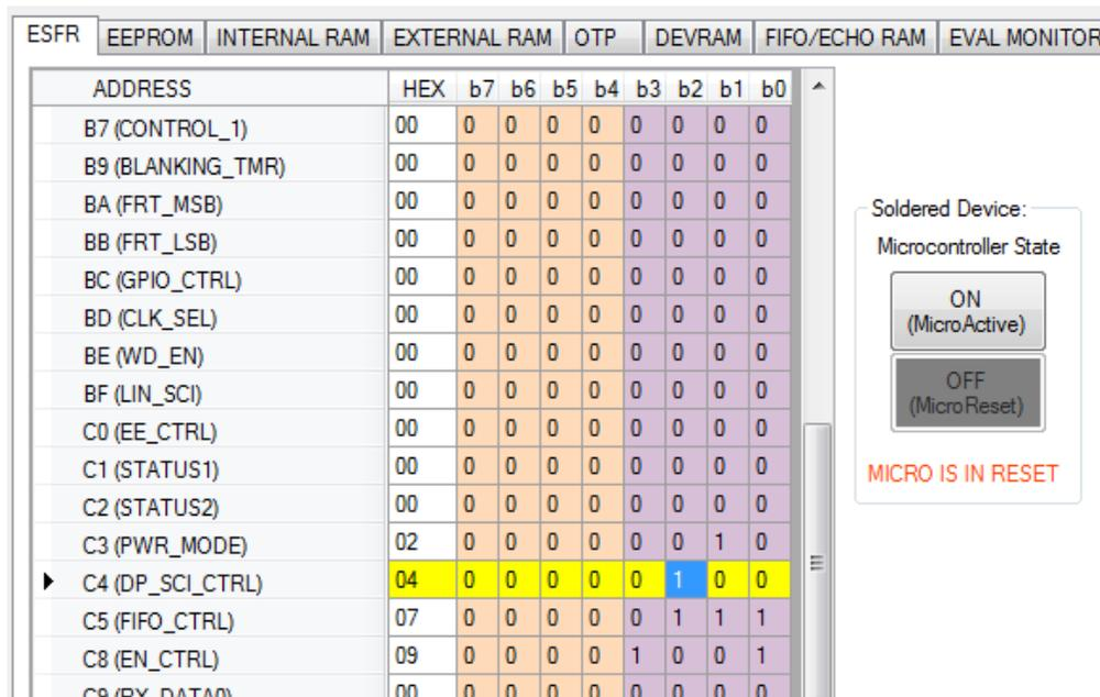
Figure 3. DP\_SCI\_CTRL Register Change in PGA450Q1EVM GUI
