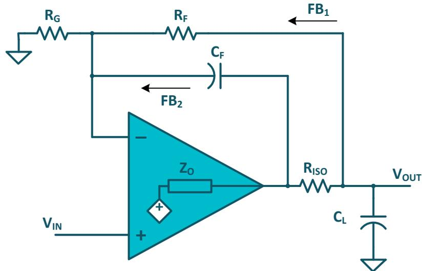
Figure 1. In-Loop Compensation: Circuit for Capacitive Load Drive
