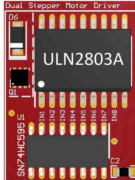
Figure 15. BoosterPack With ULN2803A
