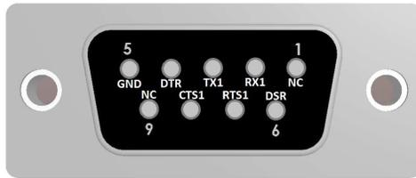
**DB9 Connector Pinout**
