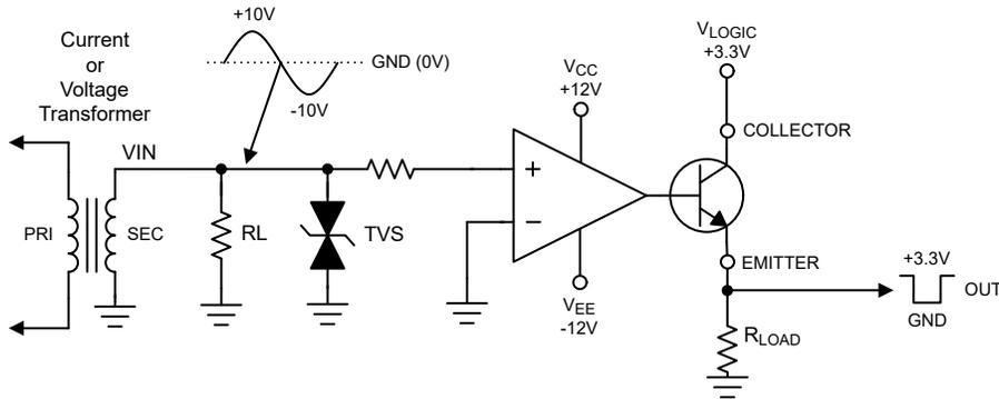
Figure 2-6. Bipolar Input With Open Emitter Output Example
