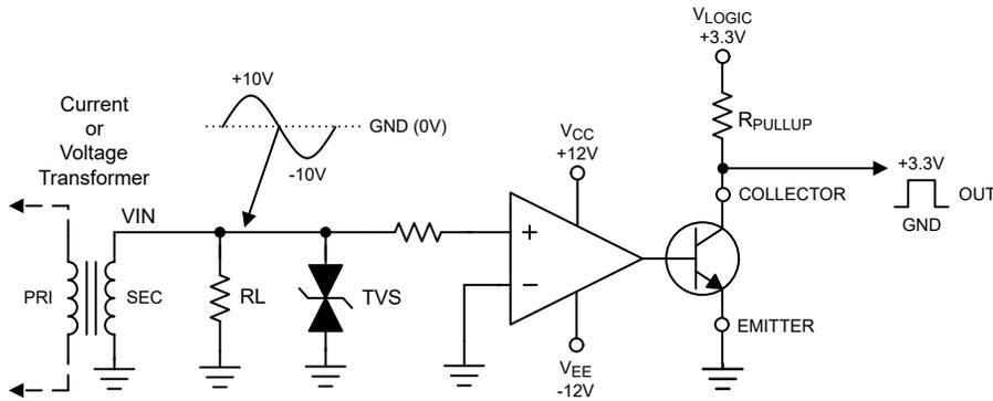
Figure 2-5. Bipolar Input Using Open Collector Output Example
