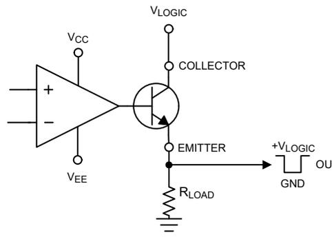
Figure 2-4. Open Emitter Configuration
