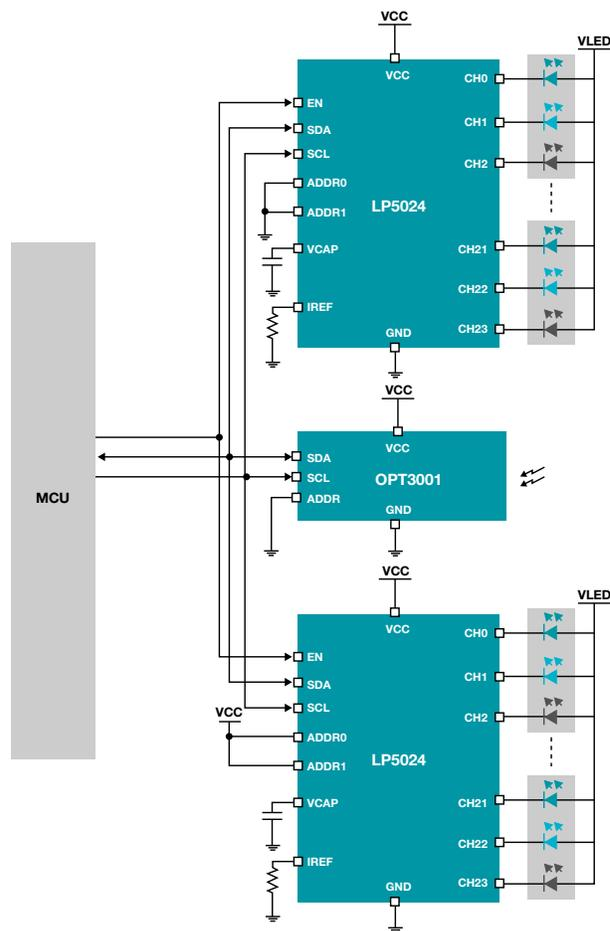
**Figure 6.** Various LED ring lighting patterns reference design.
