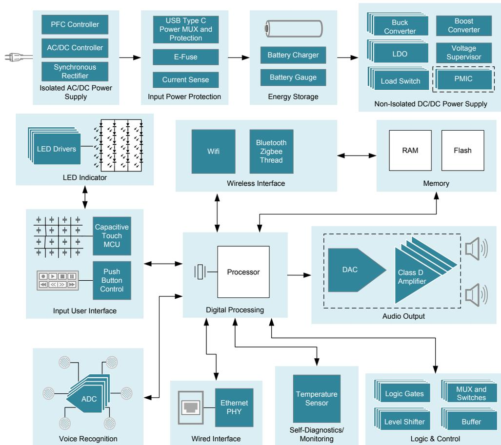
Figure 2. TI's smart speaker system block diagram.
