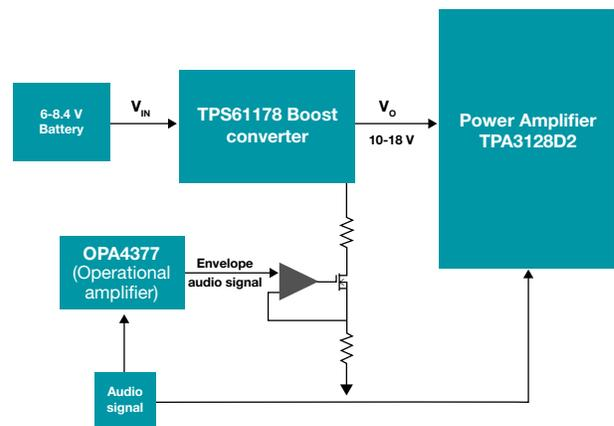
**Figure 5.** Envelope-tracking power supply reference design.
