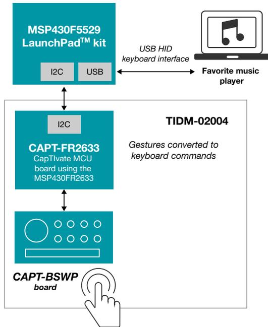
**Figure 7.** Gesture-based capacitive-touch interface reference design.
