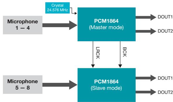
**Figure 3.** Circular microphone board reference design.
