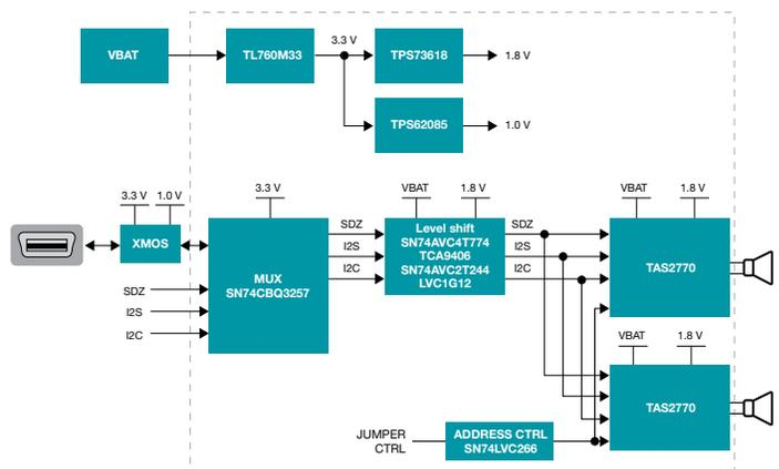
**Figure 4.** Stereo evaluation module reference design.
