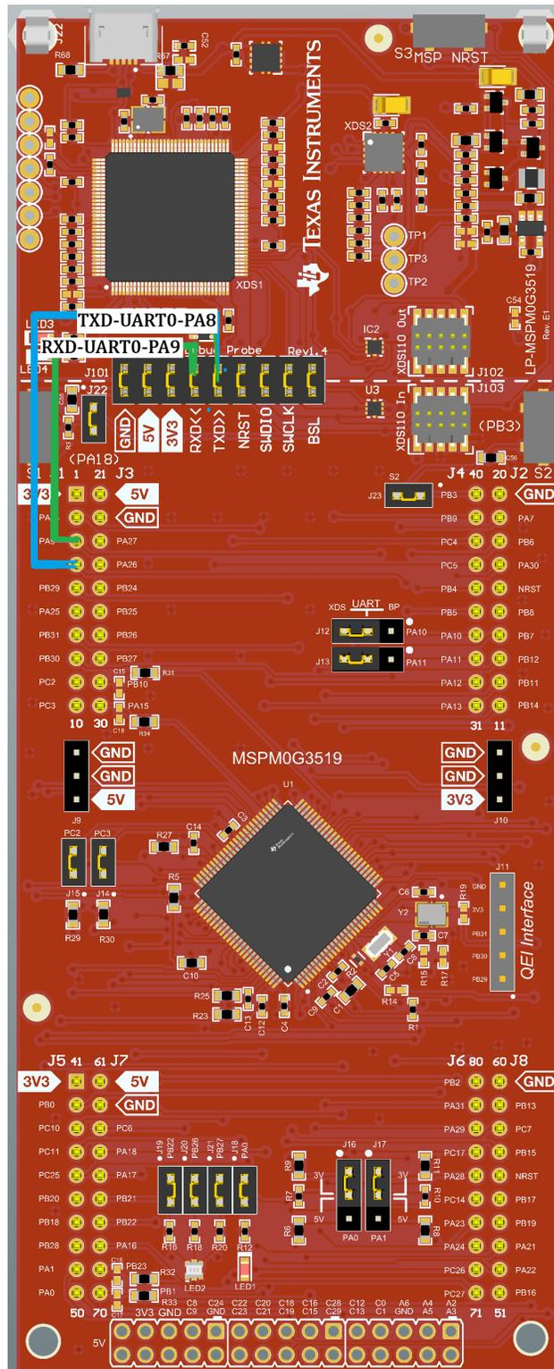
Figure 2-6. LP-MSPM0G3519 Backchannel Connection to UART0
