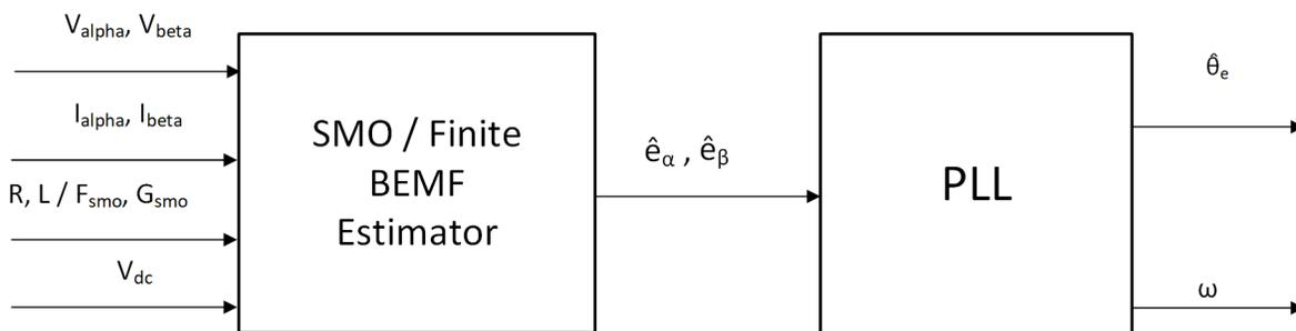
**Figure 6-11. Sensorless PMSM Rotor Position Estimation Block Diagram**
