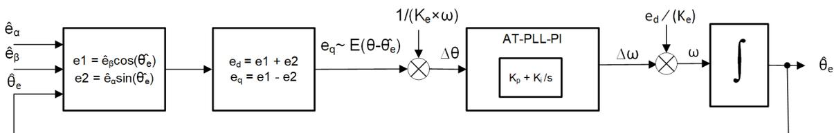
Figure 6-14. PLL-Based Rotor Speed and Position Estimation
