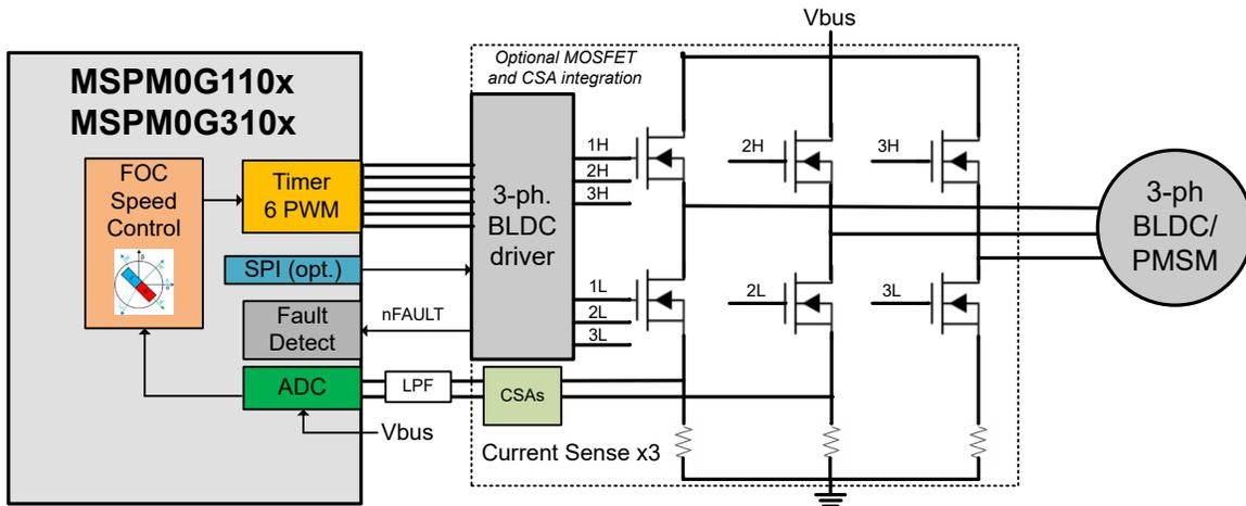
Figure 1-1. Simplified Schematic of MSPM0Gxxx + BLDC Motor Driver
