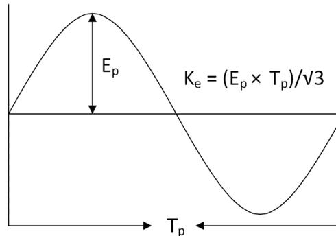
Figure 6-5. BEMF Constant Measurement
