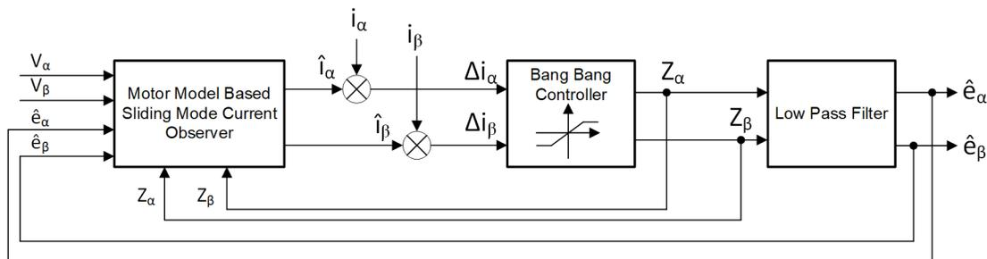
Figure 6-13. Sliding Mode Observer based BEMF Estimation
