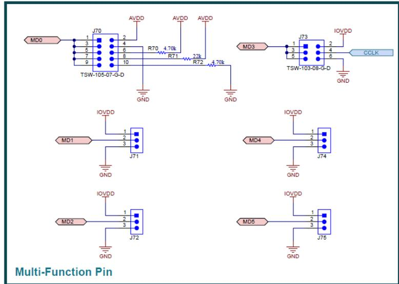
Figure 4-8. TAD5242 EVM Connectors and Supporting Circuitry Schematic
