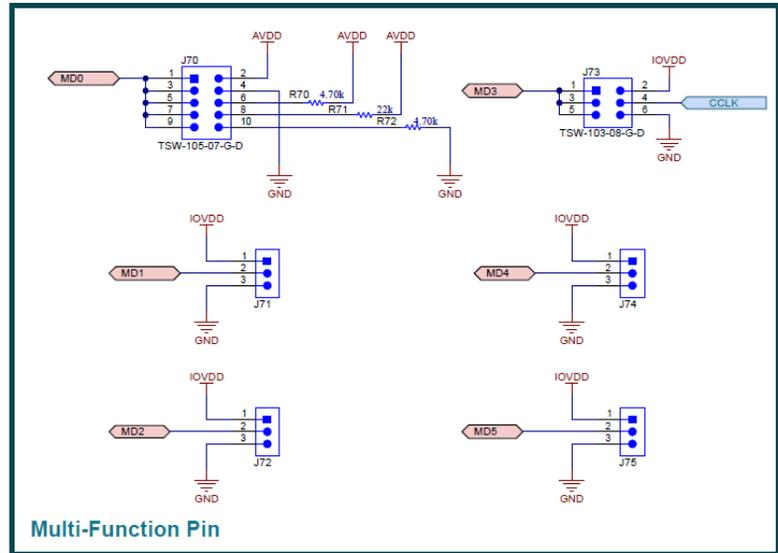
Figure 4-4. TAC5142 EVM Connectors and Supporting Circuitry Schematic
