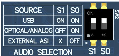
**Figure 2-3. AC-MB USB Audio Setting**
