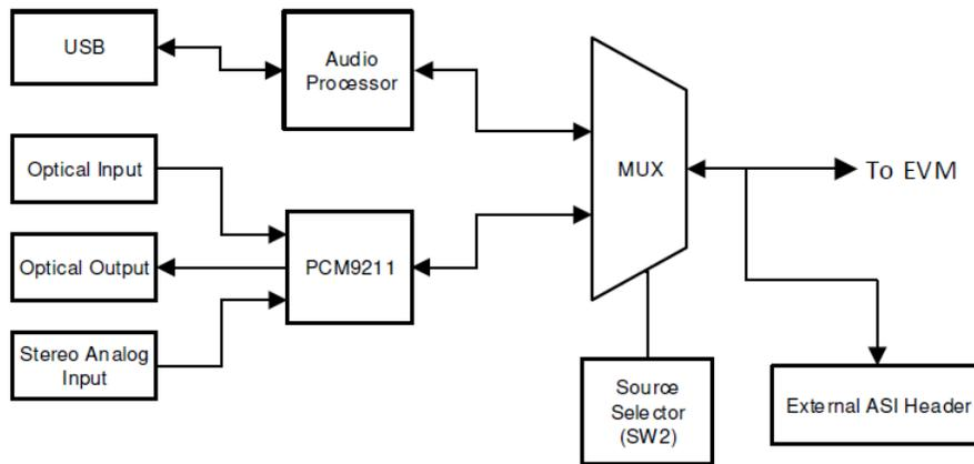
Figure 2-2. AC-MB Audio Interface Block Diagram
