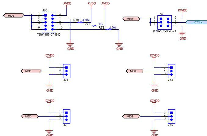
**Figure 2-11. Multi-Function Pin Setting**
