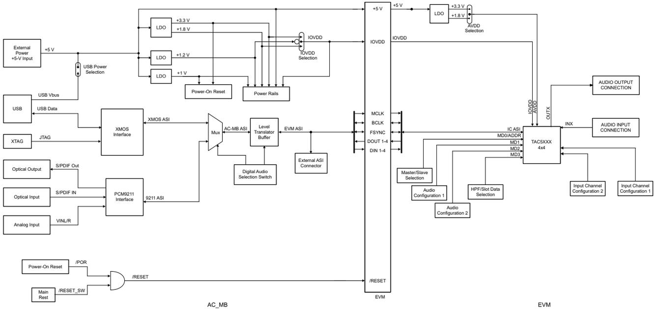
Figure 2-1. TA5x42 EVM Block Diagram
