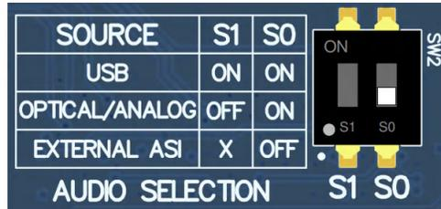
Figure 2-5. AC-MB External Audio Interface Setting
