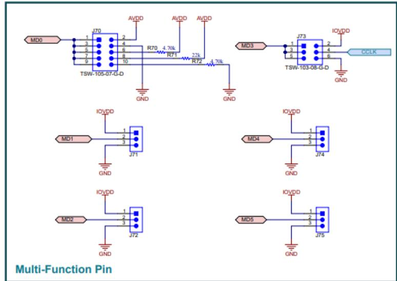
Figure 4-10. TAD5142 EVM Connectors and Supporting Circuitry Schematic
