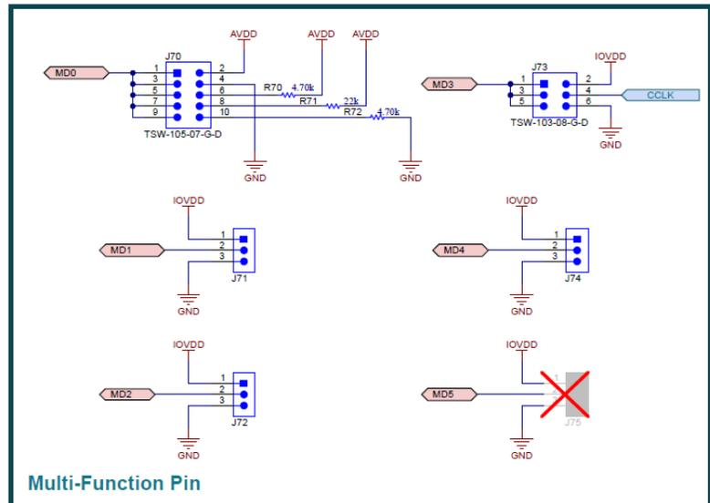
Figure 4-6. TAA5242 EVM Connectors and Supporting Circuitry Schematic
