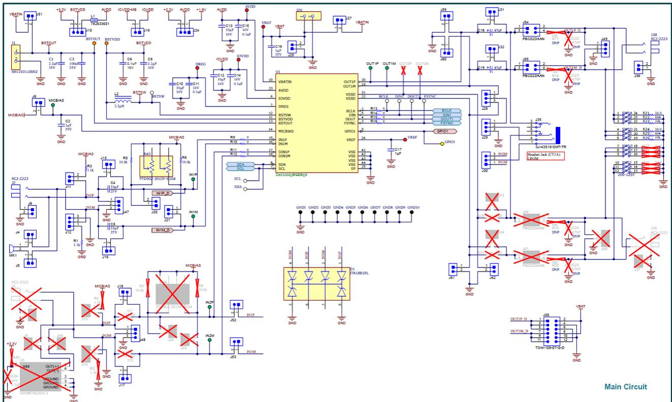
Figure 4-3. TAC5311-Q1 EVM Main DUT Schematic
