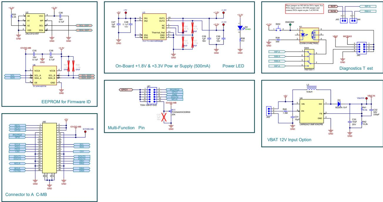
Figure 4-4. TAC5311-Q1 EVM Connectors and Supporting Circuitry Schematic
