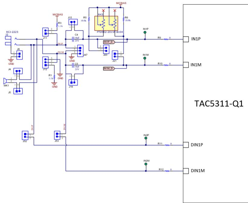
Figure 2-9. TAC5311-Q1 EVM Input Architecture for Channel 1 and DIN1P/M
