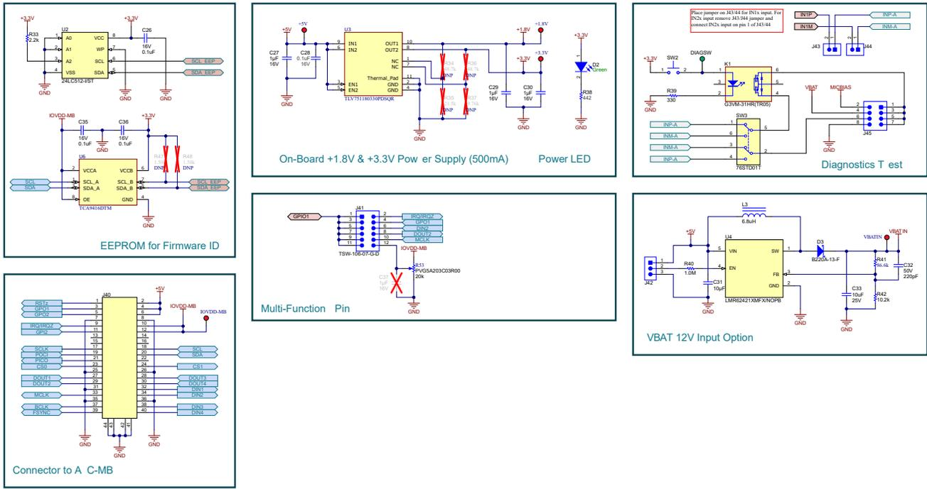
Figure 4-2. TAC5412-Q1 EVM Connectors and Supporting Circuitry Schematic
