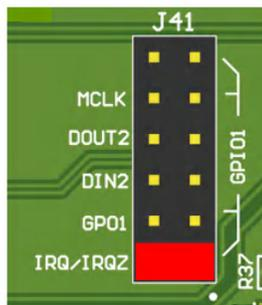
Figure 2-20. GPIO1 Configuration
