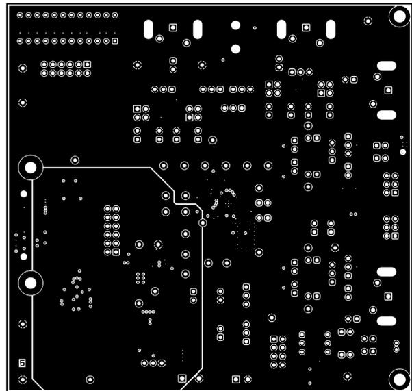
Figure 4-10. TA5x1x-Q1 EVM Power Layer 2
