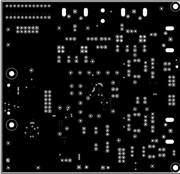
**Figure 4-11. TA5x1x-Q1 EVM Ground Layer 1**
