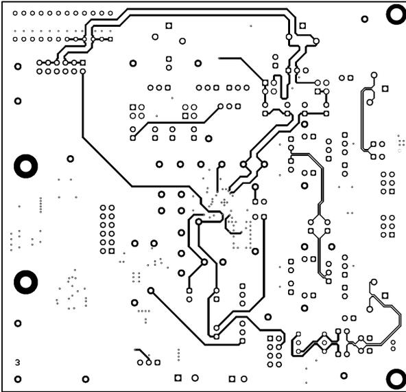
**Figure 4-13. TA5x1x-Q1 EVM Signal Layer 1**
