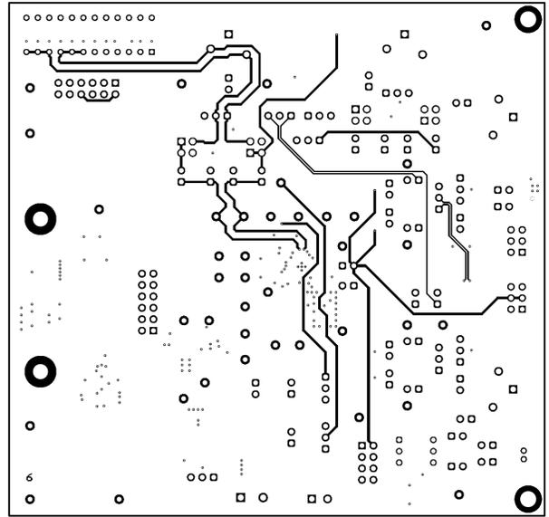
**Figure 4-14. TA5x1x-Q1 EVM Signal Layer 2**
