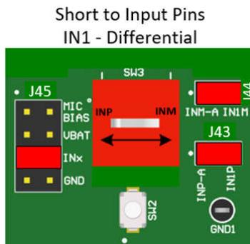
Figure 2-18. Short to Input Diagnostic Test Setup
