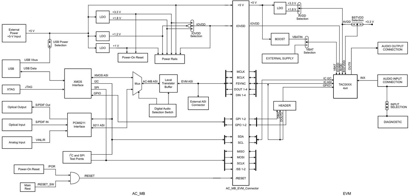
Figure 2-1. TA5x1xQ1 EVM Block Diagram
