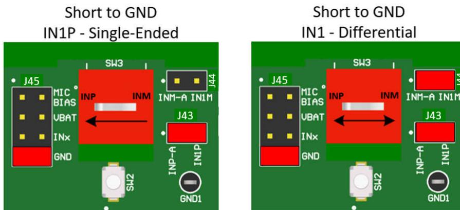
Figure 2-19. Short to Ground Diagnostic Test Setup
