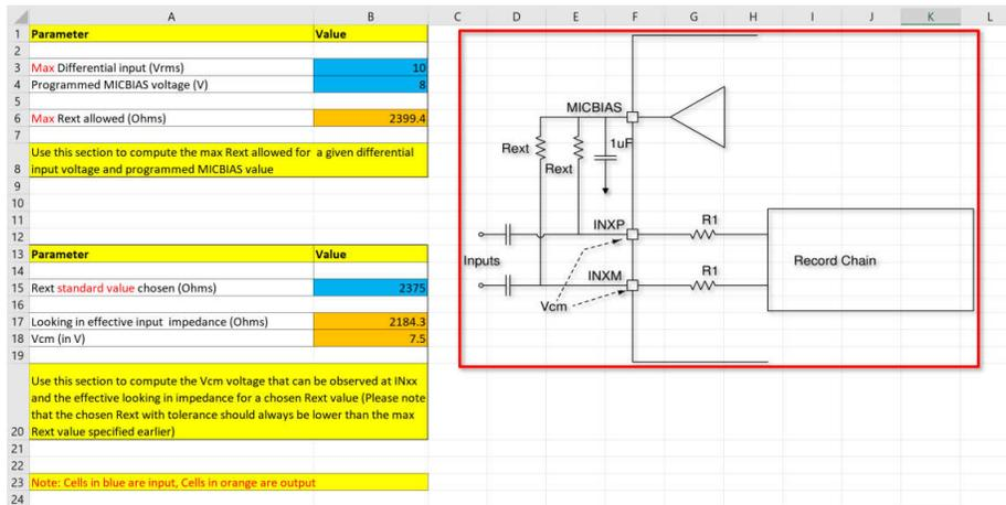
**Figure 2-10. AC-Coupled External Resistor Calculator**
