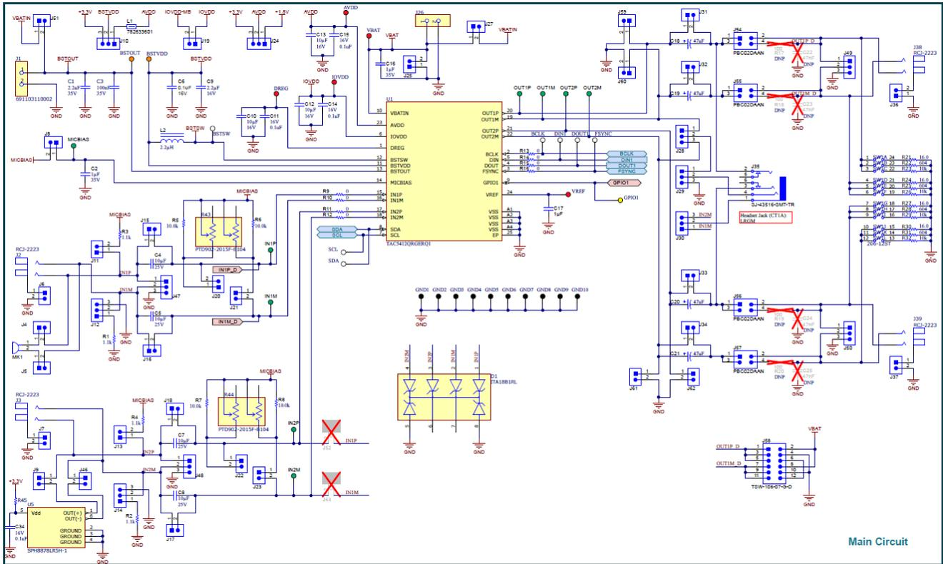
Figure 4-1. TAC5412-Q1 EVM Main DUT Schematic
