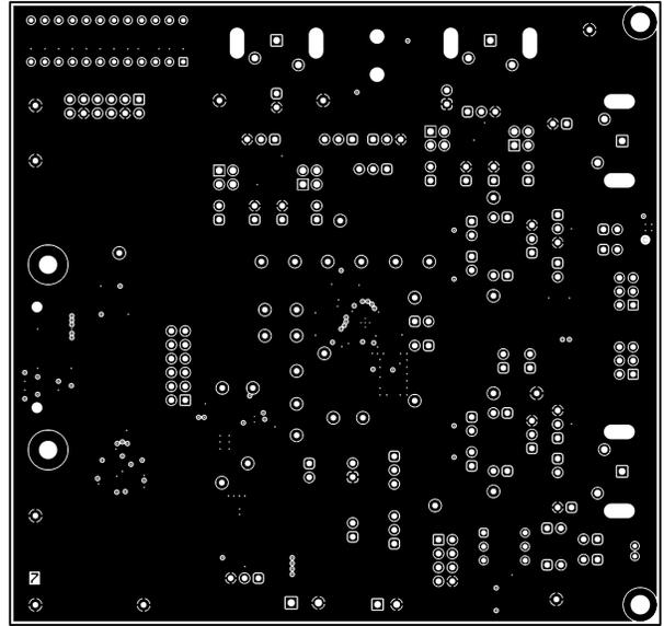
**Figure 4-12. TA5x1x-Q1 EVM Ground Layer 2**
