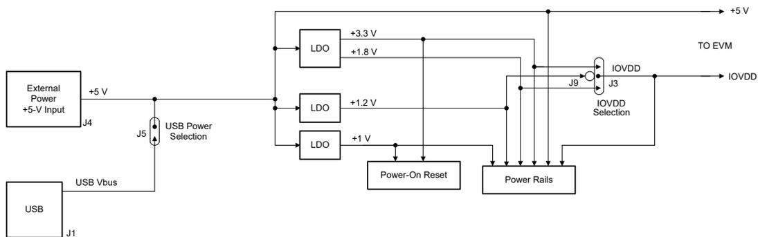
Figure 2-7. Power-Supply Distribution of the AC-MB
