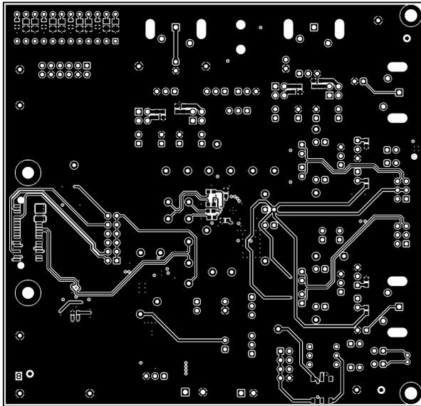
Figure 4-15. TA5x1x-Q1 EVM Bottom Layer
