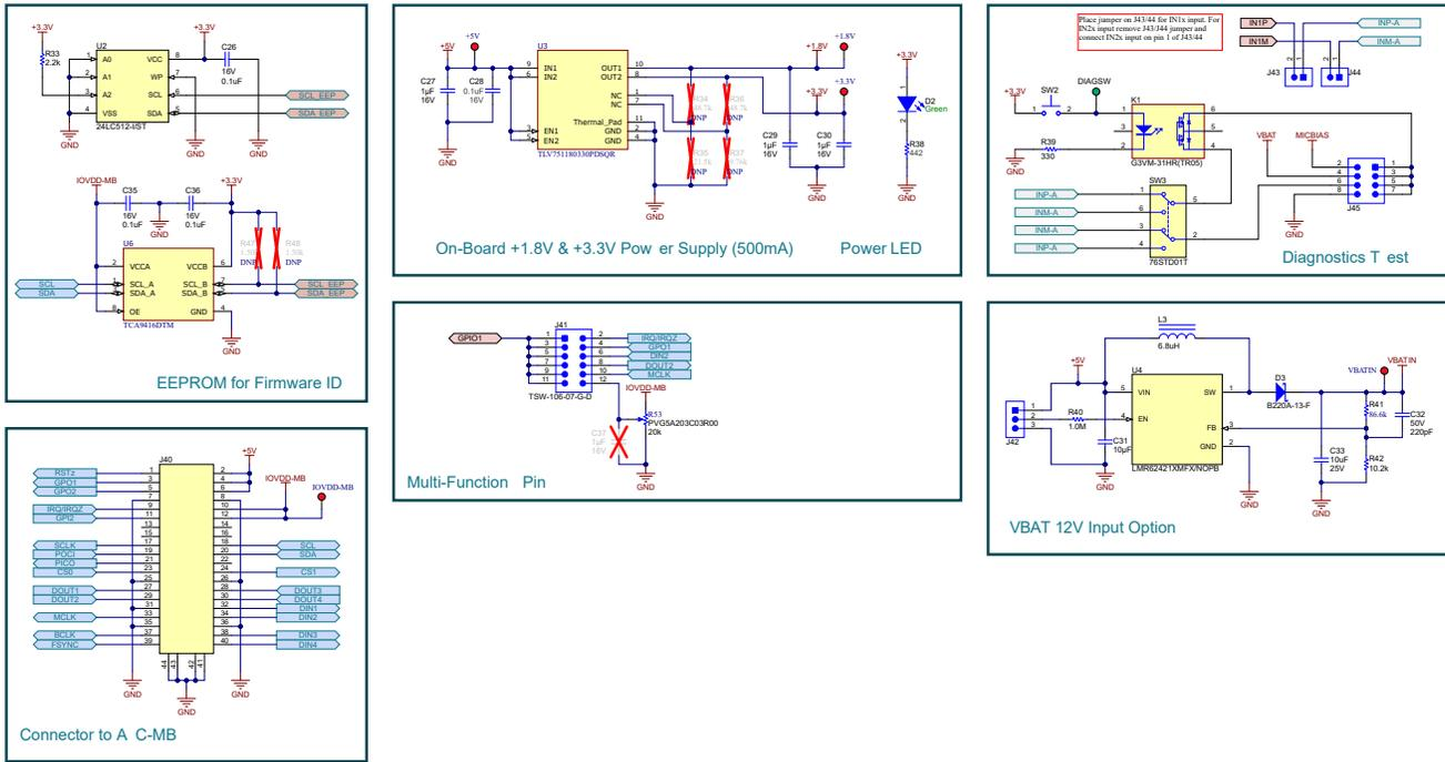
Figure 4-6. TAA5412-Q1 EVM Connectors and Supporting Circuitry Schematic
