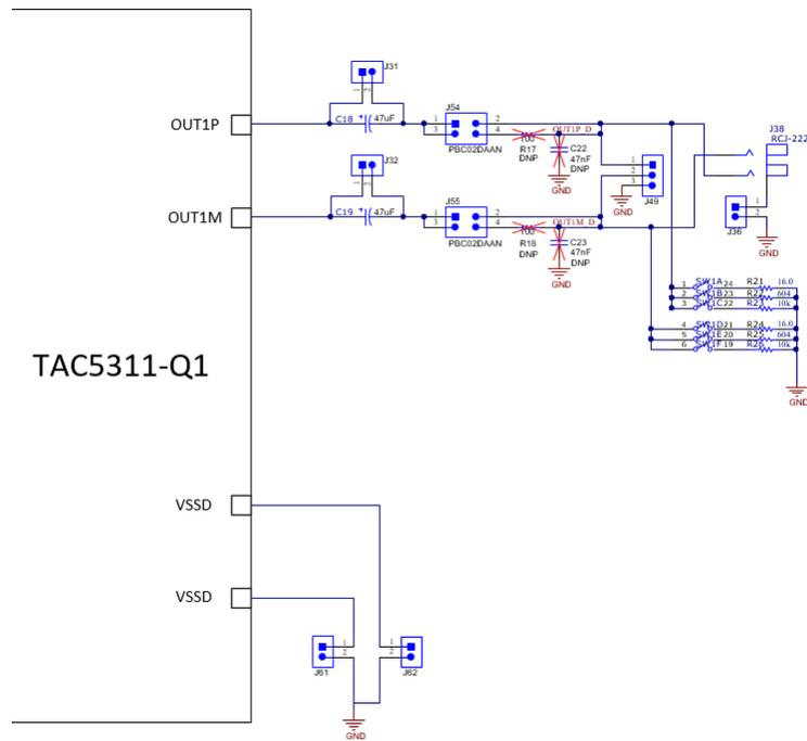
Figure 2-13. TAC5311-Q1 EVM Output Architecture for Channel 1
