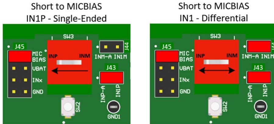
Figure 2-15. Short to MICBIAS Diagnostic Test Setup
