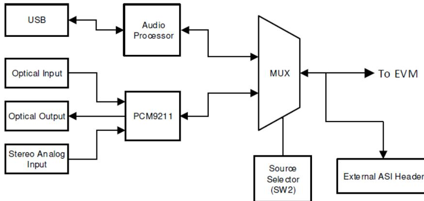
Figure 2-2. AC-MB Audio Interface Block Diagram
