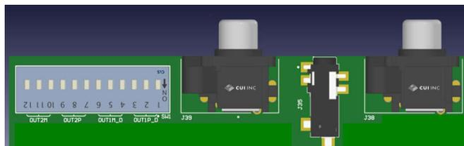
**Figure 2-12. TAC5412-Q1 Analog Output Connections**
