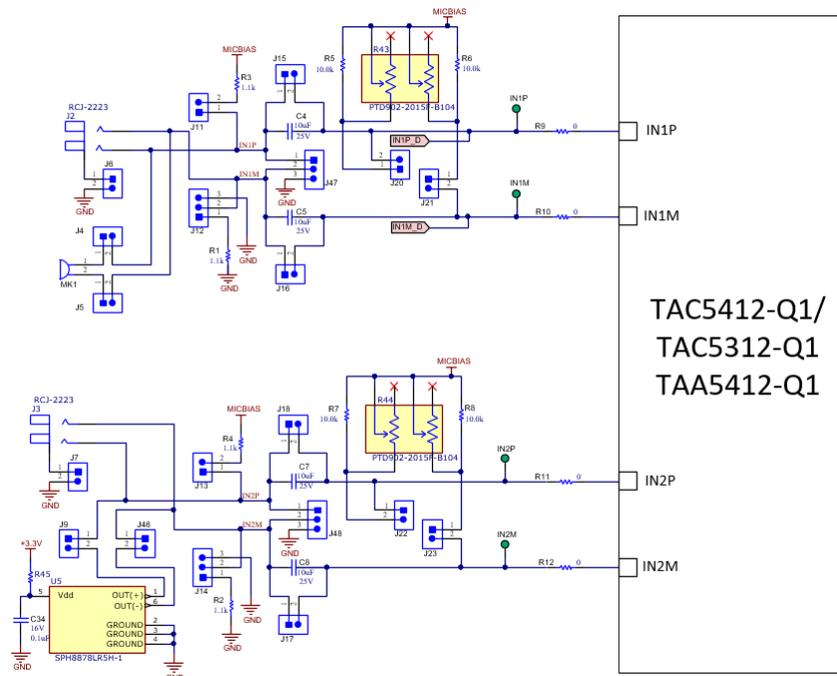
**Figure 2-8. TAC5412Q1/TAC5312Q1/TAA5412Q1 EVM Input Architecture for Channel 1 and 2**
