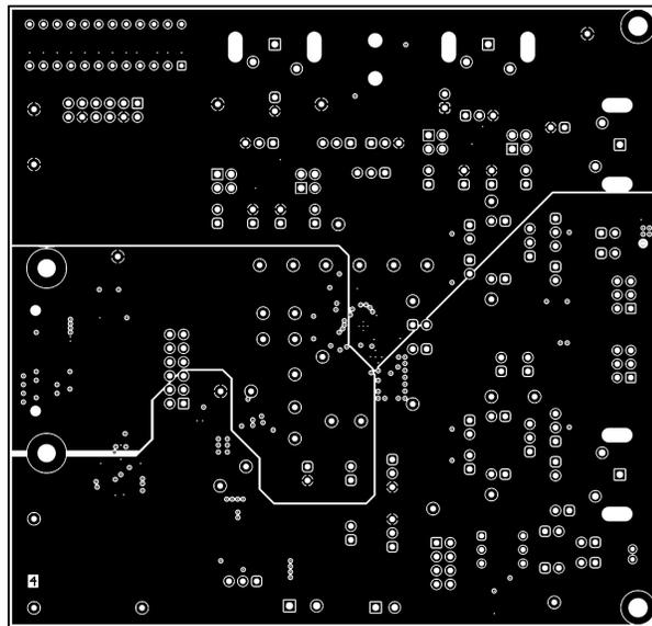
Figure 4-9. TA5x1x-Q1 EVM Power Layer 1
