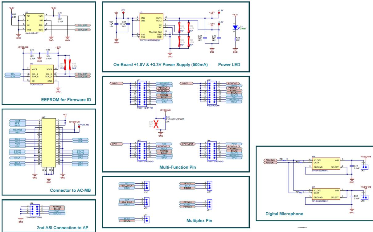
Figure 4-8. TAA5212 EVM Connectors and Supporting Circuitry Schematic
