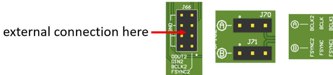
**Figure 2-17. External Audio Serial Interface Connection**
