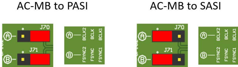
**Figure 2-16. AC\_MB Audio Serial Interface Connection**
