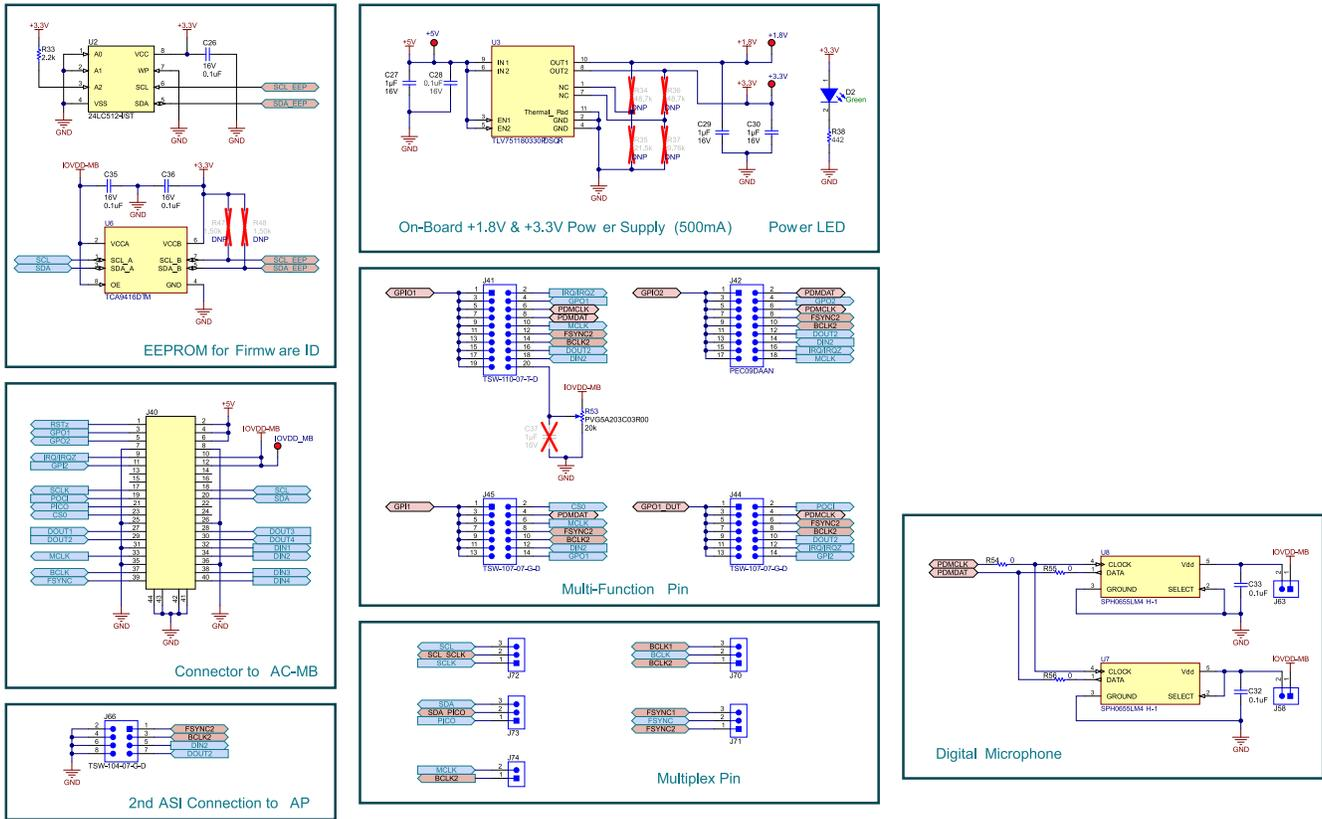
Figure 4-4. TAC5112 EVM Connectors and Supporting Circuitry Schematic
