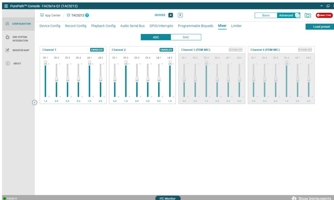
Figure 3-25. Mixer ADC Tab
