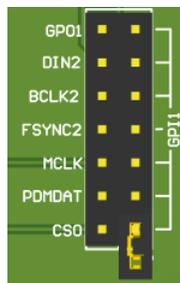
Figure 2-14. GPI1 Configuration
