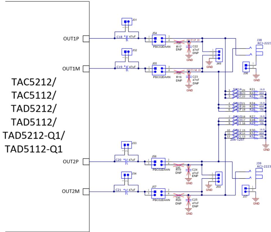
**Figure 2-9. TA<sub>x</sub>5x12 EVM Output Architecture for Channel 1 and 2**
