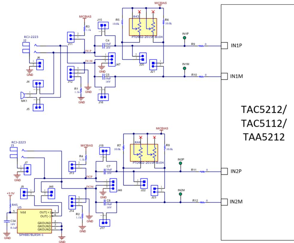
**Figure 2-8. TAC5212 and TAC5112 EVM Input Architecture for Channel 1 and 2**
