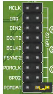
**Figure 2-13. GPIO2 Configuration**
