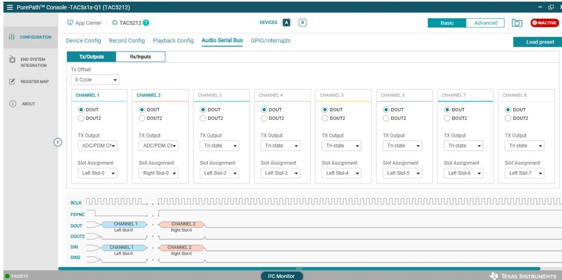
Figure 3-20. I2S Configuration Example
