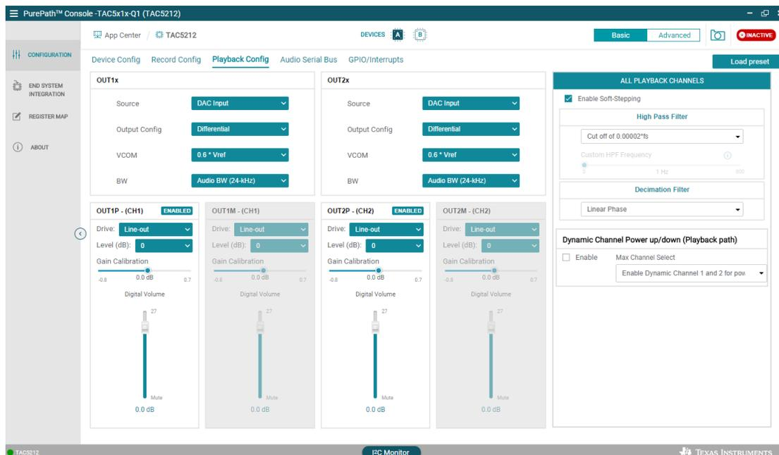
**Figure 3-13. Playback Config Tab**
