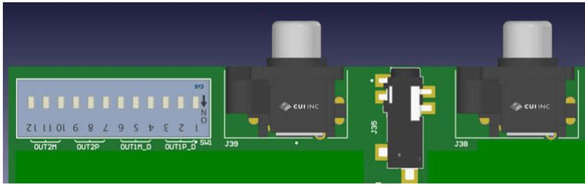
Figure 2-10. TA5x12 Analog Output Connections
