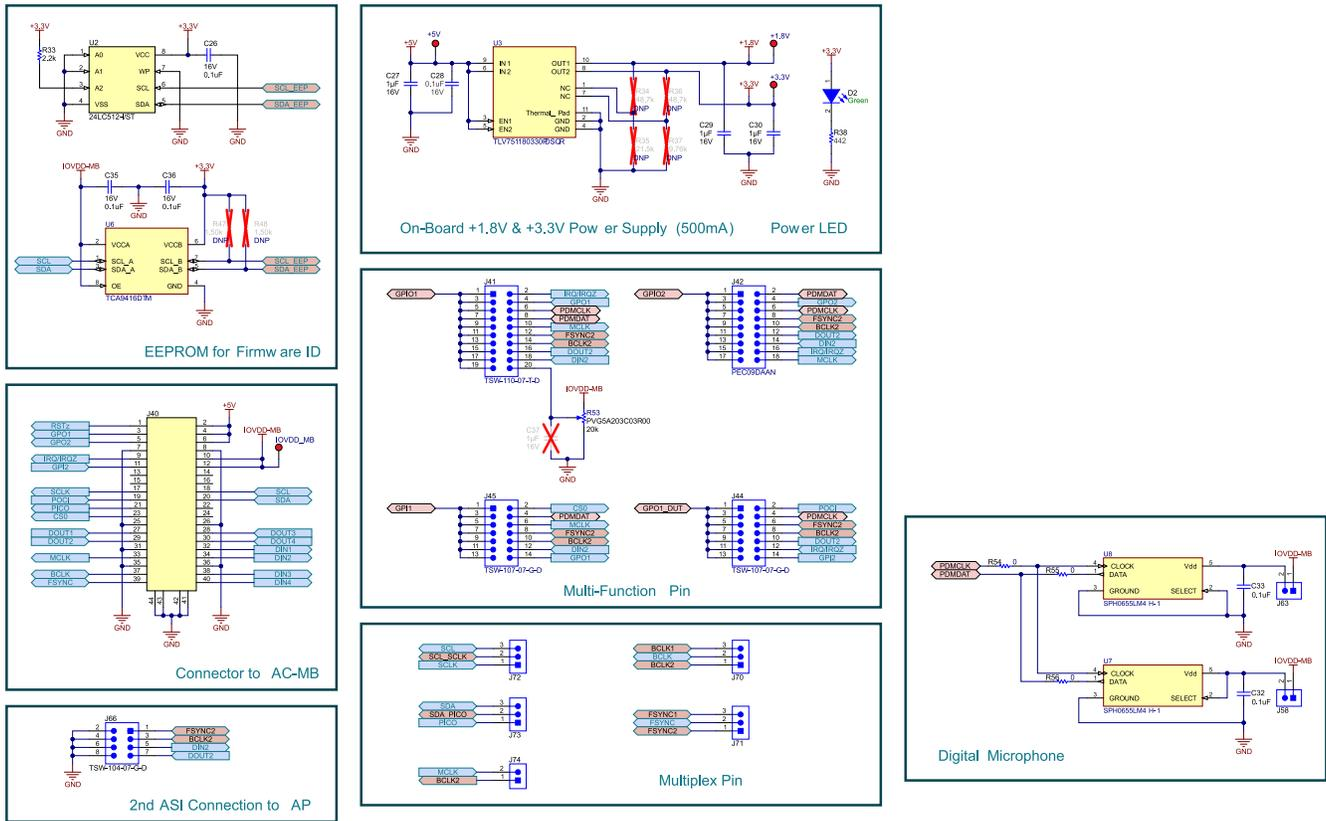
Figure 4-2. TAC5212 EVM Connectors and Supporting Circuitry Schematic
