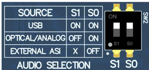
Figure 2-3. AC-MB USB Audio Setting
