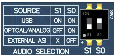
Figure 2-4. AC-MB Optical or Auxiliary Analog Audio Input Setting
