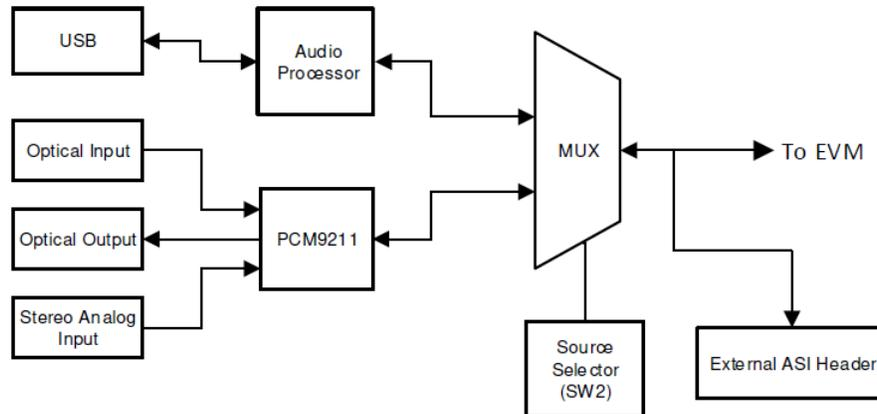
**Figure 2-2. AC-MB Audio Interface Block Diagram**
