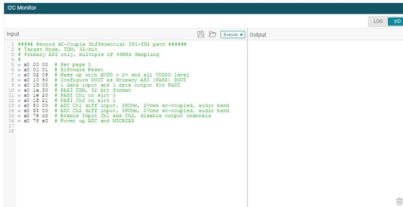
Figure 3-32. I2C Monitor I/O Window
