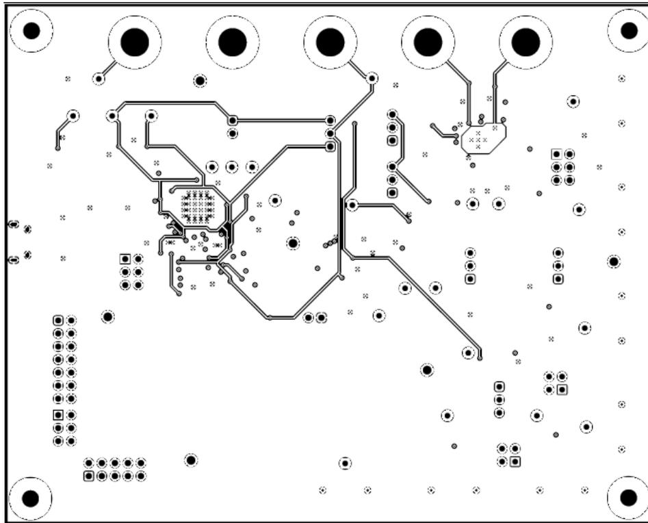
Figure 4-5. AFE882H1EVM PCB Mid Layer 2 Layout
