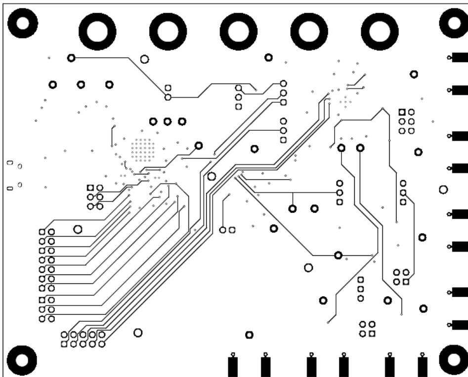
Figure 4-6. AFE882H1EVM PCB Bottom Layer Layout
