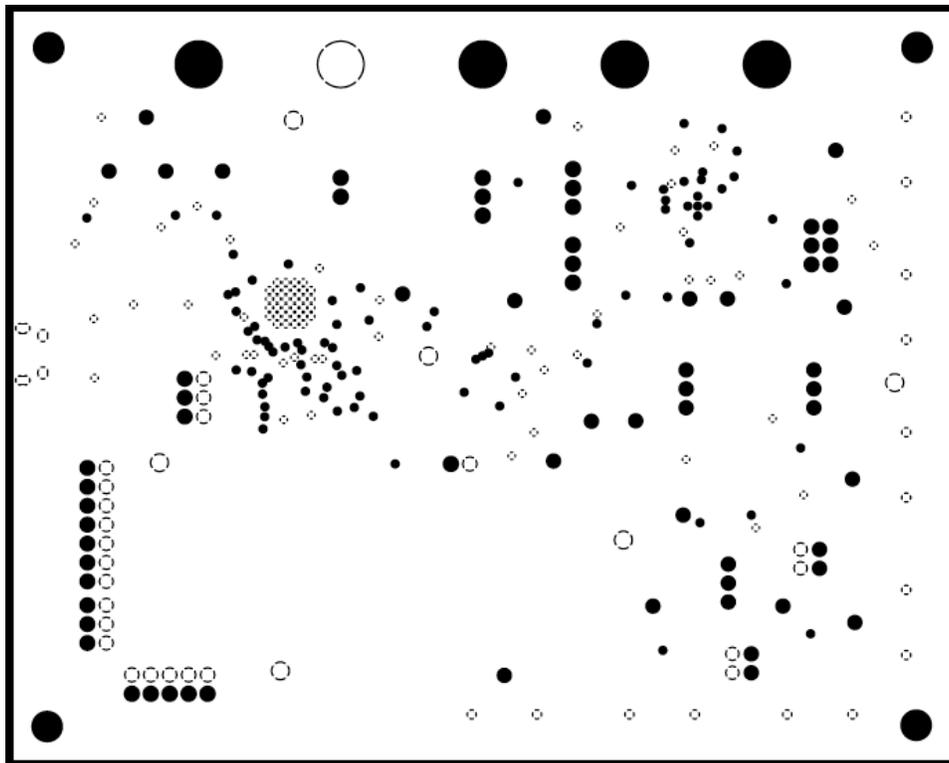
Figure 4-4. AFE882H1EVM PCB Mid Layer 1 Layout
