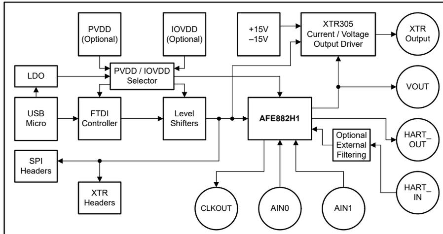
**Figure 3-1. Block Diagram for the AFE882H1EVM**
