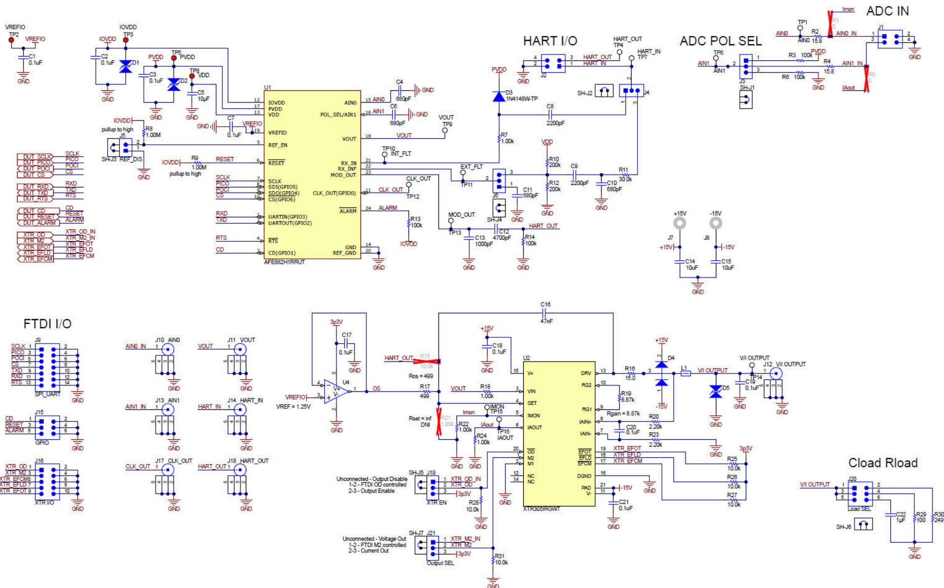
Figure 4-2. AFE882H1EVM Schematic: AFE882H1 and XTR305 Analog Output
