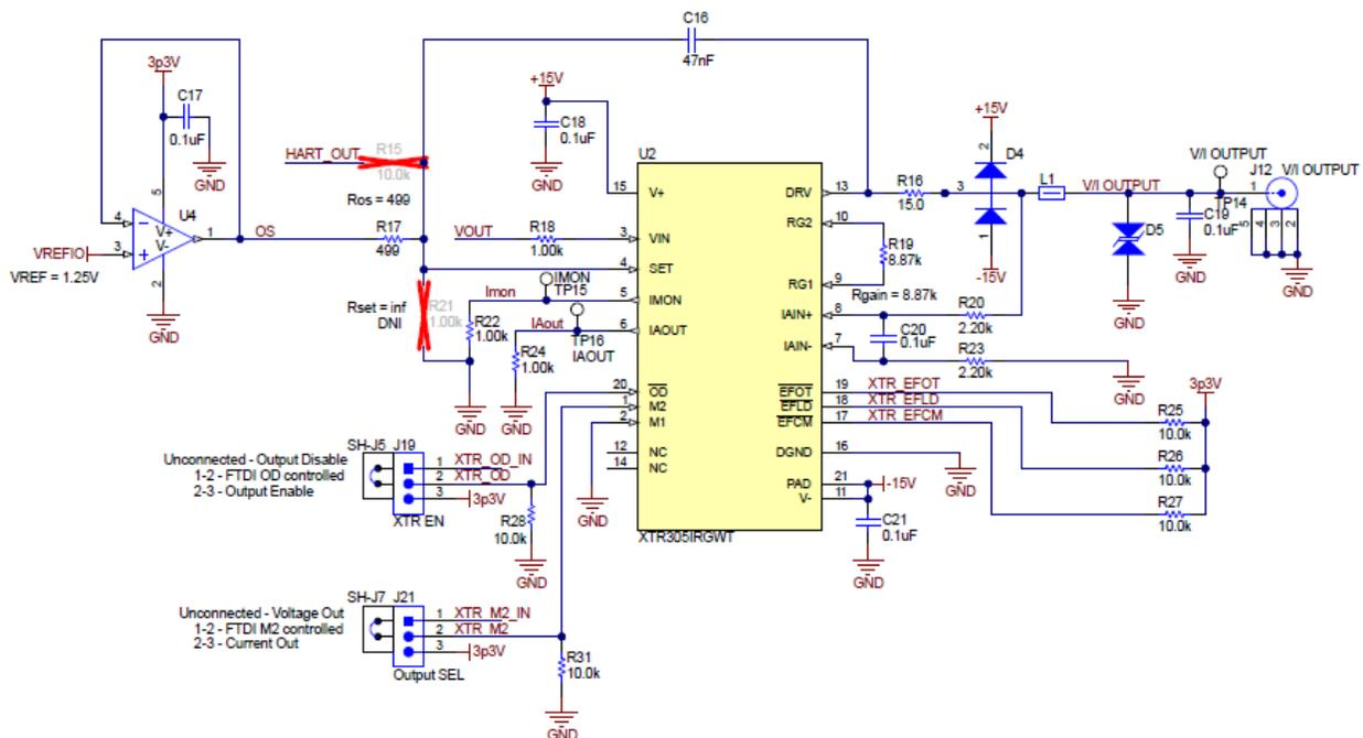
**Figure 3-2. XTR305 Circuit on the AFE882H1EVM**
