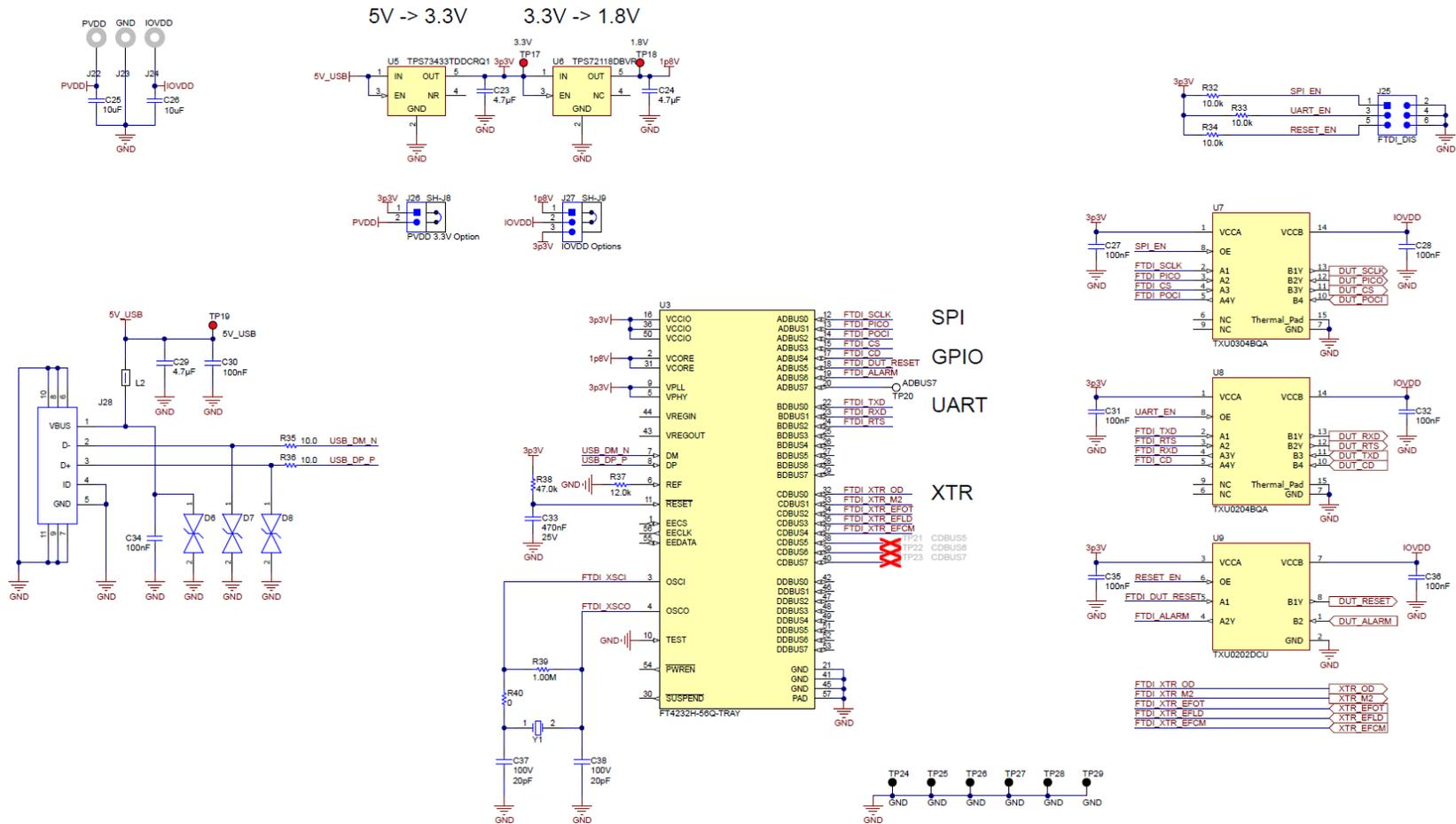
Figure 4-1. AFE882H1EVM Schematic: FTDI Controller
