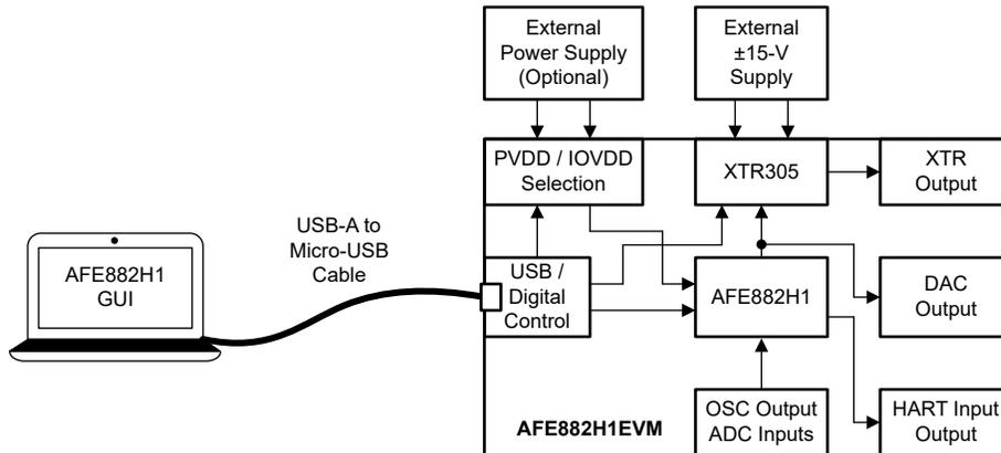
**Figure 2-4. AFE882H1EVM Hardware Setup**
