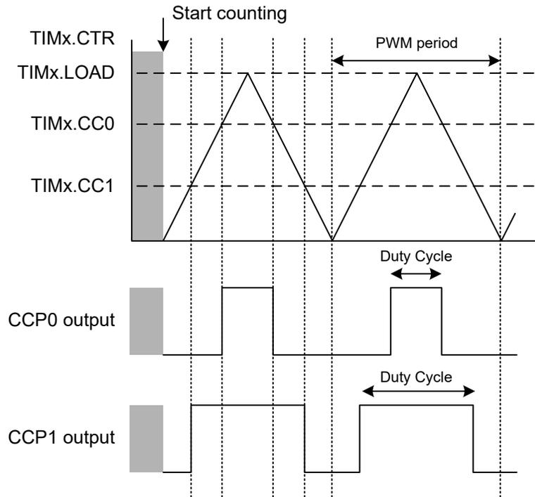
Figure 27-30. Center-Aligned PWM
