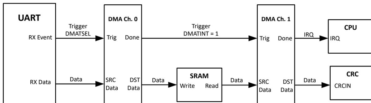
**Figure 5-4. DMA Cascading Channels**
