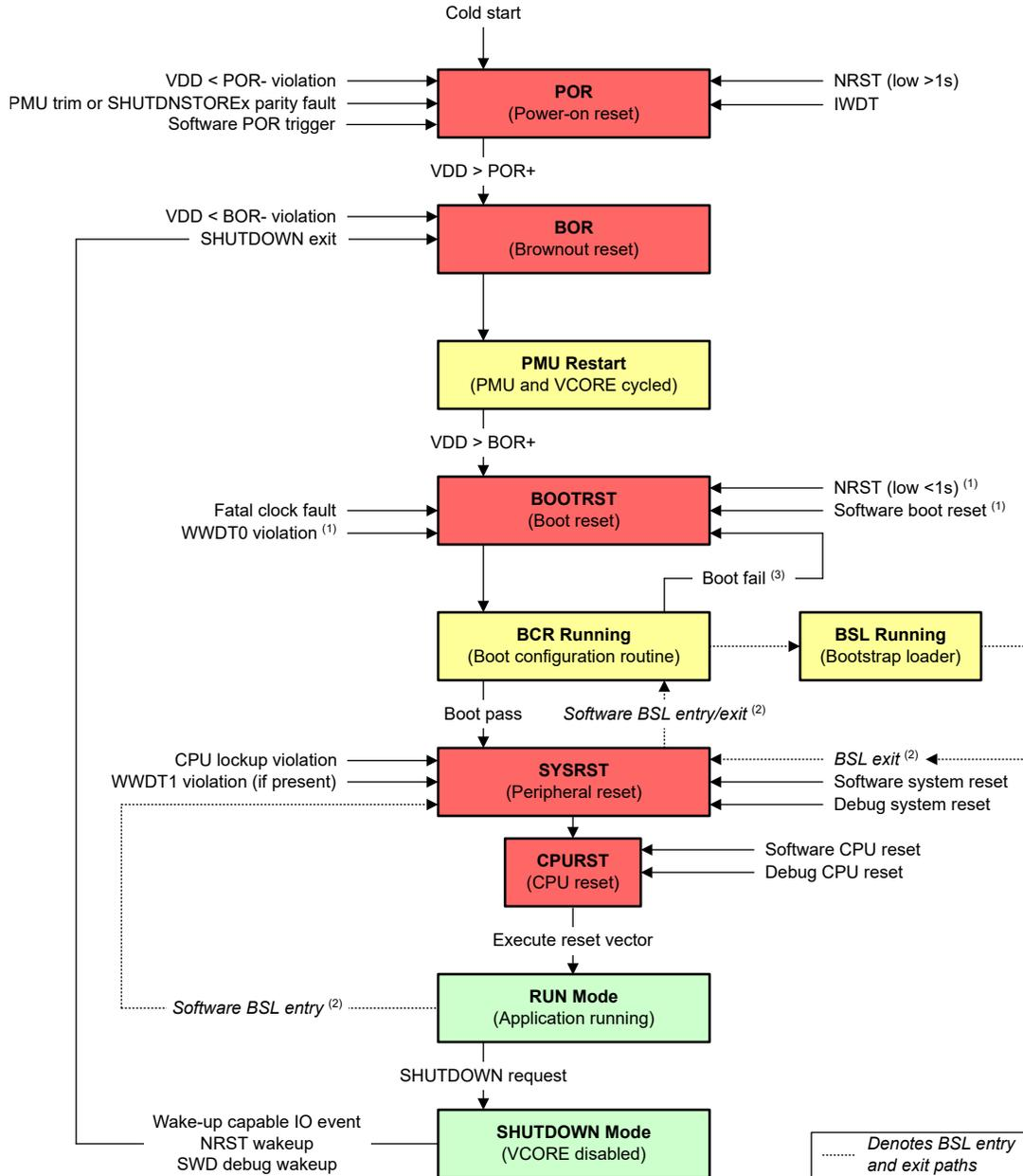
Figure 2-10. Device Reset Levels
