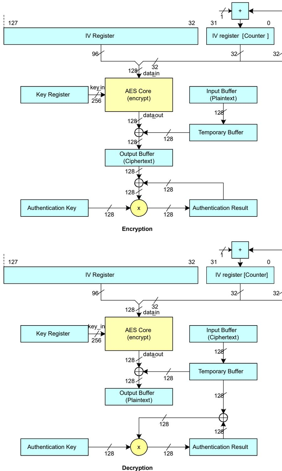
**Figure 12-8. GCM Operation on a Block**
