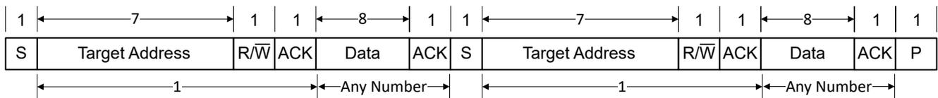
**Figure 24-7. Data Format with Repeated Start**
