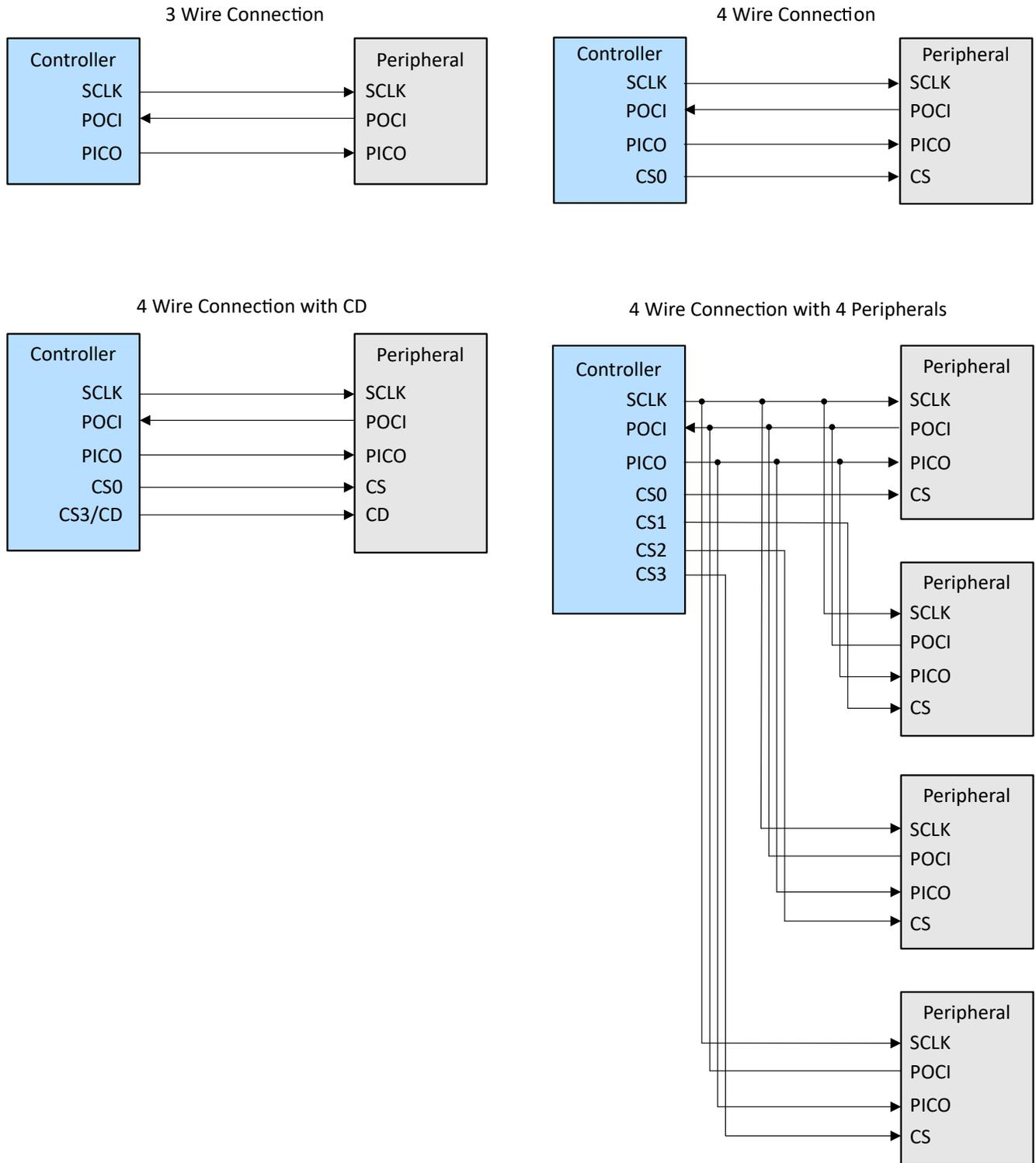
Figure 25-2. External Connections for Different SPI Configurations
