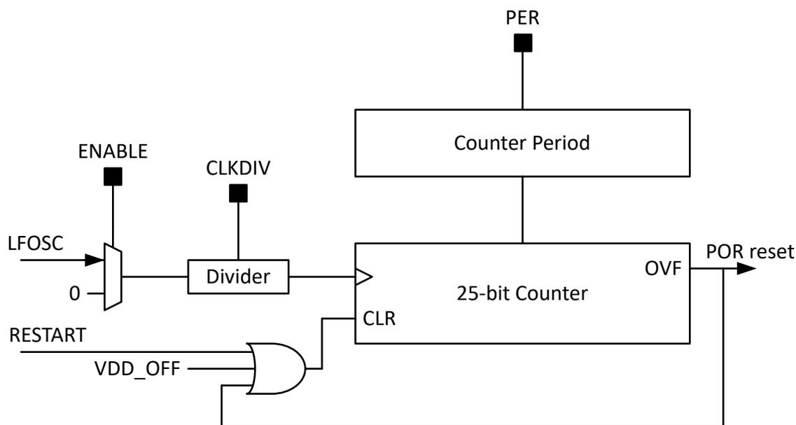
**Figure 30-1. Independent Watchdog Timer (IWDT) Block Diagram**
