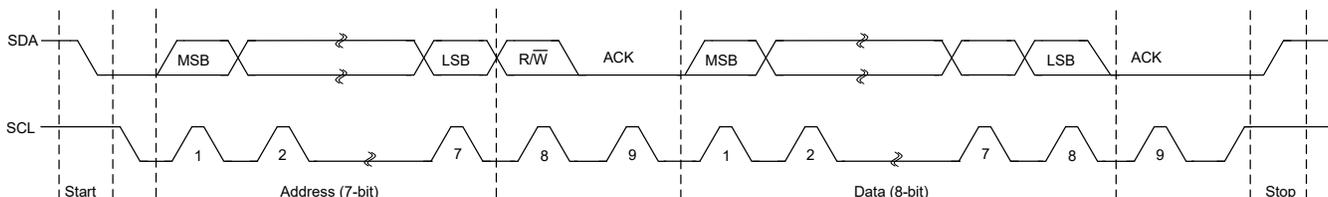
**Figure 24-3. Module Data Transfer**
