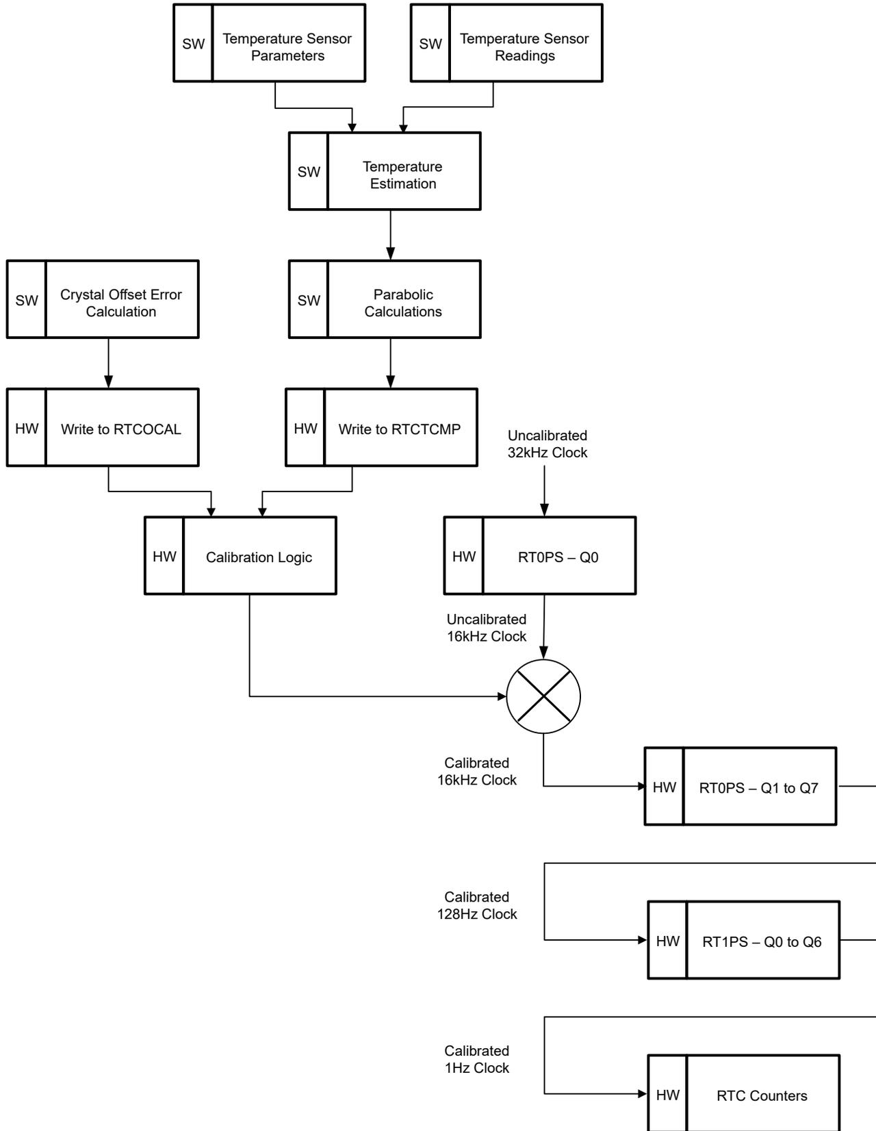
Figure 29-2. RTC Calibration
