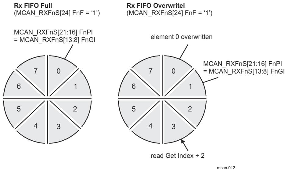
**Figure 26-19. Rx FIFO Overflow Handling**
