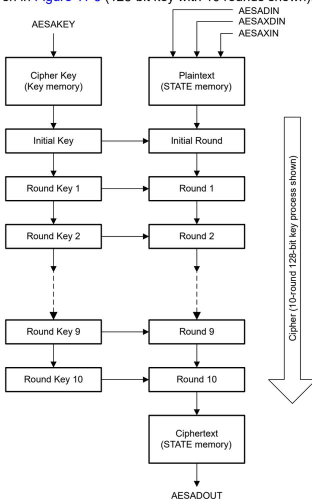
**Figure 11-3. AES Encryption ( $OPx=0x0$ , 128-bit Key)**
