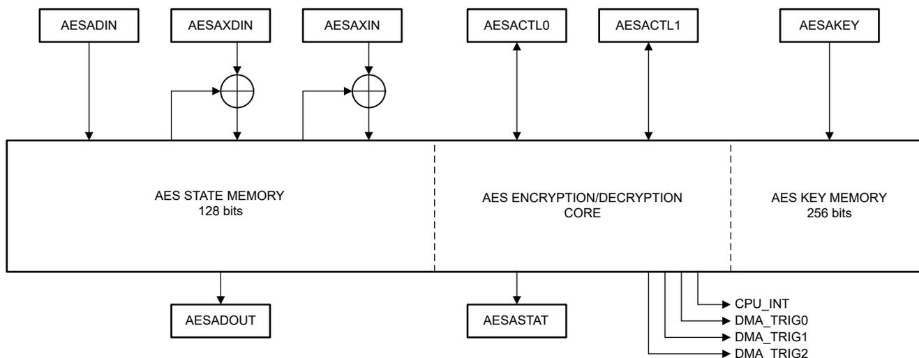
**Figure 11-1. AES Accelerator Block Diagram**
