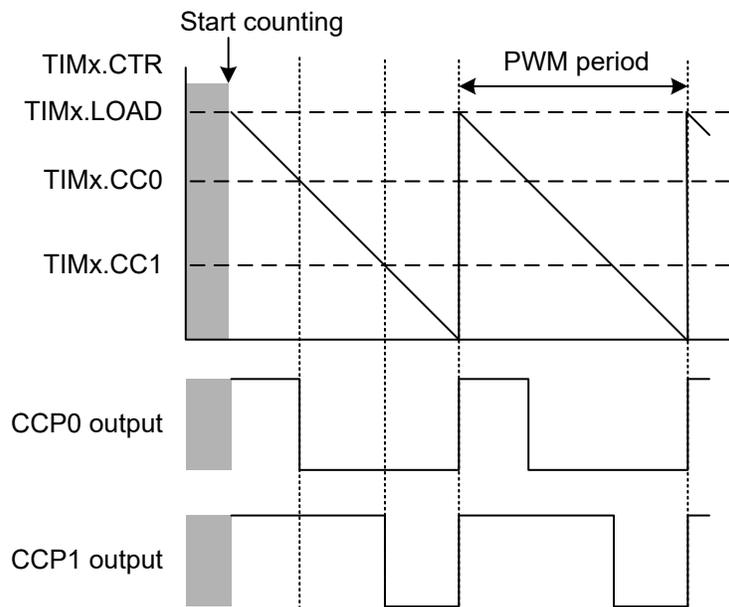
**Figure 27-28. Edge-Aligned PWM Signals in Down-Counting Mode**
