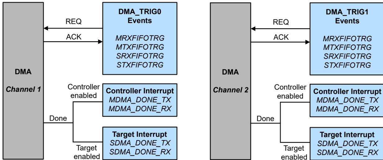
Figure 24-17. I<sup>2</sup>C DMA Trigger and Status
