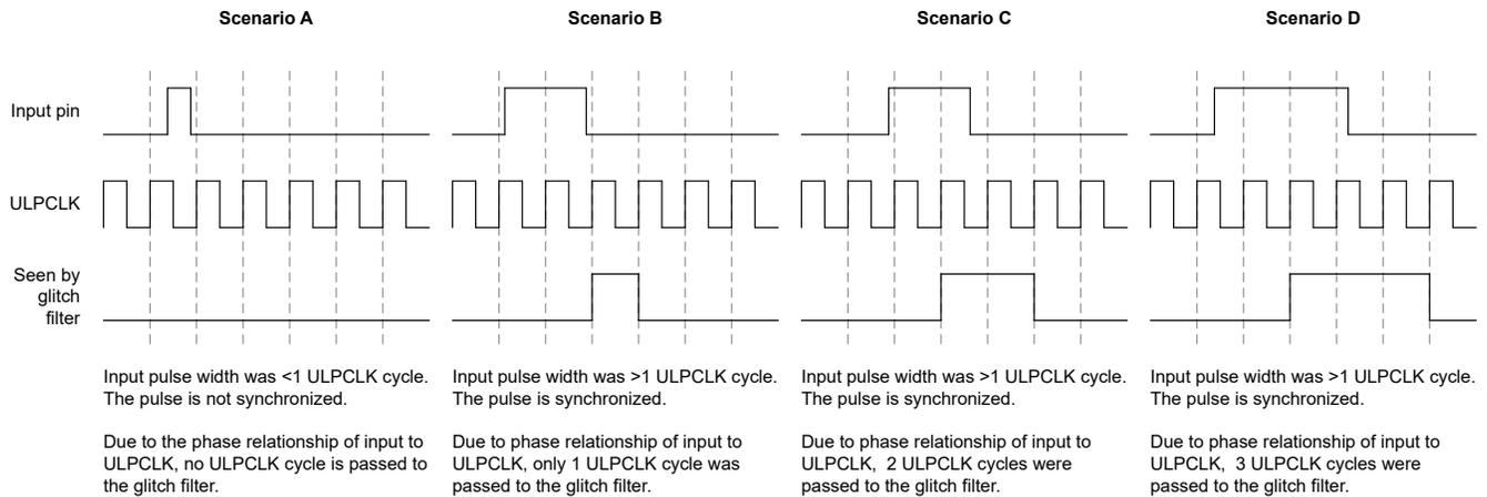
**Figure 9-3. GPIO Input Synchronizer and Glitch Filtering Scenarios**
