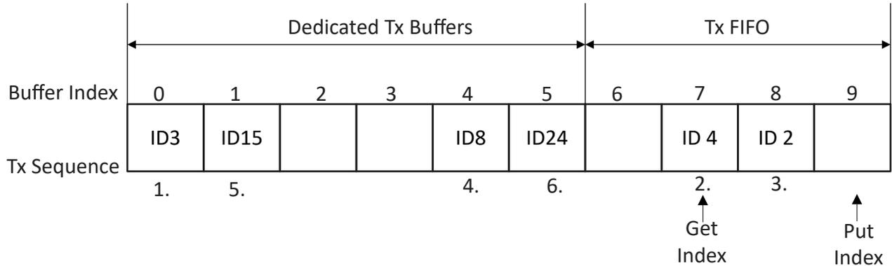
**Figure 26-14. Mixed Dedicated Tx Buffers/ Tx FIFO (example)**
