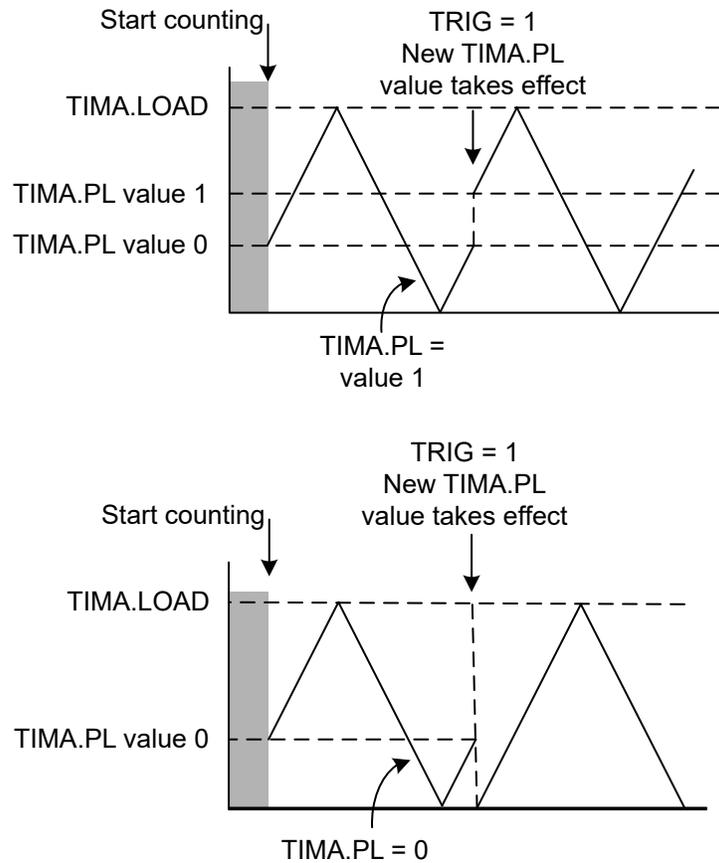
**Figure 27-11. Phase Load Register Synchronization in Up-Down Mode**
