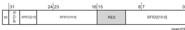
**Figure 26-24. Standard Message ID Filter Element Structure**
