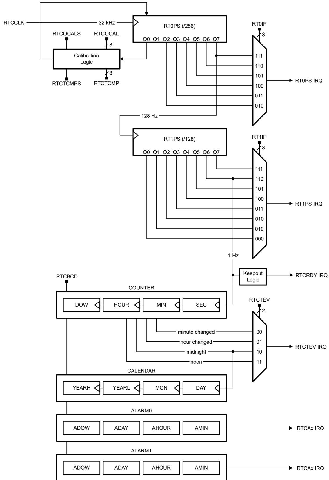
Figure 29-1. RTC Block Diagram
