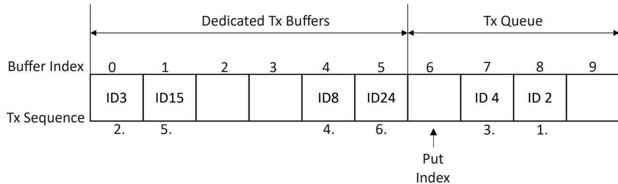
**Figure 26-15. Mixed Dedicated Tx Buffers/ Tx FIFO (Example)**
