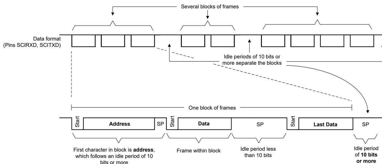
**Figure 23-10. Idle-Line Multiprocessor**
