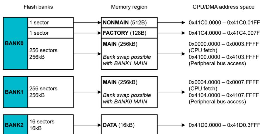
**Figure 6-3. Memory Organization Example - Multiple Bank Configuration**
