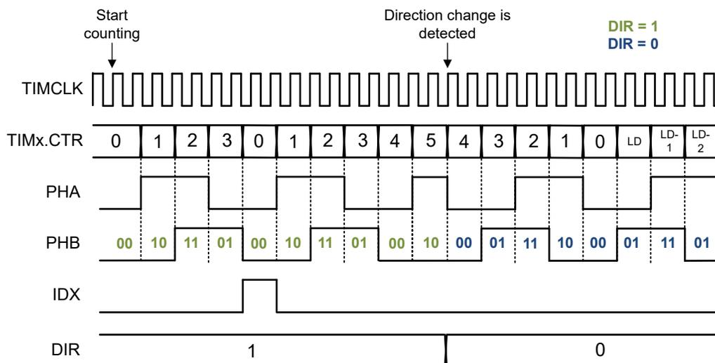
Figure 27-20. 2-Signal QEI with Index Input Operation
