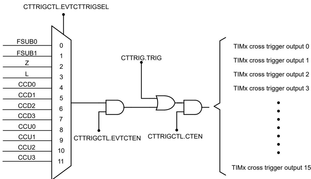
**Figure 27-39. Main Timer Cross Trigger Output Configuration**
