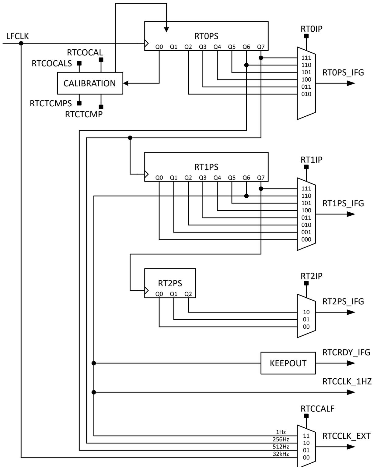
Figure 29-3. RTC Prescaler and Interval Timer Event
