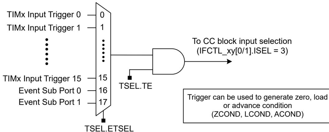
**Figure 27-40. Secondary Timer Cross Trigger Input Configuration**
