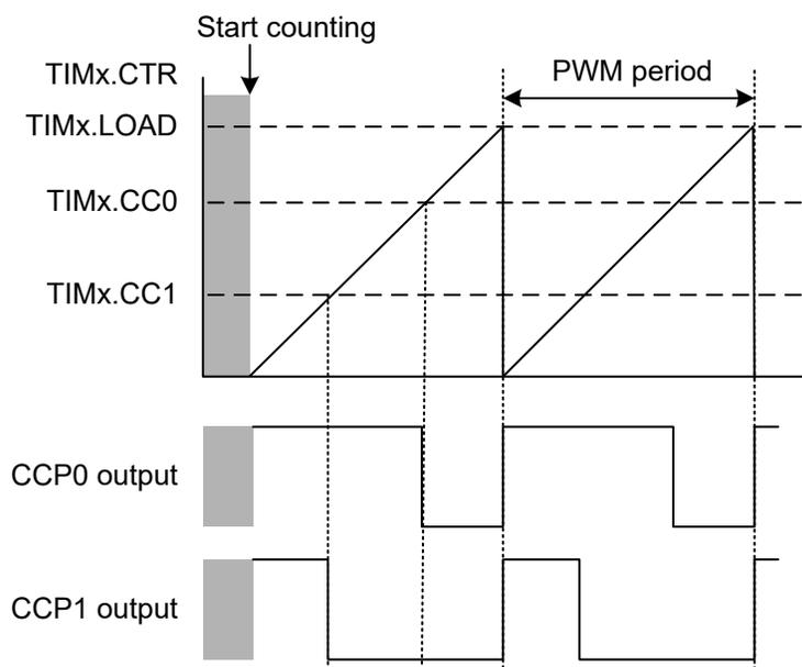
**Figure 27-29. Edge-Aligned PWM Signals in Up-Counting Mode**
