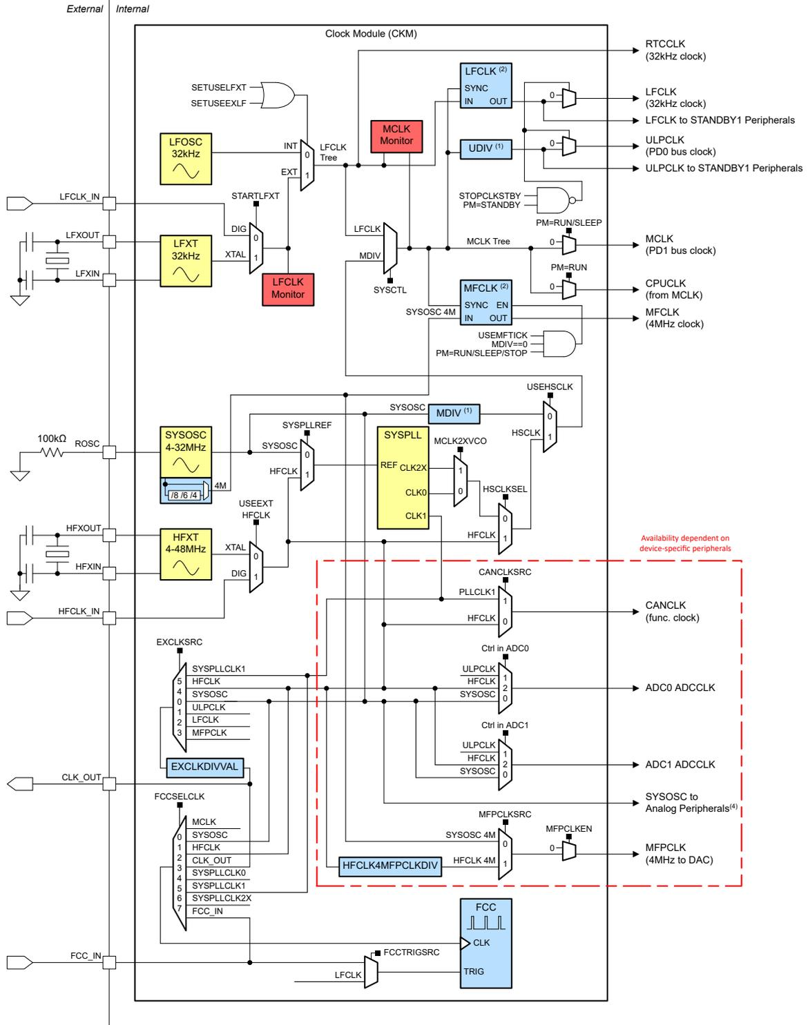
Figure 2-8. MSPM0Gxx Top Level Clocking Tree
