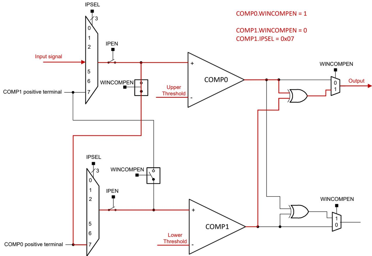
**Figure 18-5. Window Comparator Mode Configuration**
