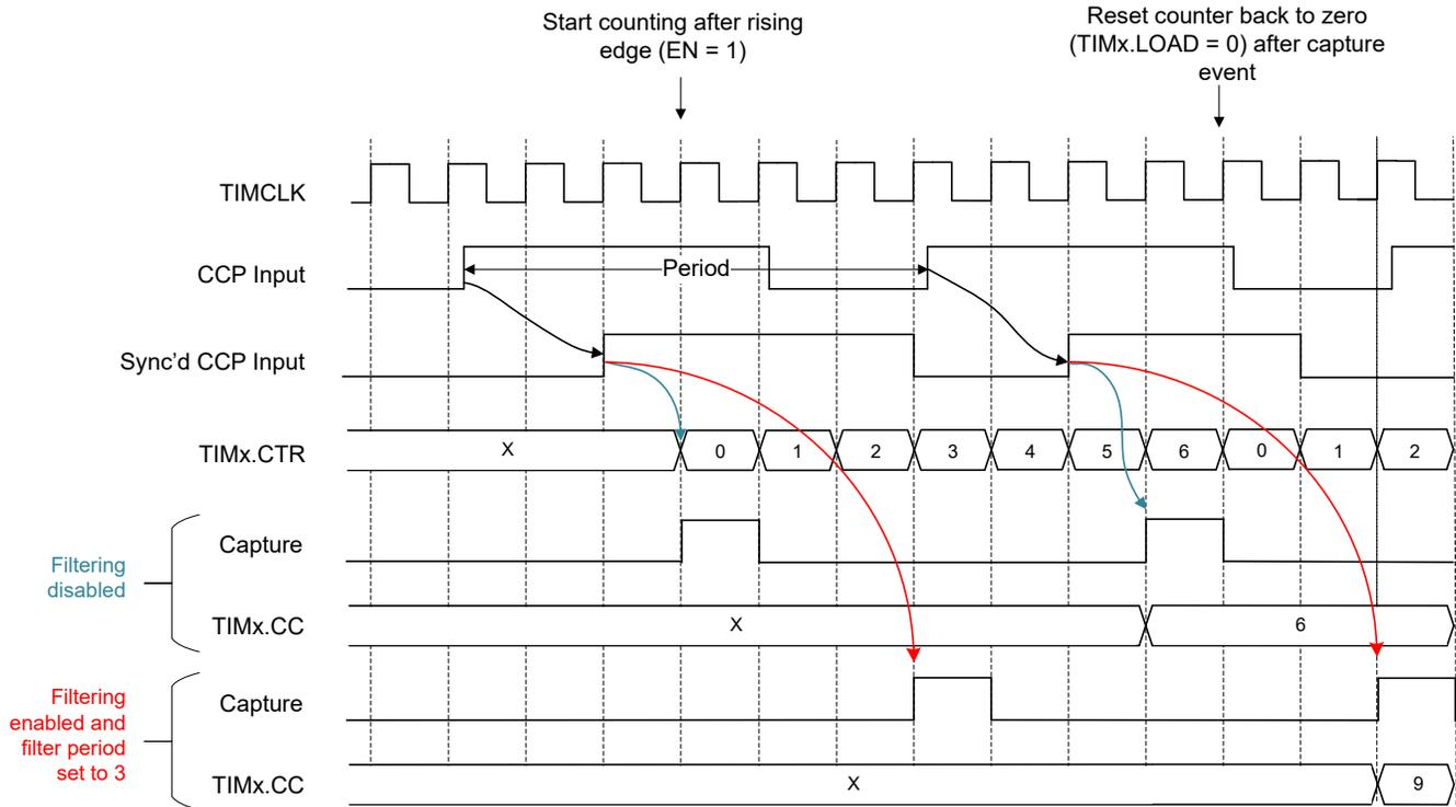
**Figure 27-15. Period Capture Mode in Up-Counting Mode, CVAE = 2**
