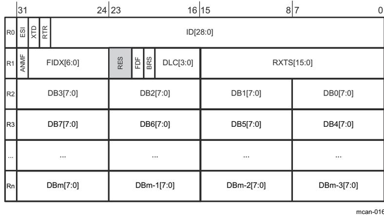
Figure 26-21. Rx Buffer/Rx FIFO Element Structure
