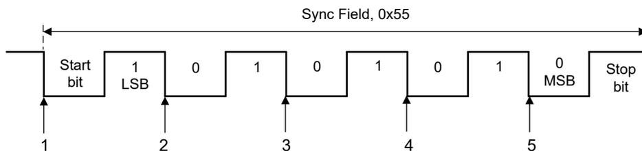
**Figure 23-7. LIN SYNC Field Detection**
