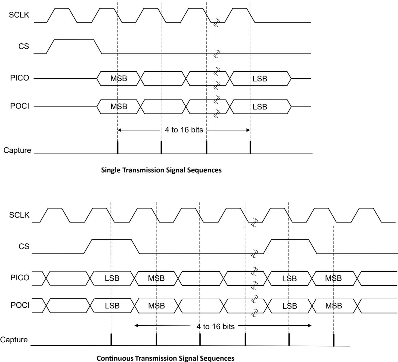
**Figure 25-8. TI Synchronous Serial Frame Format**
