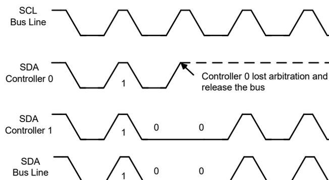
**Figure 24-8. Arbitration Procedure Between Two Controller Transmitters**
