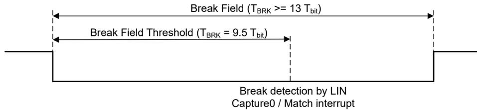
**Figure 23-6. LIN Break Field Detection**
