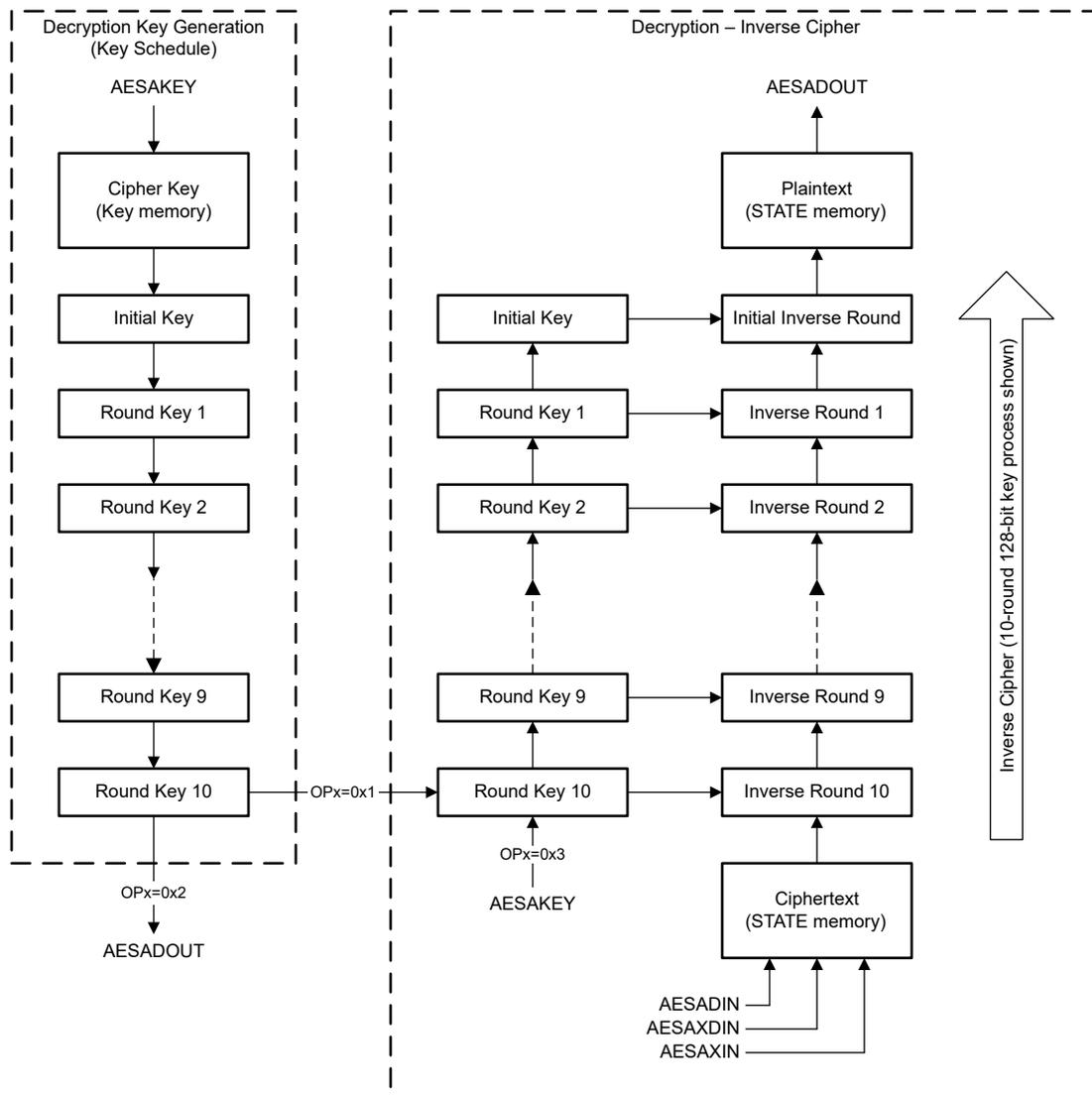
**Figure 11-4. AES Decryption (OPx = 0x1, 128-bit Key)**
