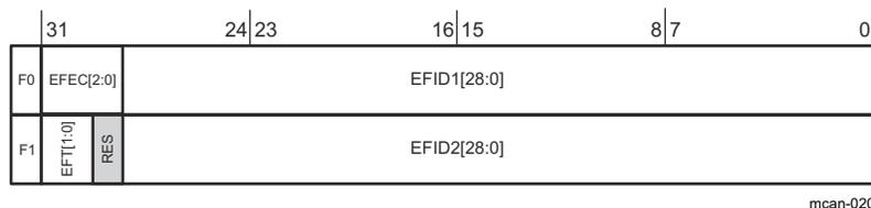
**Figure 26-25. Extended Message ID Filter Element Structure**
