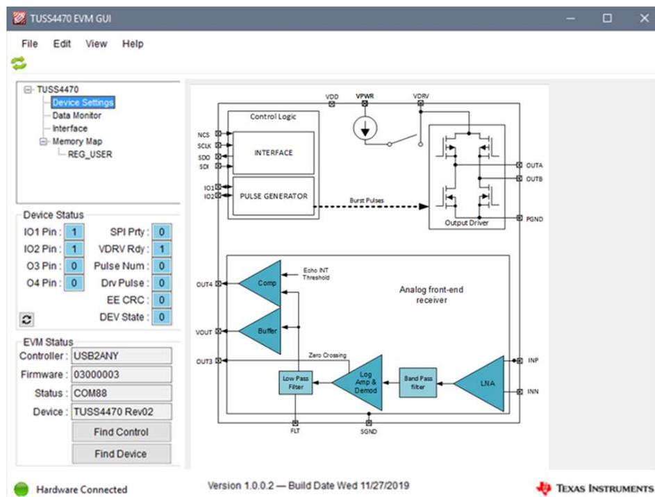
Figure 8. TUSS44x0 EVM GUI Starting Screen With Successful EVM Connection Status
