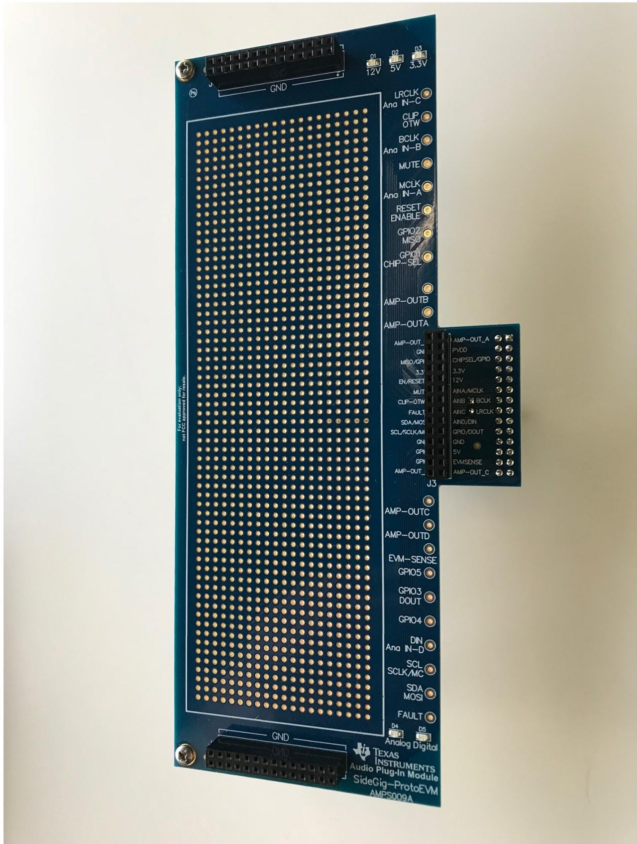
Figure 1. Prototype Plug-In Module
