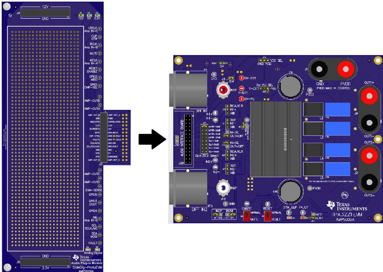
Figure 3. Connecting Prototype Plug-in Module to EVM
