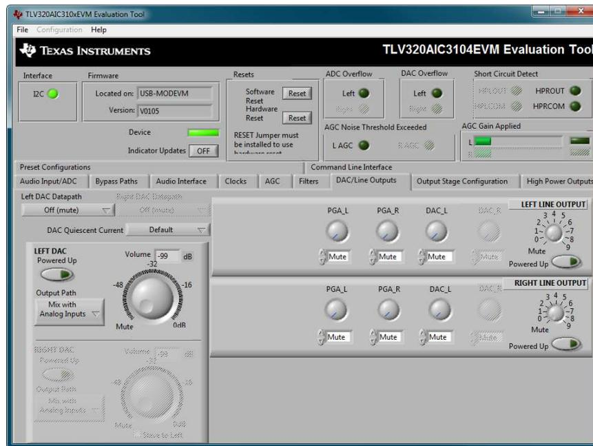
Figure 26. DAC/Line Outputs Tab
