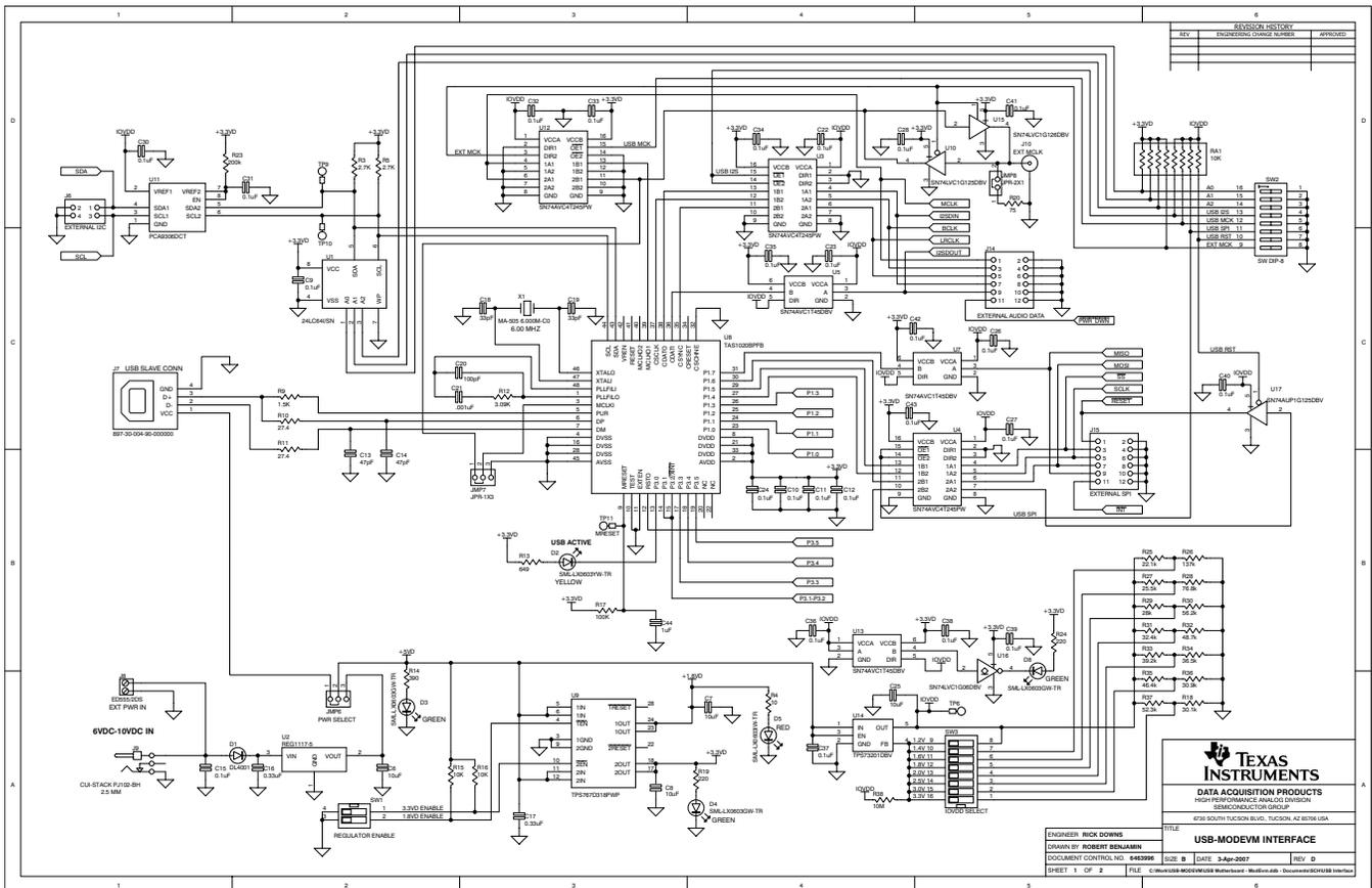
**Figure 39. USB-MODEVM Interface Board Schematic (1 of 2)**
