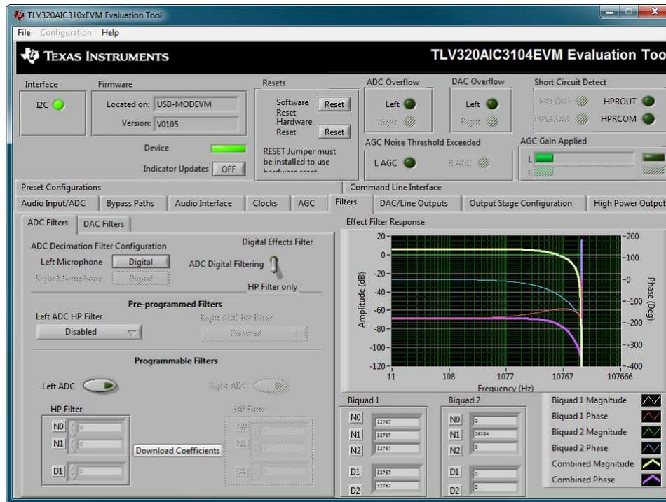
**Figure 15. Filters Tab**
