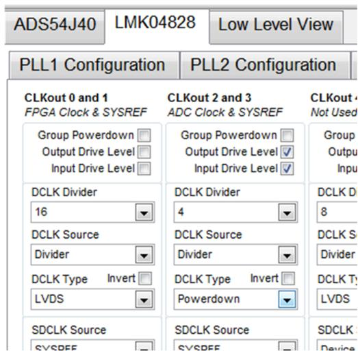
Figure 9. LMK04828 Clock Outputs Tab
