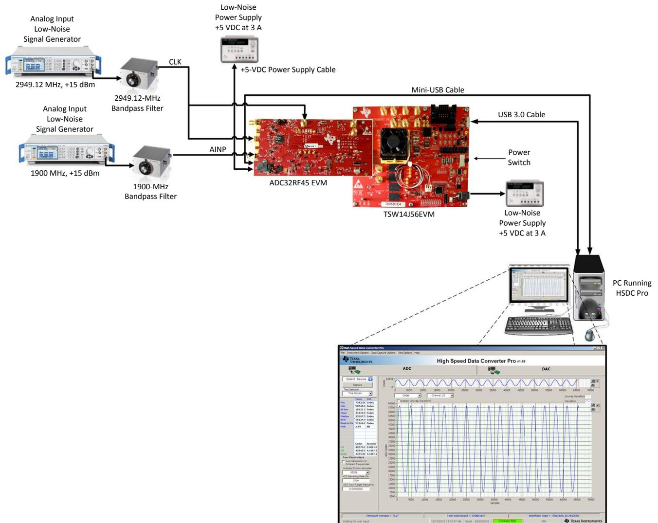
Figure 2. ADC32RFxx-EVM GUI Bench Setup Block Diagram
