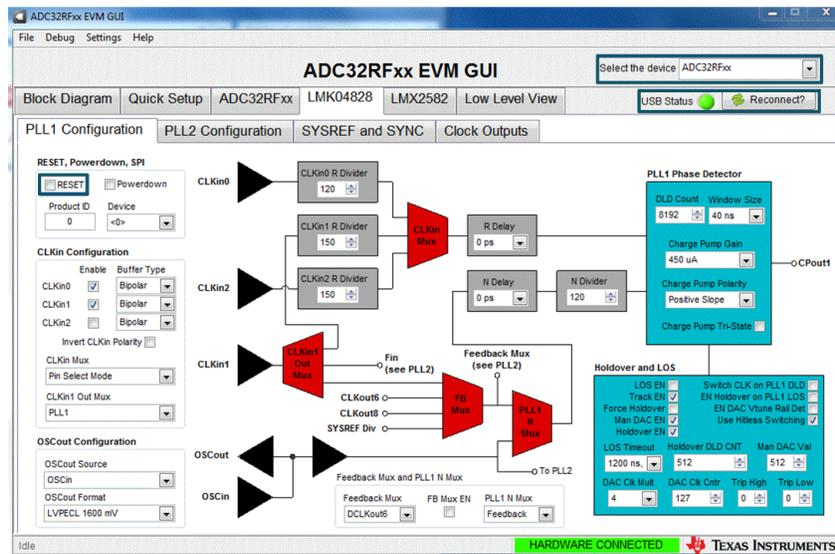
Figure 18. ADC32RFxx-EVM GUI LMK04828 PLL1 Page DDC Mode
