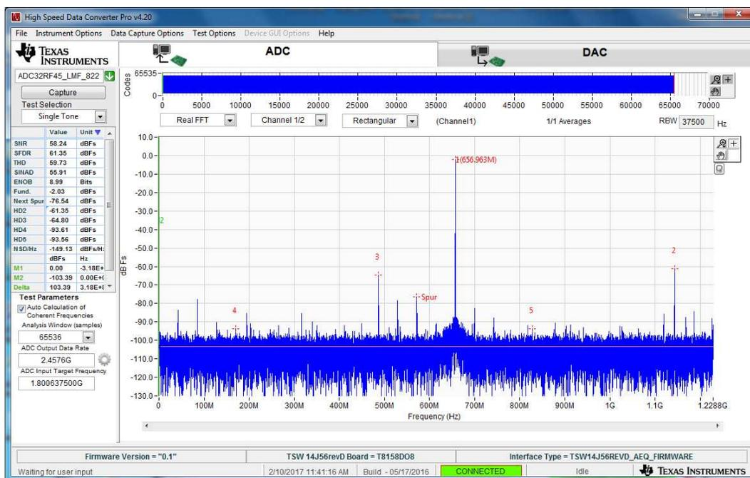
Figure 30. Example Capture from Channel A – LMFS8224 Mode
