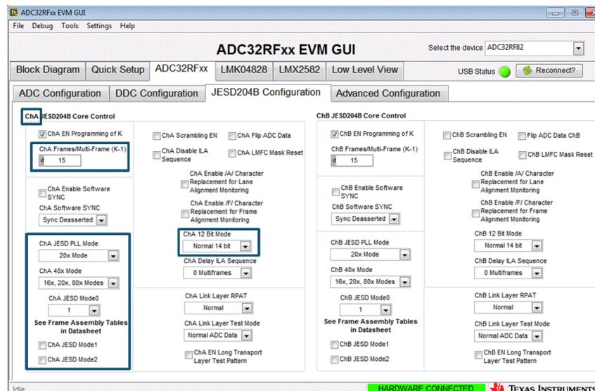
Figure 10. ADC32RFxx-EVM GUI JESD204B Configuration Tab DDC Mode
