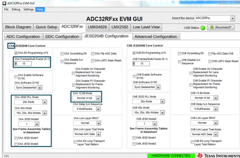
Figure 20. ADC32RFxx-EVM GUI JESD204B Configuration Tab DDC Mode
