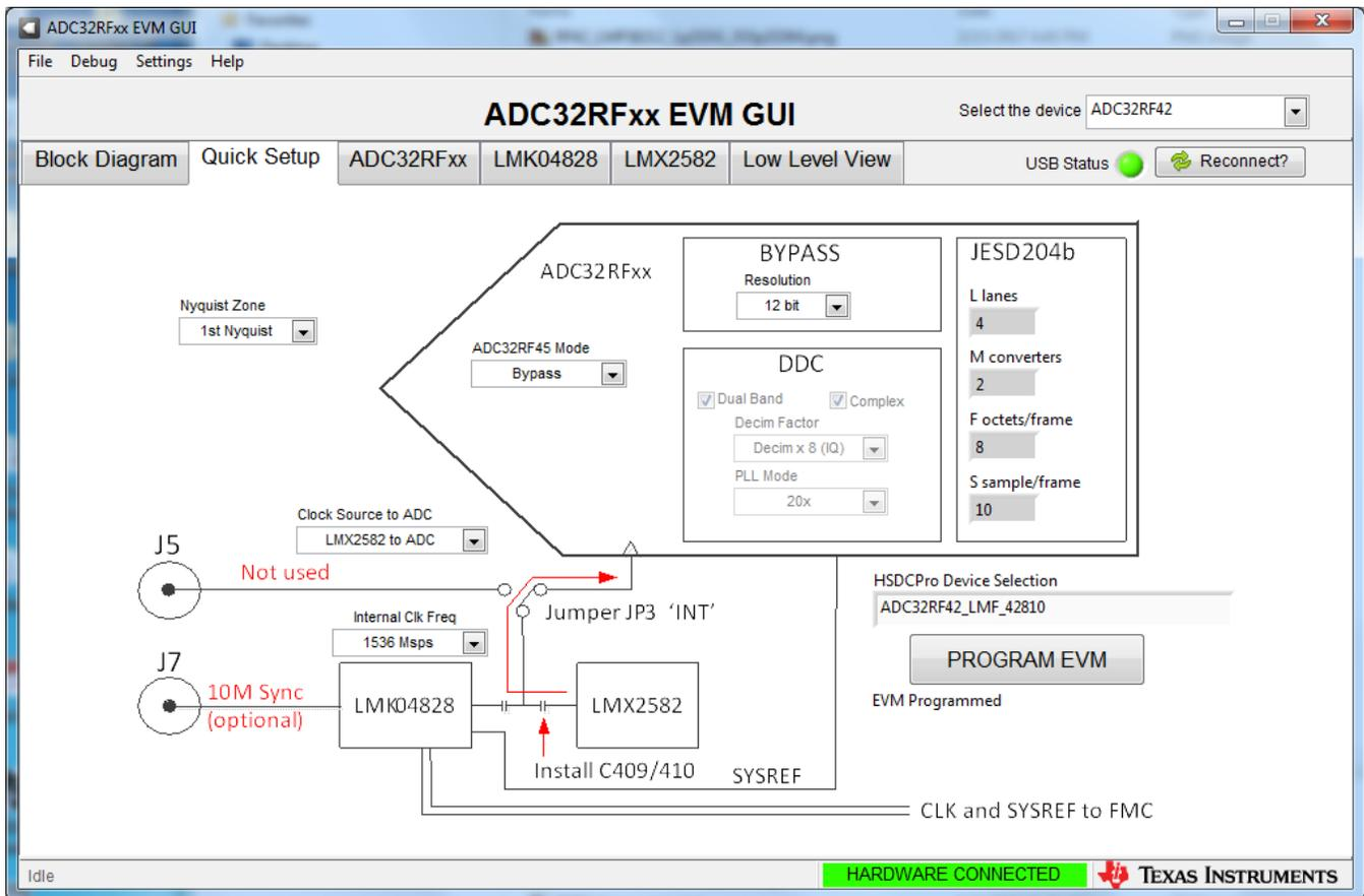
**Figure 31. ADC32RF42-EVM Quick Setup View Bypass Mode**
