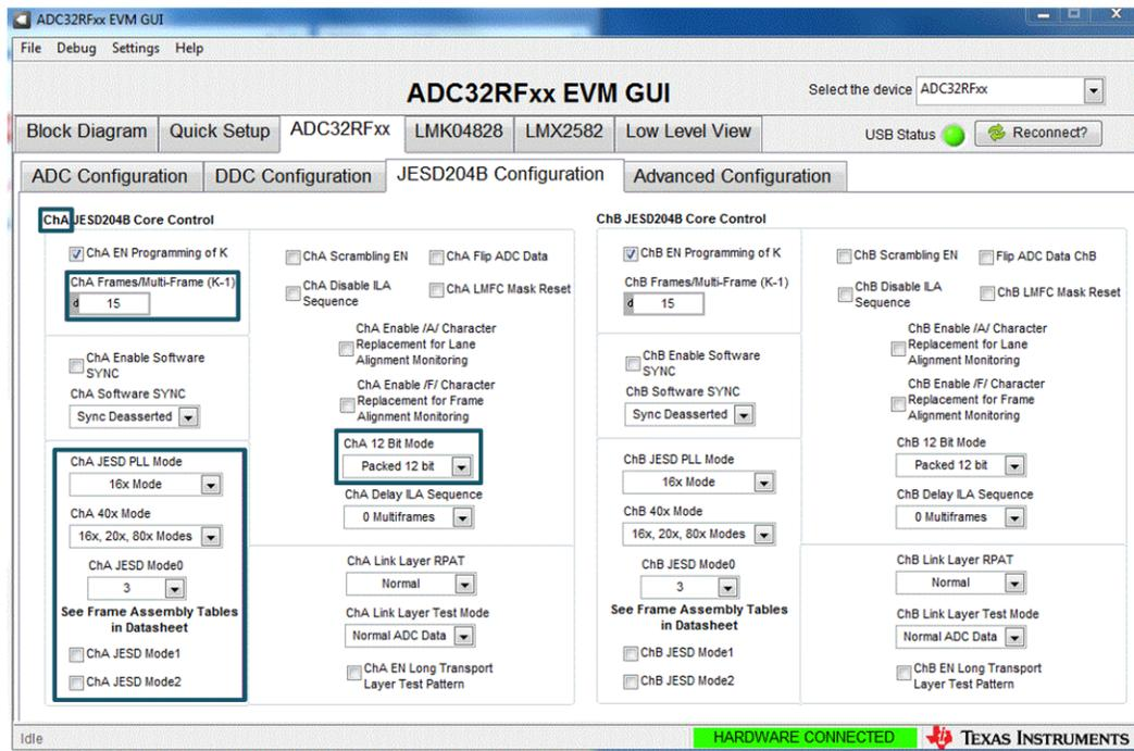
**Figure 5. ADC32RFxx-EVM GUI JESD204B Tab Bypass Mode**
