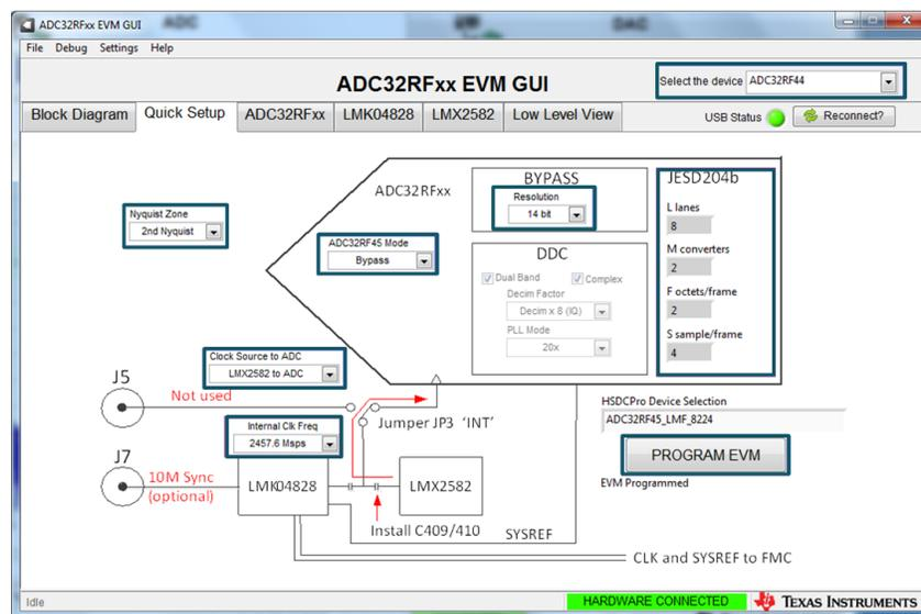
**Figure 28. ADC32RF44-EVM Quick Setup View Bypass Mode**
