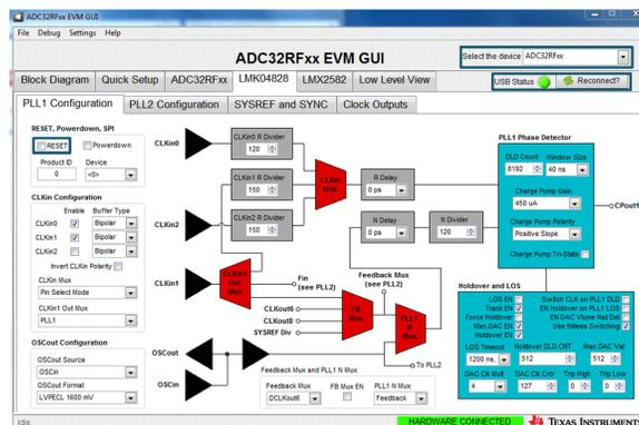
Figure 3. ADC32RFxx-EVM GUI LMK04828 PLL1 Page Bypass Mode
