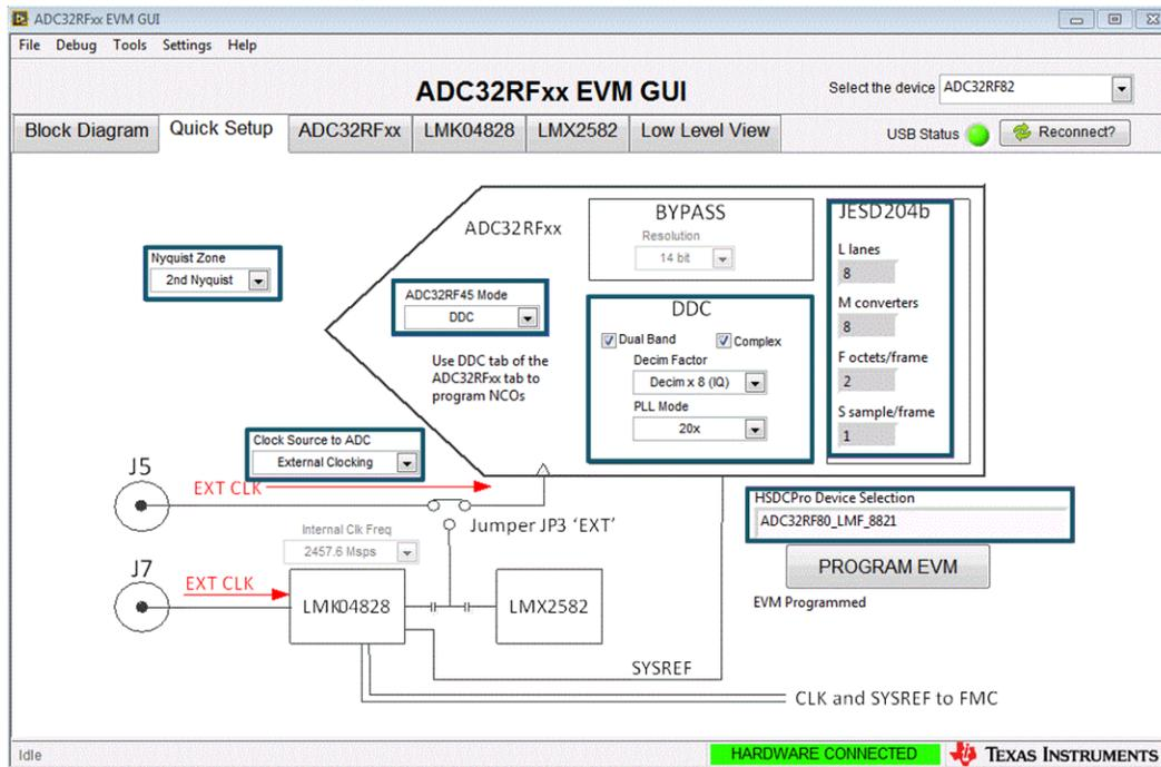
Figure 9. ADC32RFxx-EVM Quick Setup View DDC Mode
