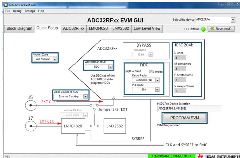
Figure 19. ADC32RFxx-EVM Quick Setup View DDC Mode
