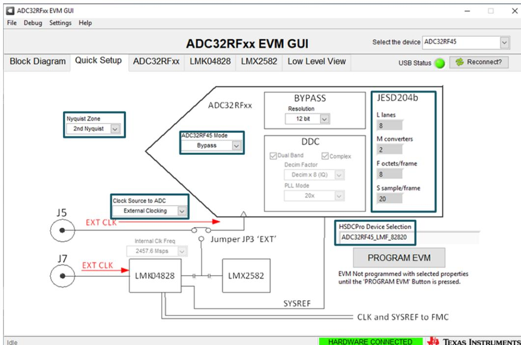
**Figure 4. ADC32RFxx-EVM Quick Setup View Bypass Mode**
