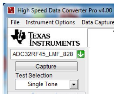
**Figure 6. HSDC Pro Device Selection LMFS\_82820 Mode**
