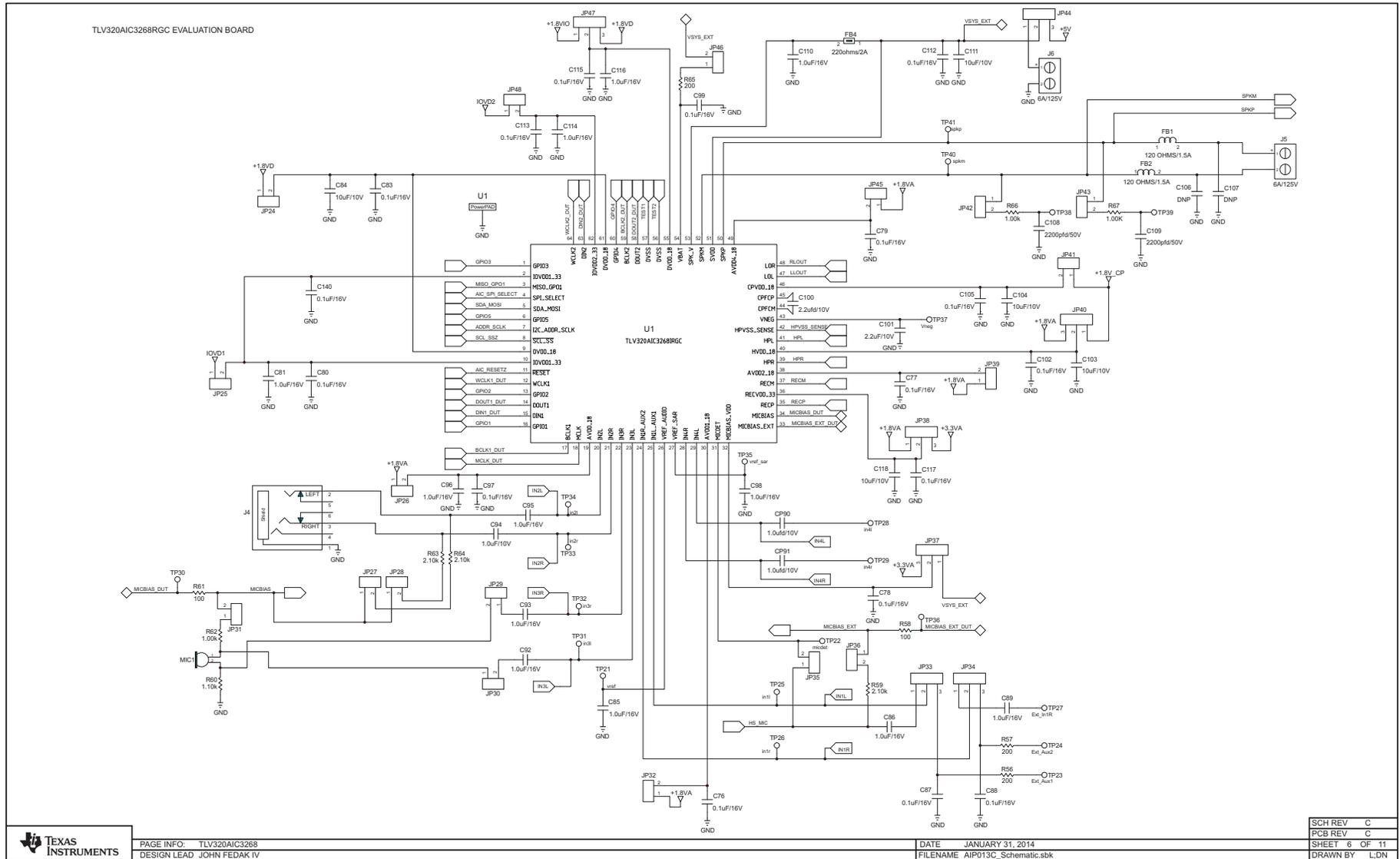
Figure 10. TLV320AIC3268 Schematic
