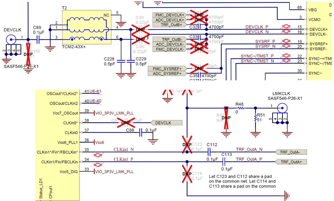
Figure B-1. Configuration for Optional Clcking Support
