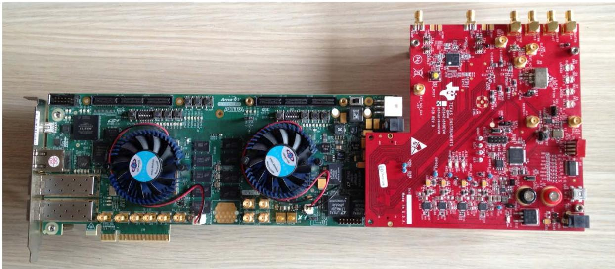
Figure 1 ADS42JB49 Hardware test bed Components
