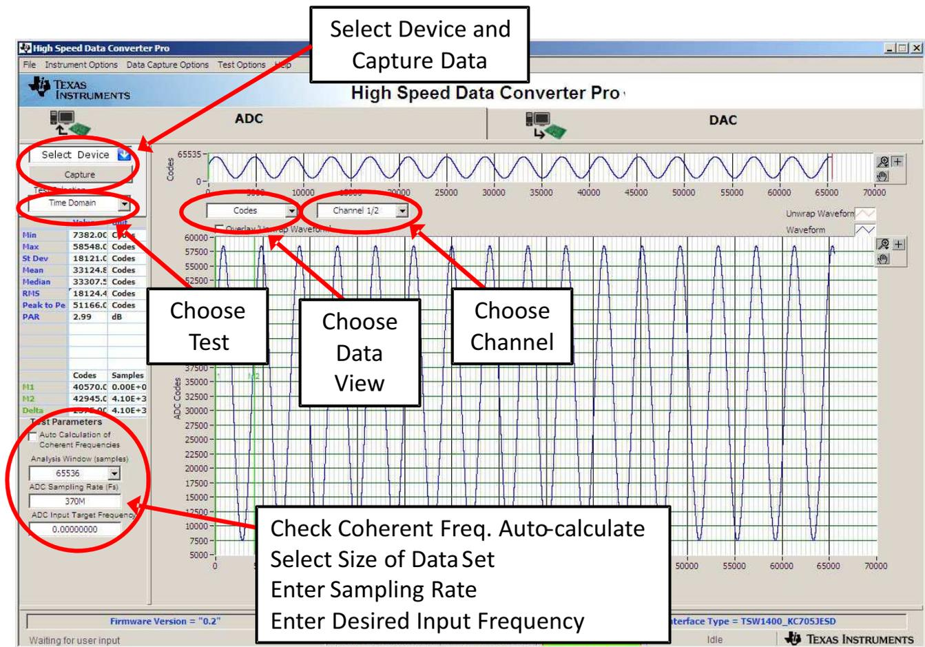
Figure 3. High Speed Data Converter Pro (HSDP) GUI
