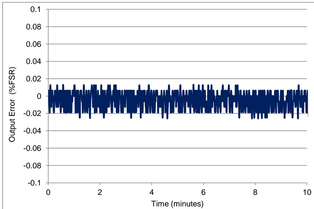
**Figure 17: Module Output Error during ESD Tests**
