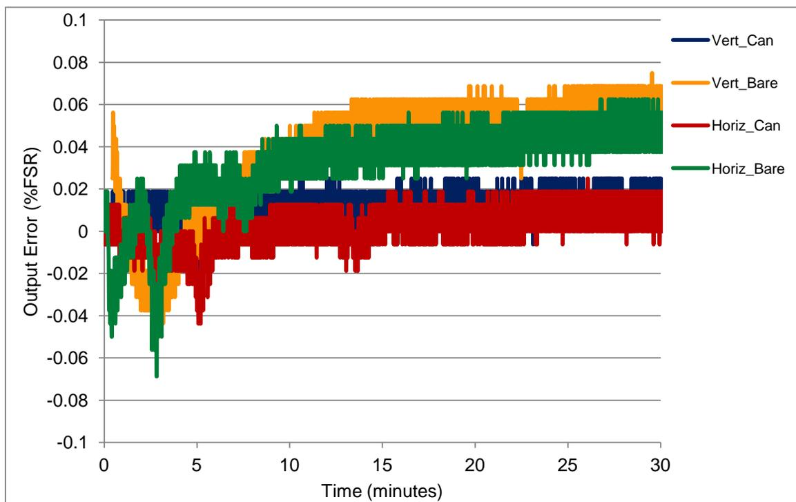
**Figure 18: Radiated Immunity Test – 3 V/m**
