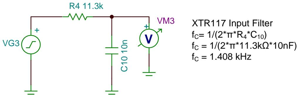
Figure 8: XTR117 Input Filter – Schematic
