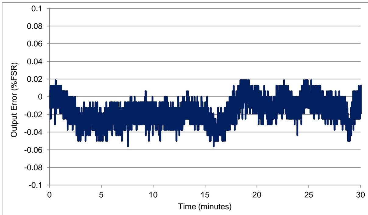
**Figure 22: Module Output Error during Conducted EMI Immunity Tests**
