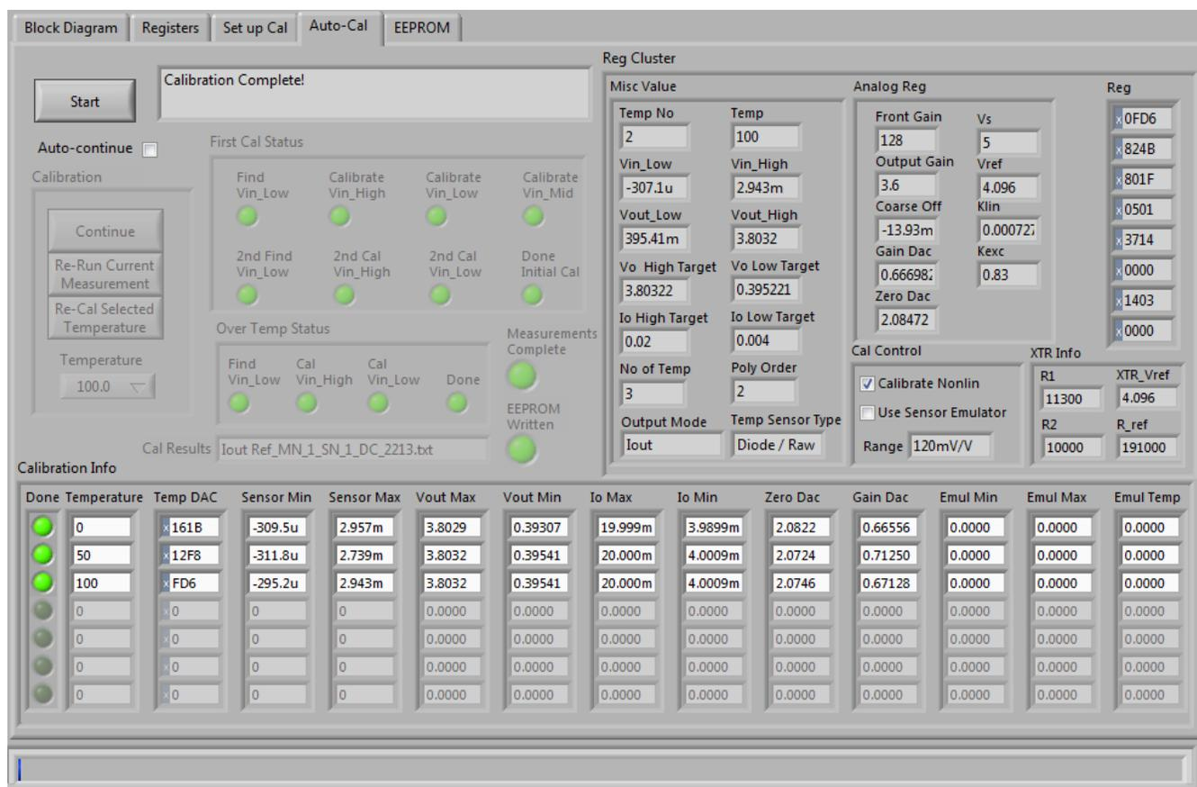
Figure 12: PGA309EVM-USB Software (Post-Calibration)
