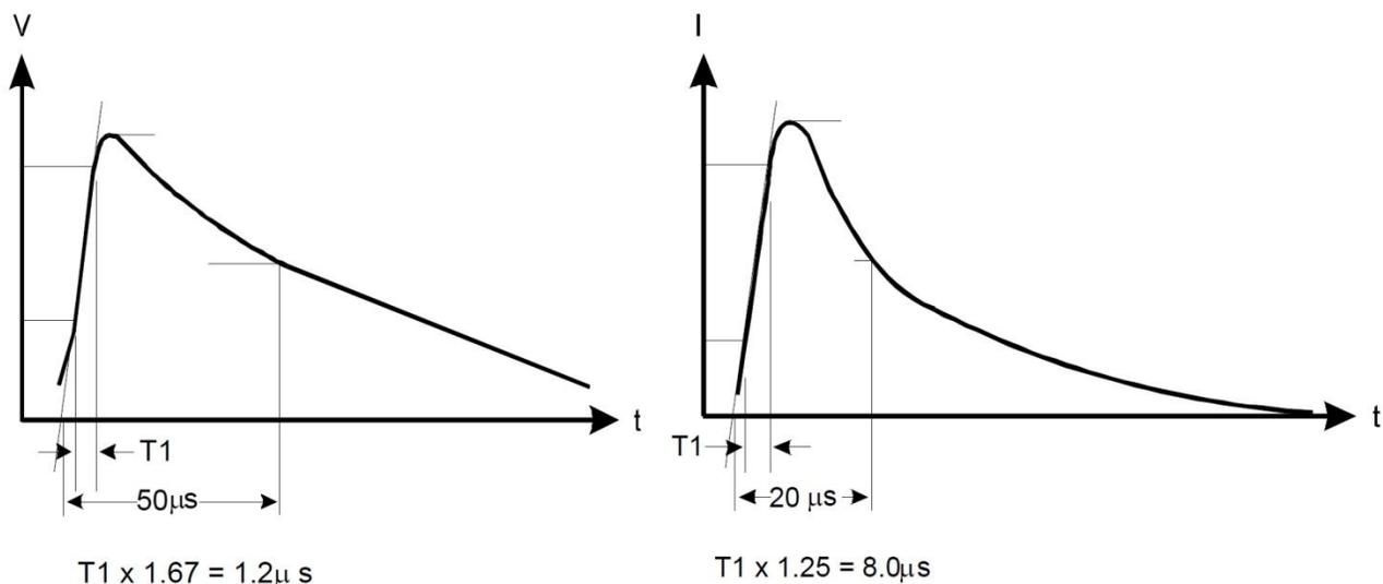
**Figure B-9: IEC 61000-4-5 Surge Waveforms [7]**
