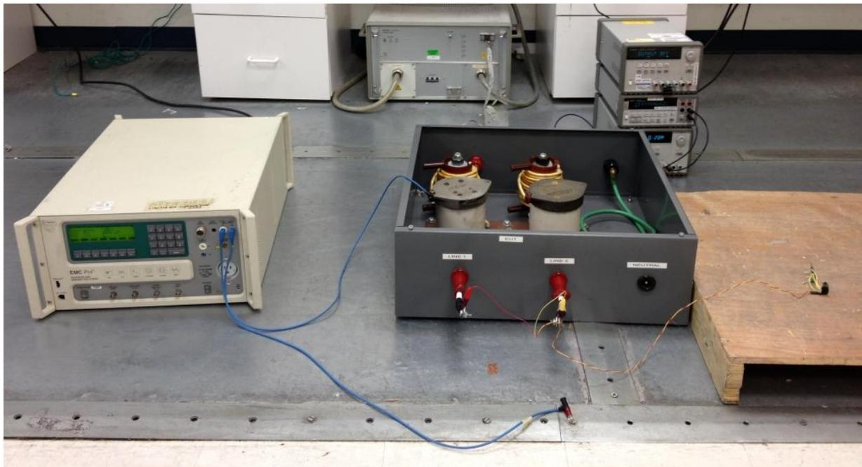
**Figure B-10: IEC 61000-4-5 Surge Test Hardware Setup**
