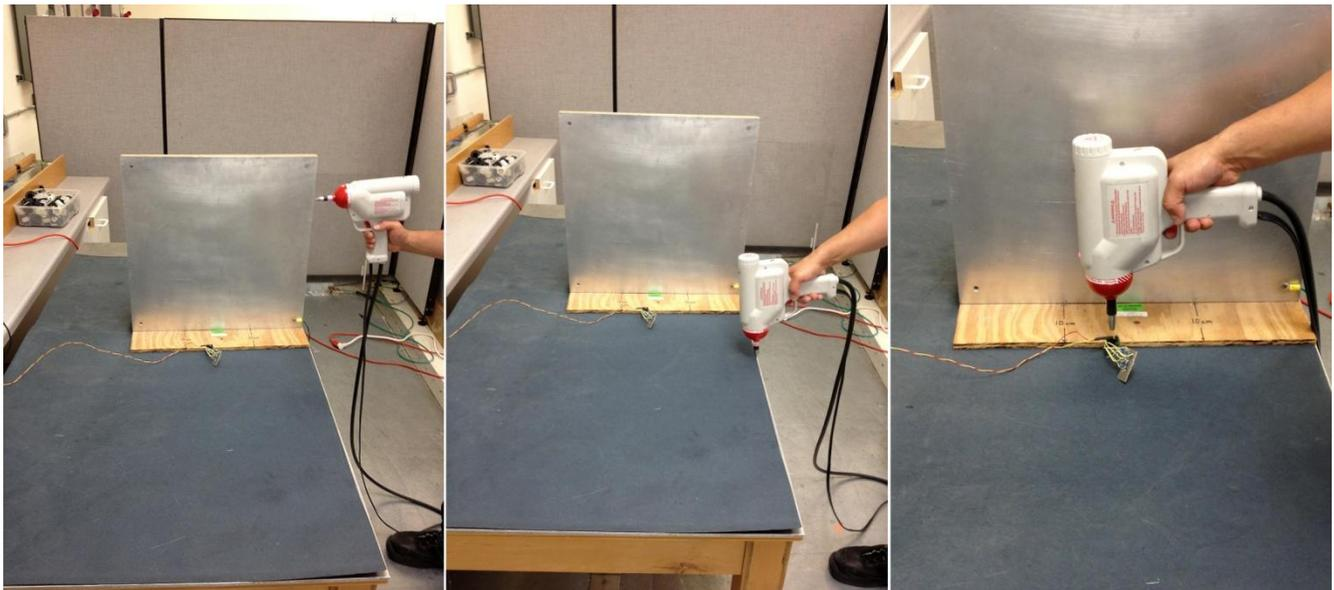
**Figure B-3: IEC 61000-4-2 ESD Tests – VCP, HCP, Air Discharge**
