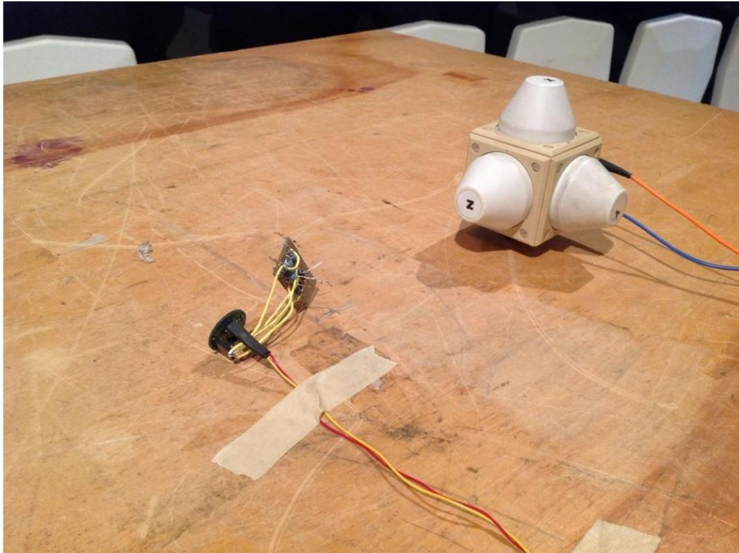
**Figure B-5: Device under Test (with Sensor Test Board) and Field Sensor**
