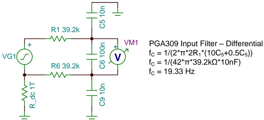
Figure 4: PGA309 Input Filter (Differential) – Schematic
