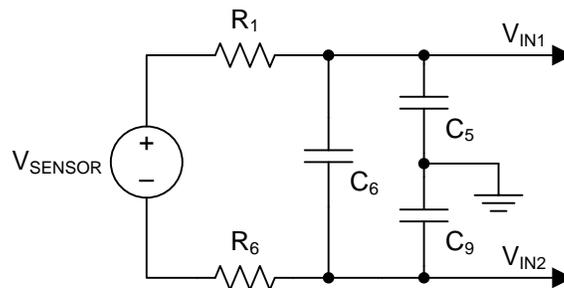
**Figure 3: Sensor Voltage Input Filter**
