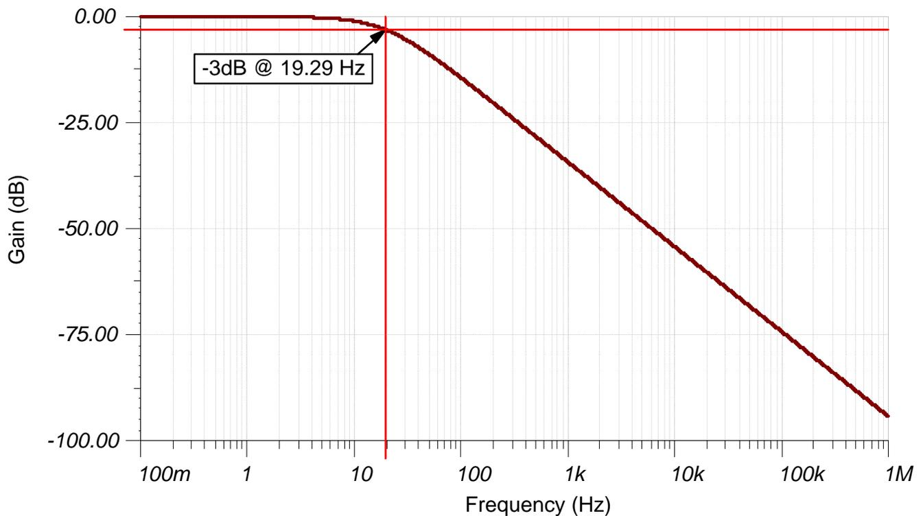
Figure 5: PGA309 Input Filter (Differential) – Transfer Characteristic
