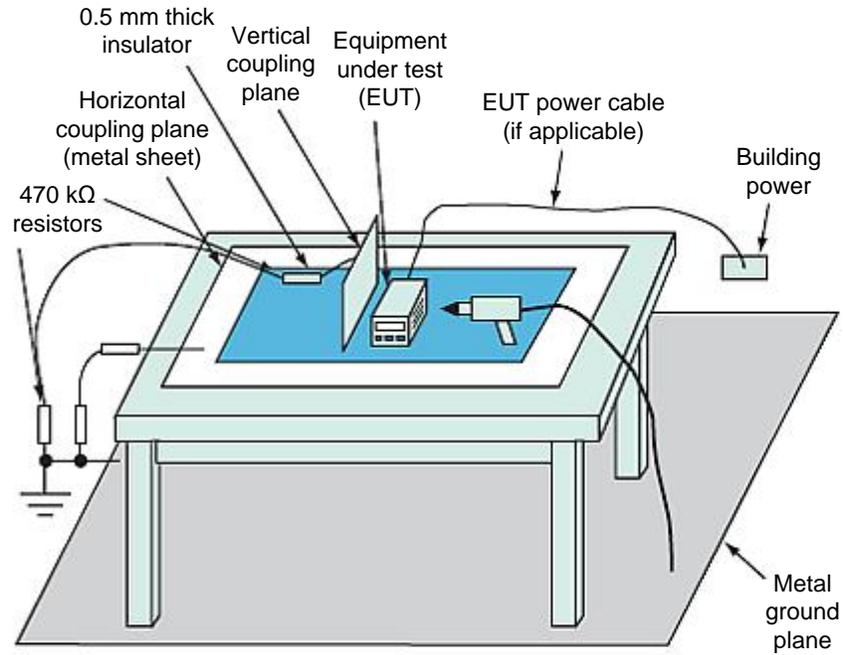
**Figure B-2: IEC 61000-4-2 ESD Test Hardware Setup [2]**
