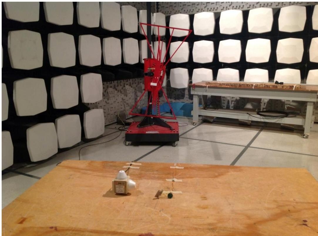
**Figure B-6: IEC 61000-4-3 Full Test Chamber Setup**
