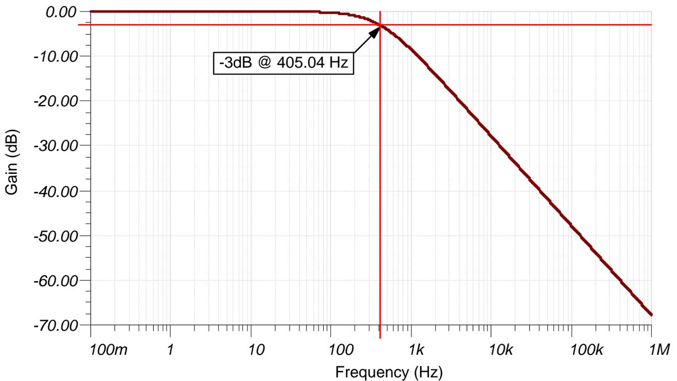
Figure 7: PGA309 Input Filter (Common-Mode) – Transfer Characteristic
