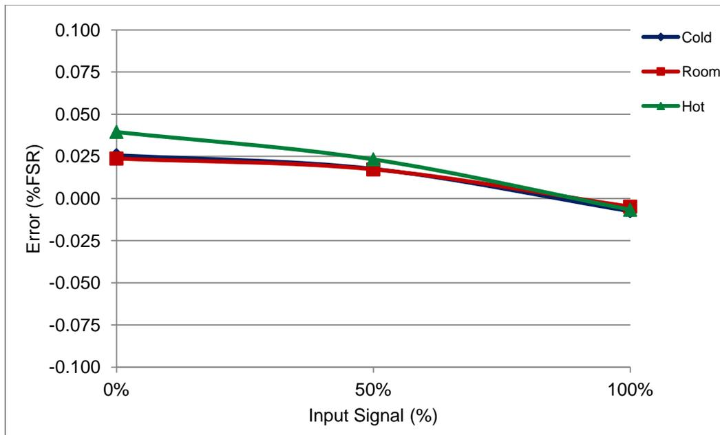
**Figure 13: Module Output Error Test Result**
