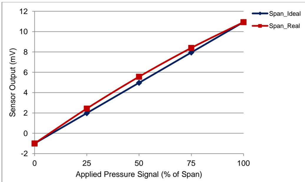
Figure 16: Sensor Output, Ideal vs. +4% Nonlinearity
