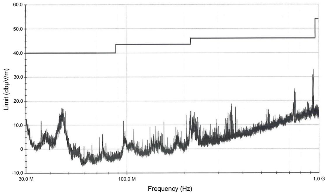
**Figure 23: Radiated EMI Emissions Test - Vertical**
