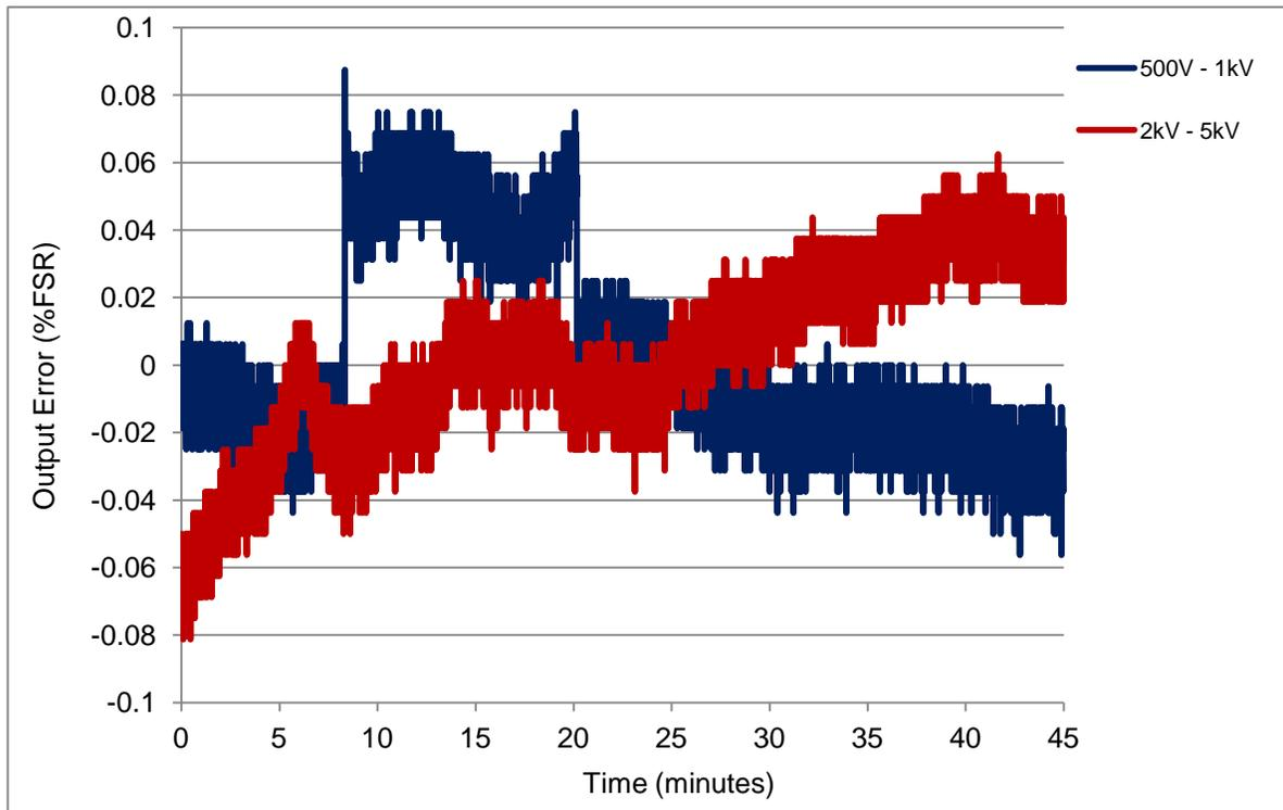
**Figure 21: Module Output Error during Surge Tests**
