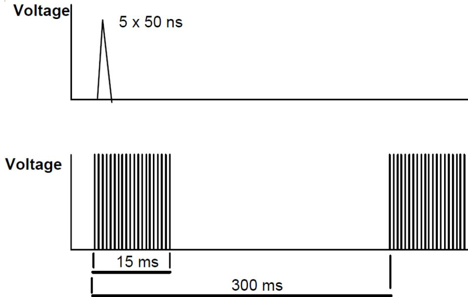
**Figure B-7: IEC 61000-4-4 EFT Voltage Waveform [7]**
