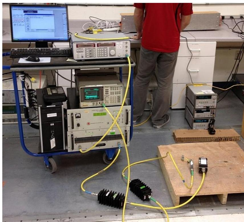
**Figure B-11: IEC 61000-4-6 Conducted EMI Immunity Test Hardware Setup**
