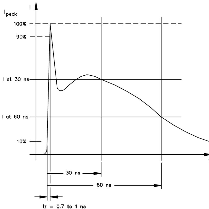
**Figure B-1: IEC 61000-4-2 ESD Current Waveform [7]**
