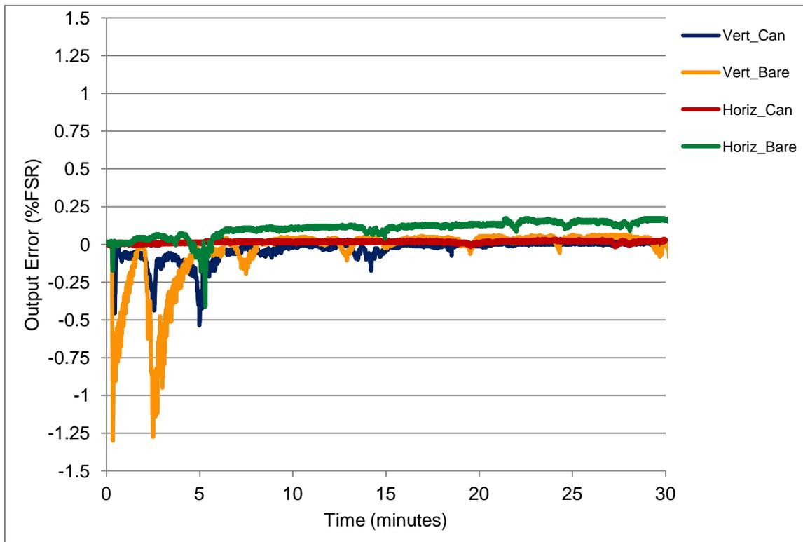
Figure 19: Radiated Immunity Test – 10 V/m
