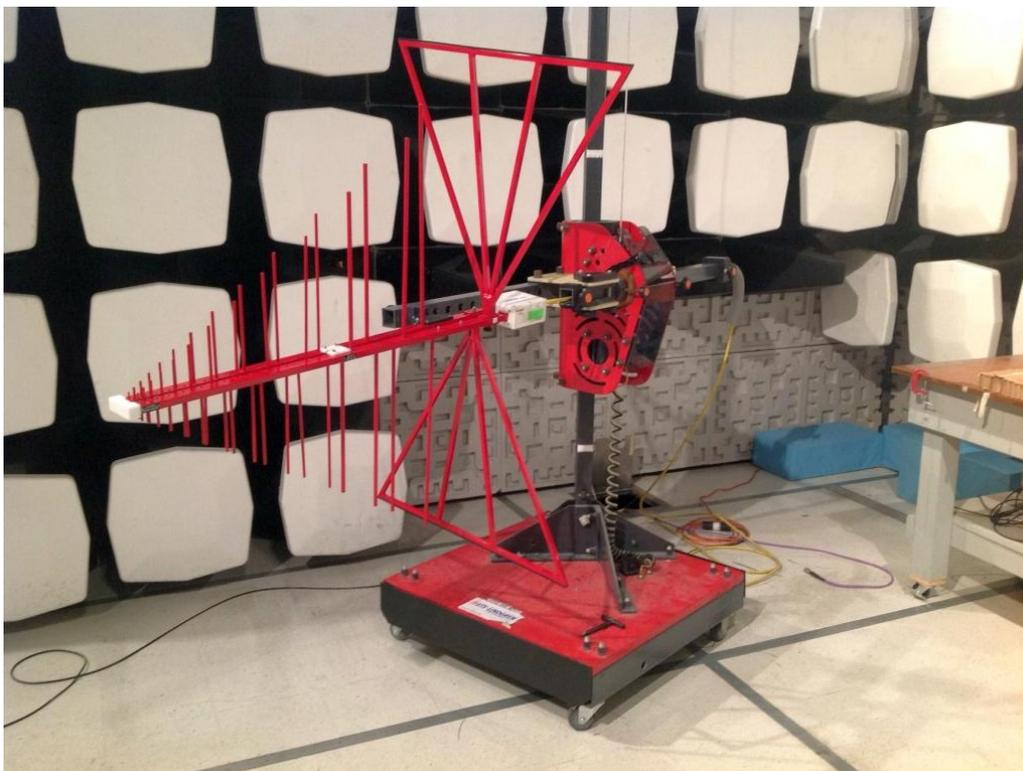
**Figure B-4: Log-Periodic Dipole Antenna – Vertical Orientation**
