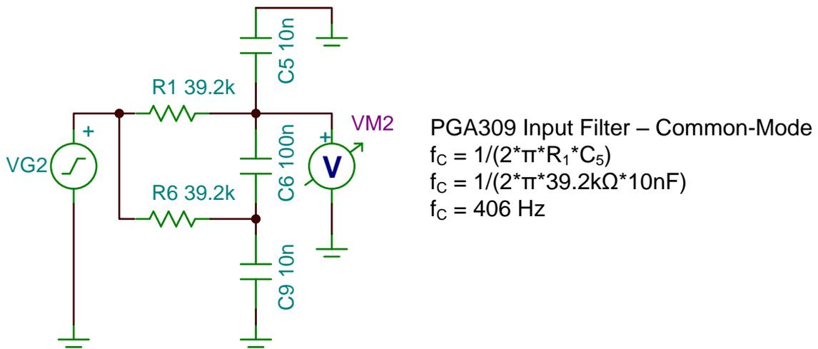
Figure 6: PGA309 Input Filter (Common-Mode) – Schematic
