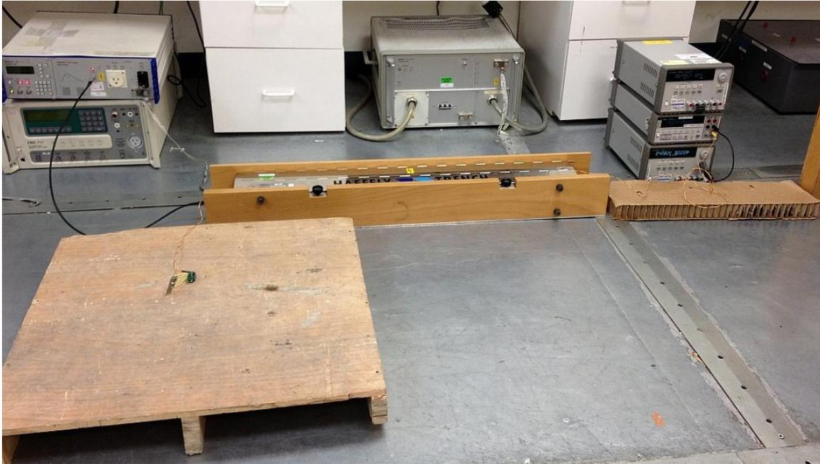
**Figure B-8: IEC 61000-4-4 EFT Test Hardware Setup**
