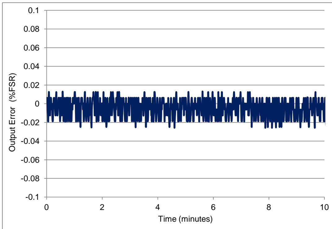
**Figure 20: Module Output Error during EFT Tests**
