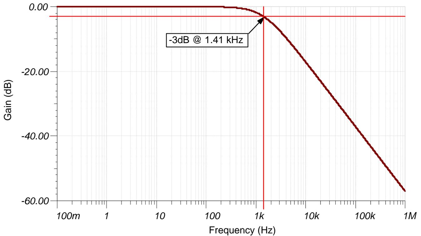
Figure 9: XTR117 Input Filter – Transfer Characteristic
