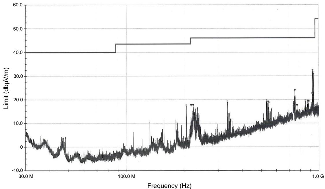
**Figure 24: Radiated EMI Emissions Test - Horizontal**
