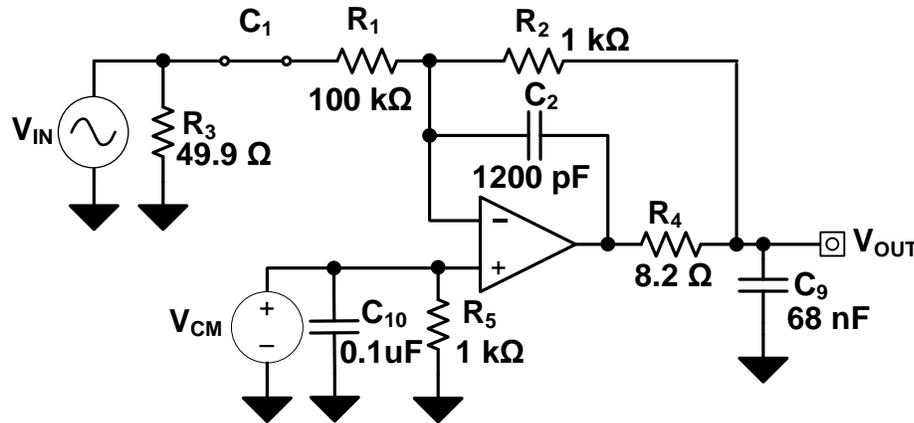
**Figure 3: Simplified attenuator circuit with  $C_1$  shorted**
