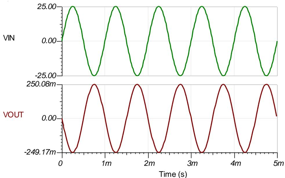
**Figure 9: TINA-TI™ - Large signal attenuation with 50 Vpp input and 500 mVpp output**
