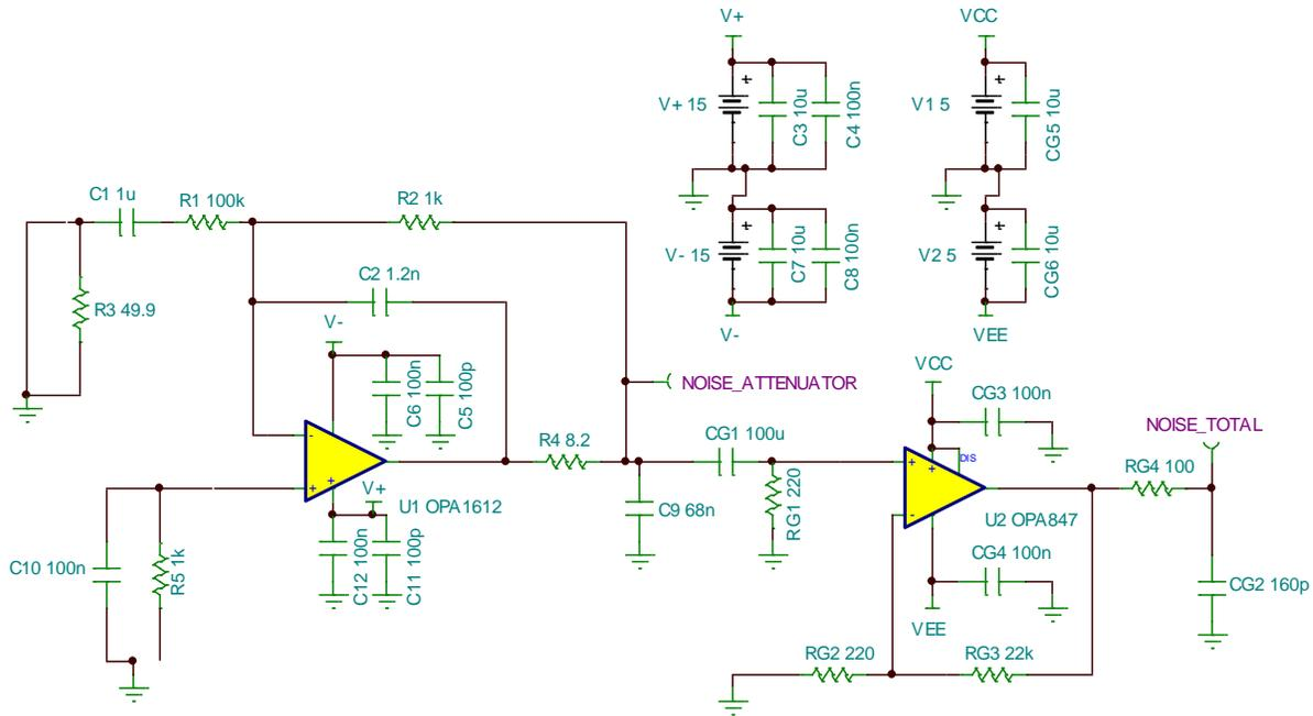
**Figure 18: TINA-TI™ – Attenuator circuit noise measurement test configuration**
