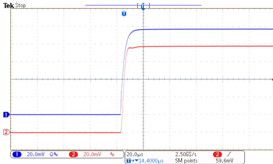
**Figure 16: Measured small signal step response for stability analysis**
