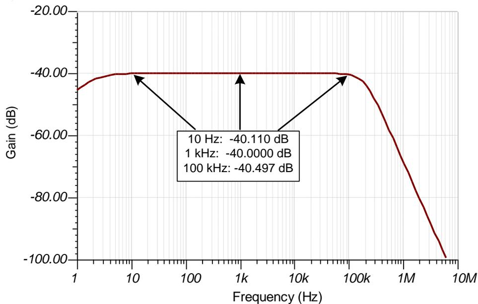
Figure 6: Simulated Full-Scale Transfer Function
