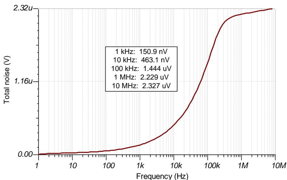
**Figure 11: TINA-TI™ - Total output noise from 1 Hz to 10 MHz**
