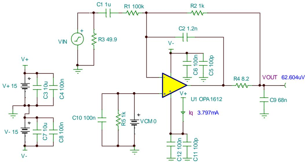
Figure 5: TINA-TI™ simulation schematic showing dc output offset and quiescent current
