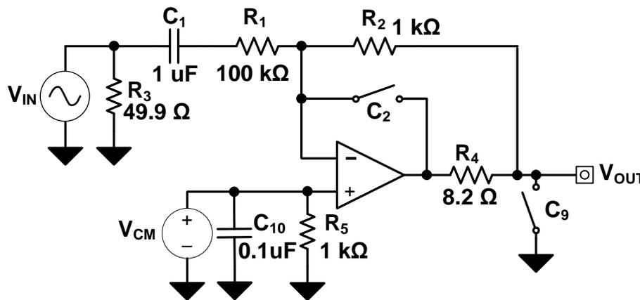
**Figure 4: Attenuator circuit with  $C_2$  and  $C_9$  open**
