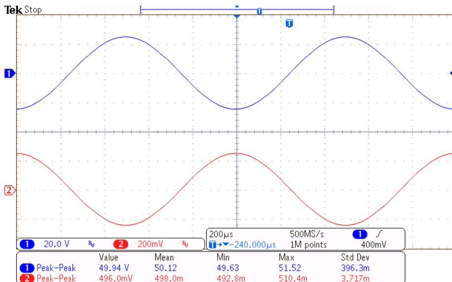
Figure 15: Measured transient response with 50 Vpp input and 500 mVpp output
