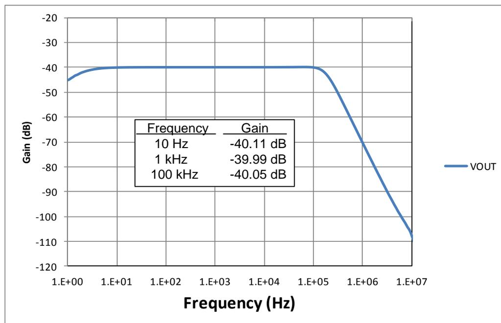
**Figure 1: Measured ac transfer function**
