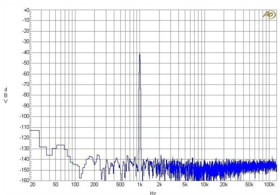
**Figure 17: Measured FFT with 1 kHz 1 Vrms input and 1 Vrms reference**
