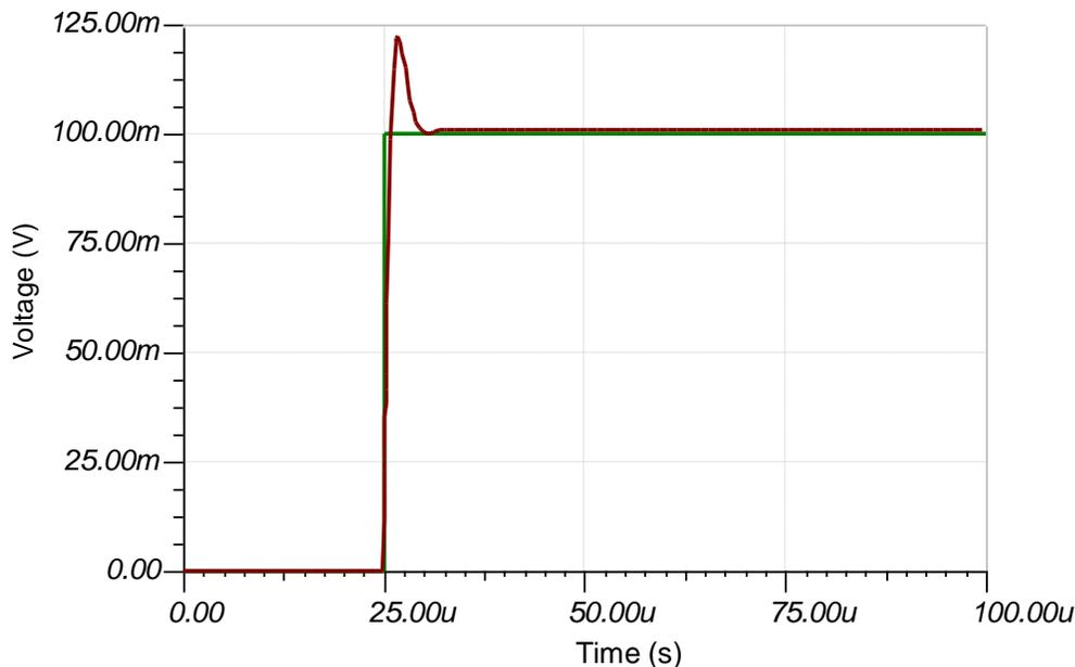
**Figure 10: TINA-TI™ - Small-Signal Step Response Simulation**
