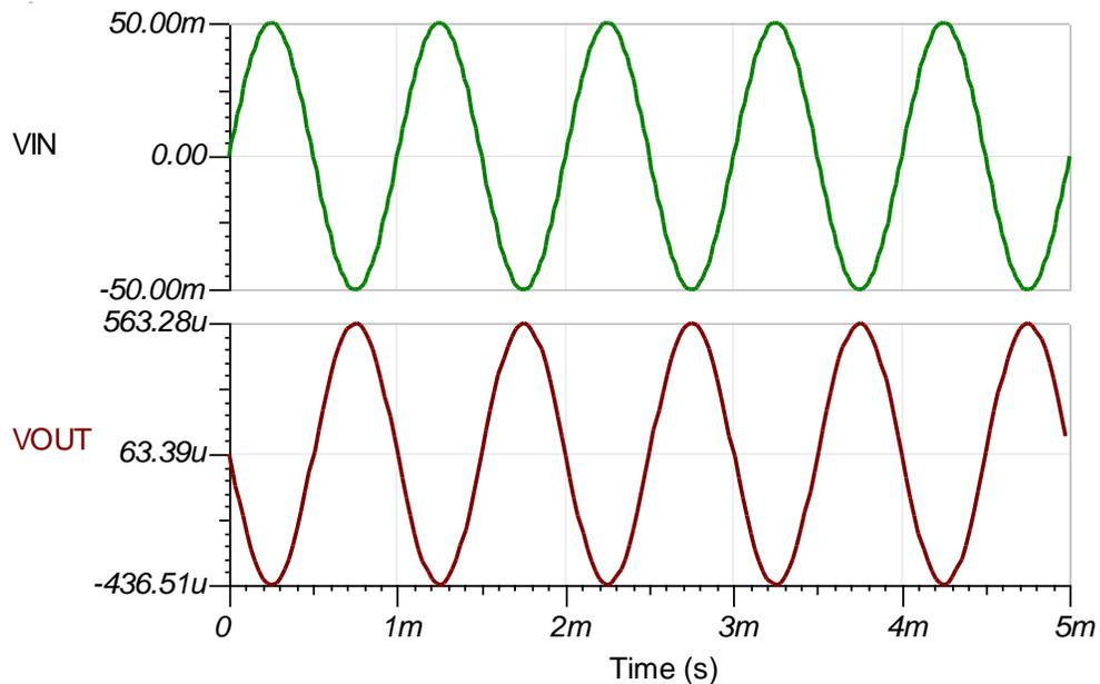
**Figure 8: TINA-TI™ - Low-level signal generation with 100 mVpp input and 1 mVpp output**
