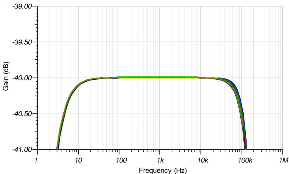
**Figure 7: Simulated Monte-Carlo Full-Scale Transfer Function**
