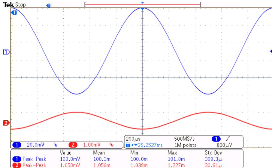
Figure 14: Measured transient response with 100 mVpp input and 1 mVpp output
