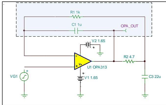
**Figure 17: Dual feedback – OPA313 with 4.7 Ohm isolation resistor**
