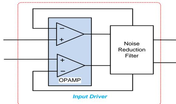
**Figure 11: Buffer driving the input**
