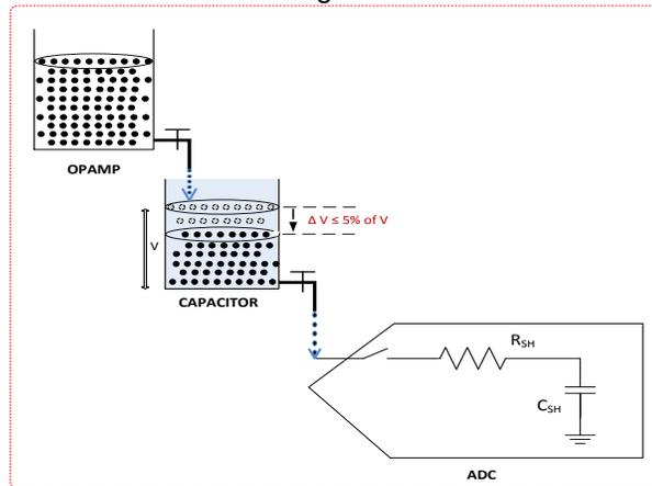
**Figure 10: Fly-wheel capacitor delivering charges to  $C_{SH}$**
