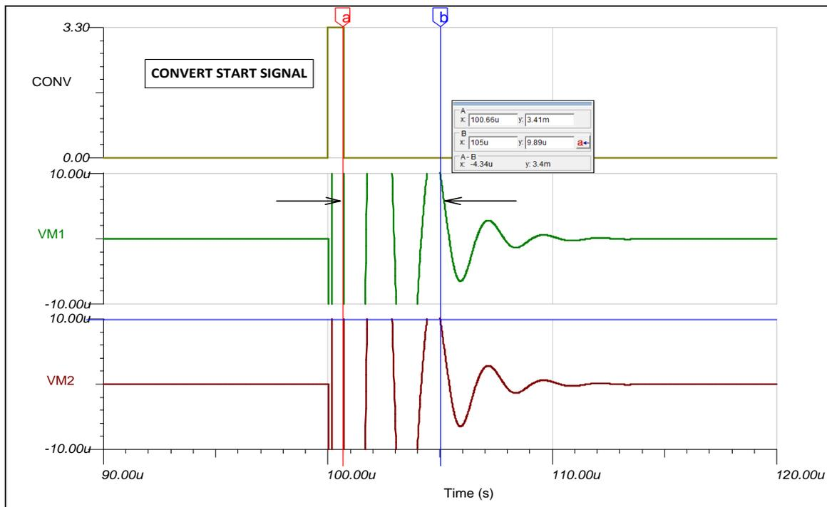
Figure 28 : Op-amp regulating load when sample hold circuit is connected
