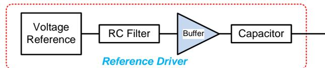
**Figure 7: Buffer for recharging the capacitor**
