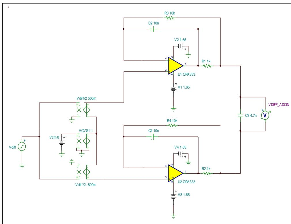
**Figure 31: Noise analysis circuit for input drive**
