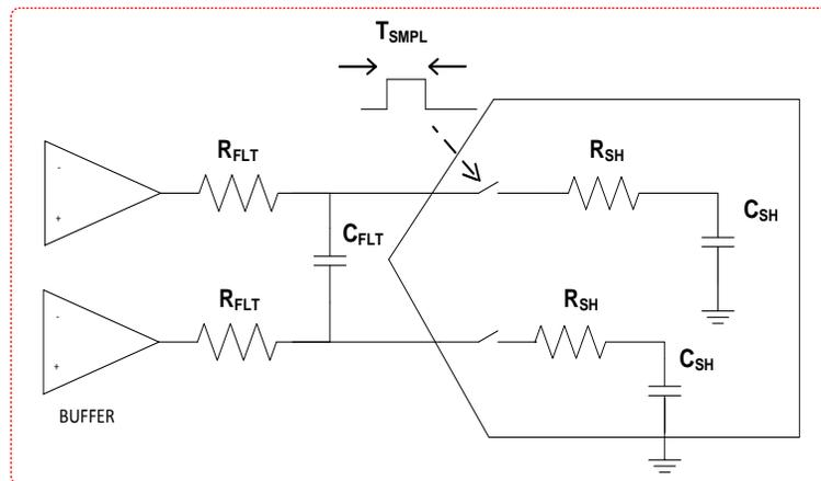
**Figure 9: Input capacitor for attenuating noise**
