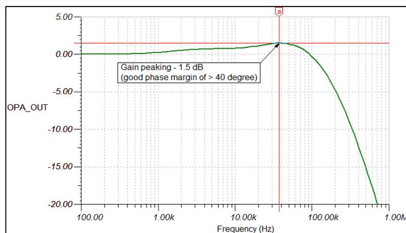
**Figure 18: Gain plot - OPA333 with 1 kOhm isolation resistor**
