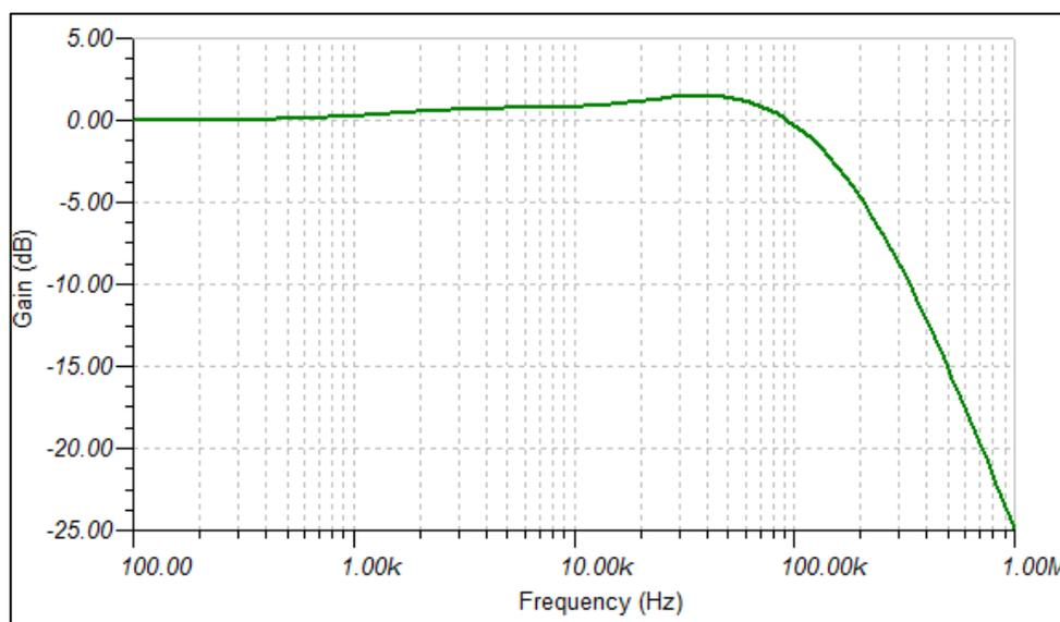
Figure 26: Input buffer stability check gain plot
