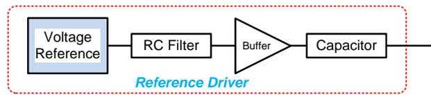
Figure 3: External voltage reference for the converter
