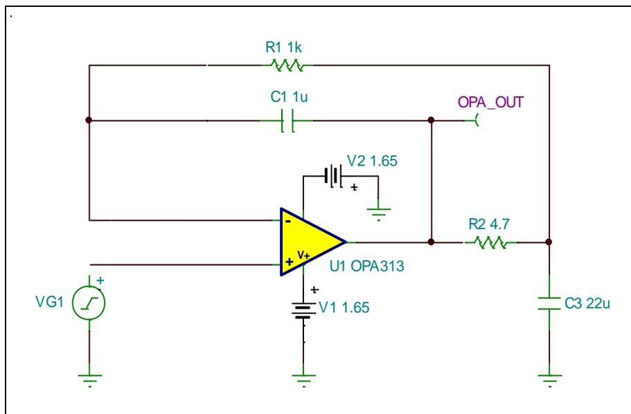
Figure 20: Reference buffer circuit for stability check
