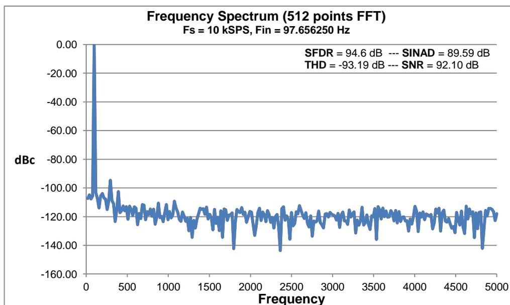
**Figure 1: AC Performance (Measured)**
