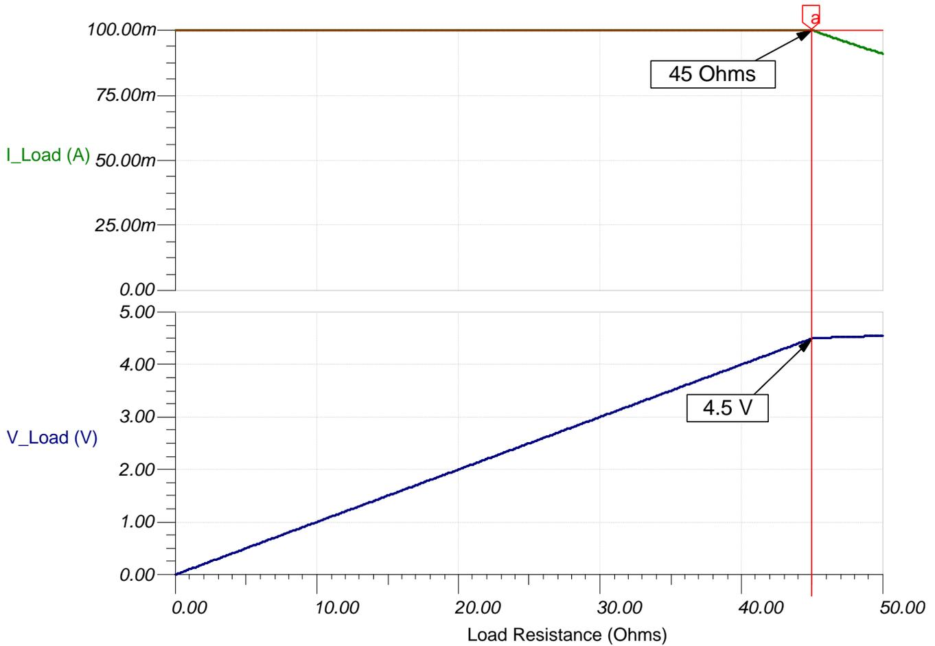
Figure 7. TINA-TI™ - Compliance Voltage and Maximum Load Resistance
