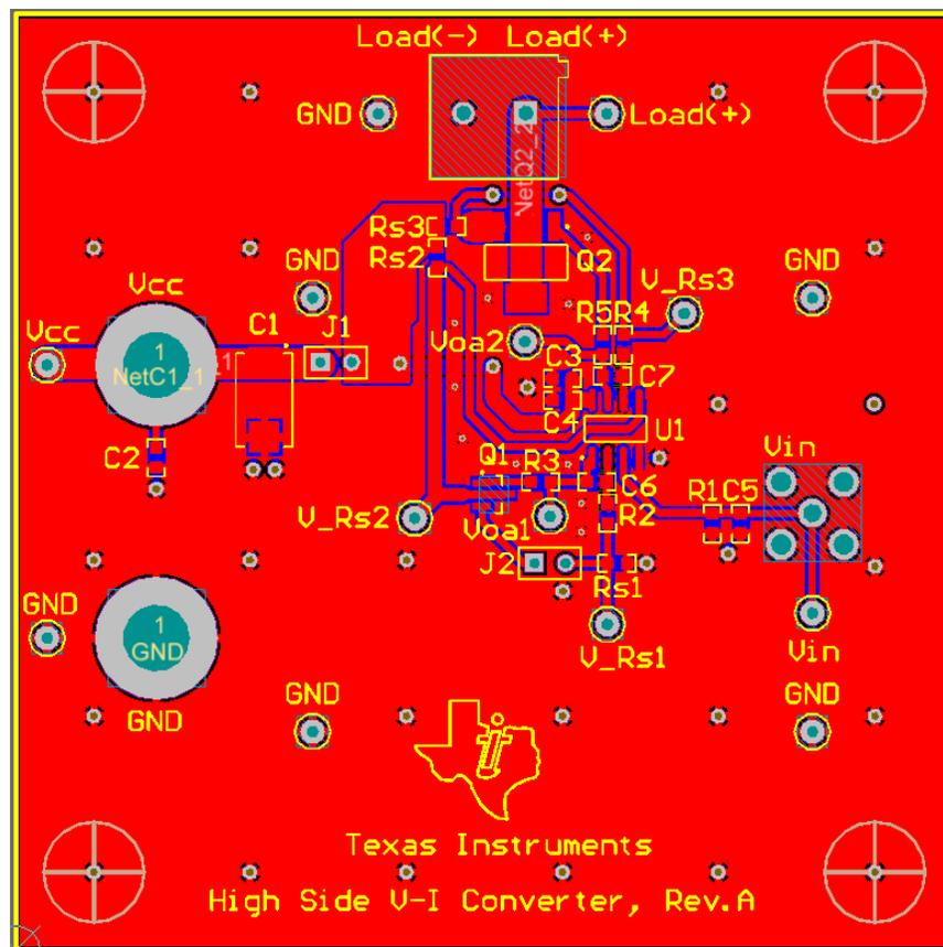
Figure 8. PCB Layout
