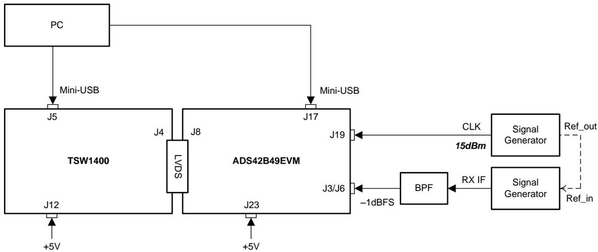
**Figure 3. Test Set-Up Block Diagram**
