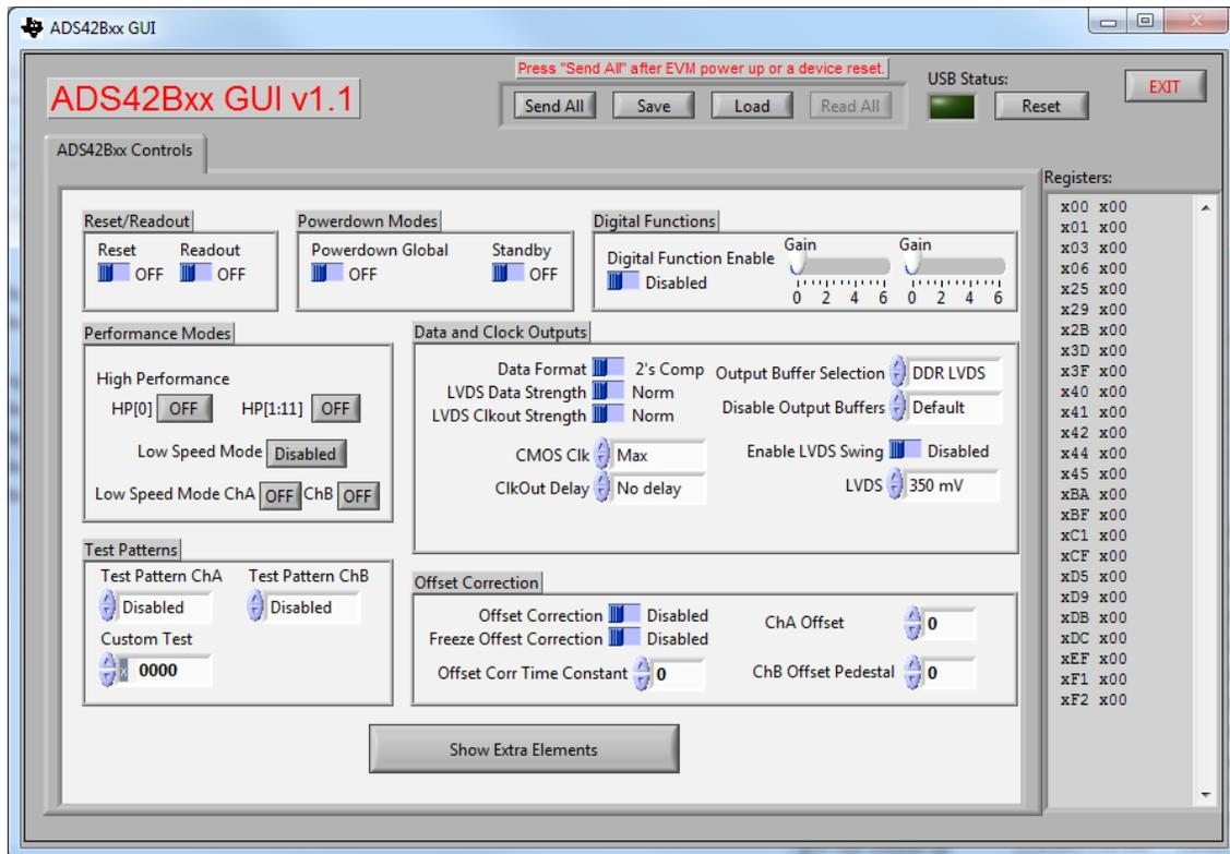
**Figure 1. ADS42Bxx\_GUI Front Panel – Top Level**
