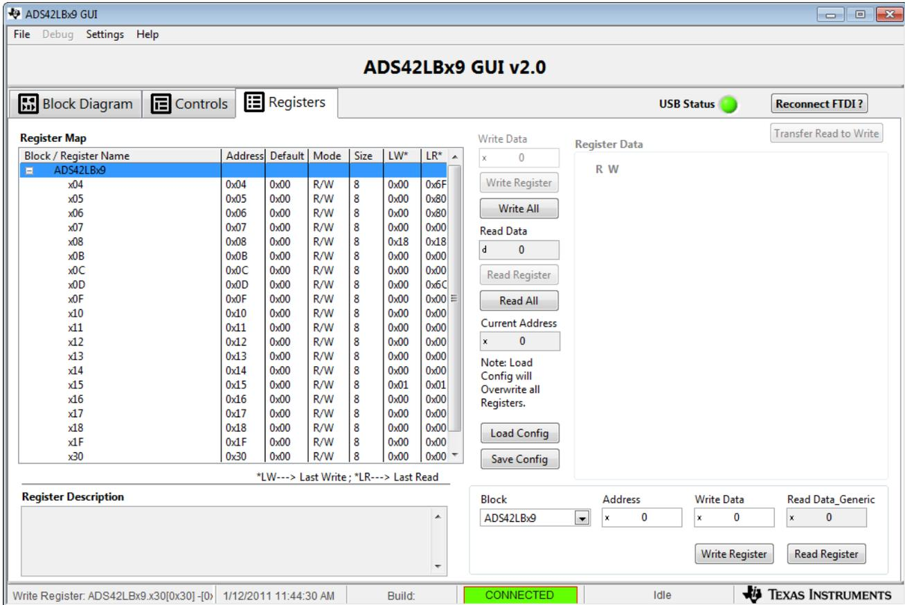
**Figure 4. Registers Tab of the ADS42LBx9 GUI v2.0**
