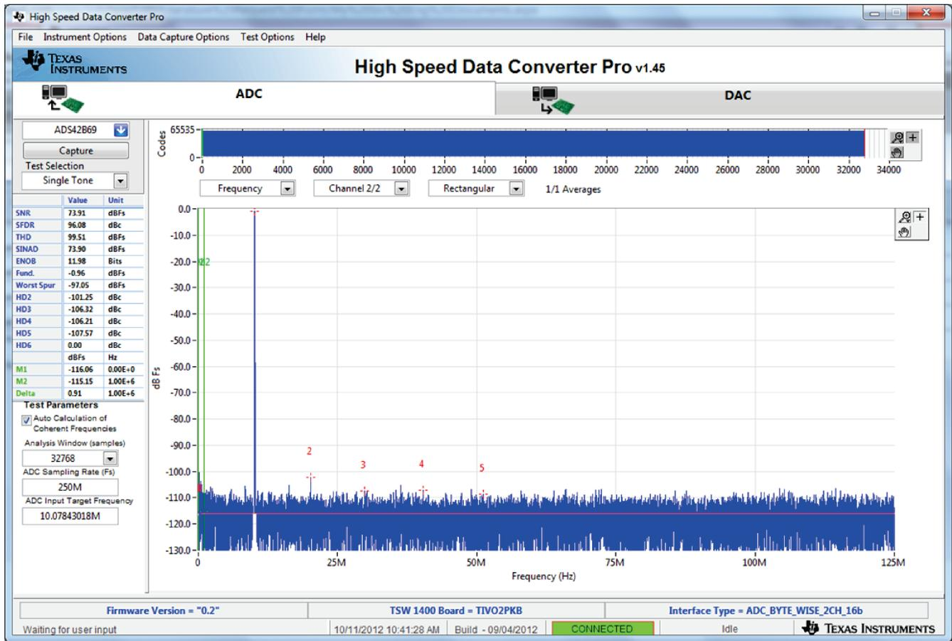
Figure 6. ADS42LB69 Sample Capture using the TSW1400
