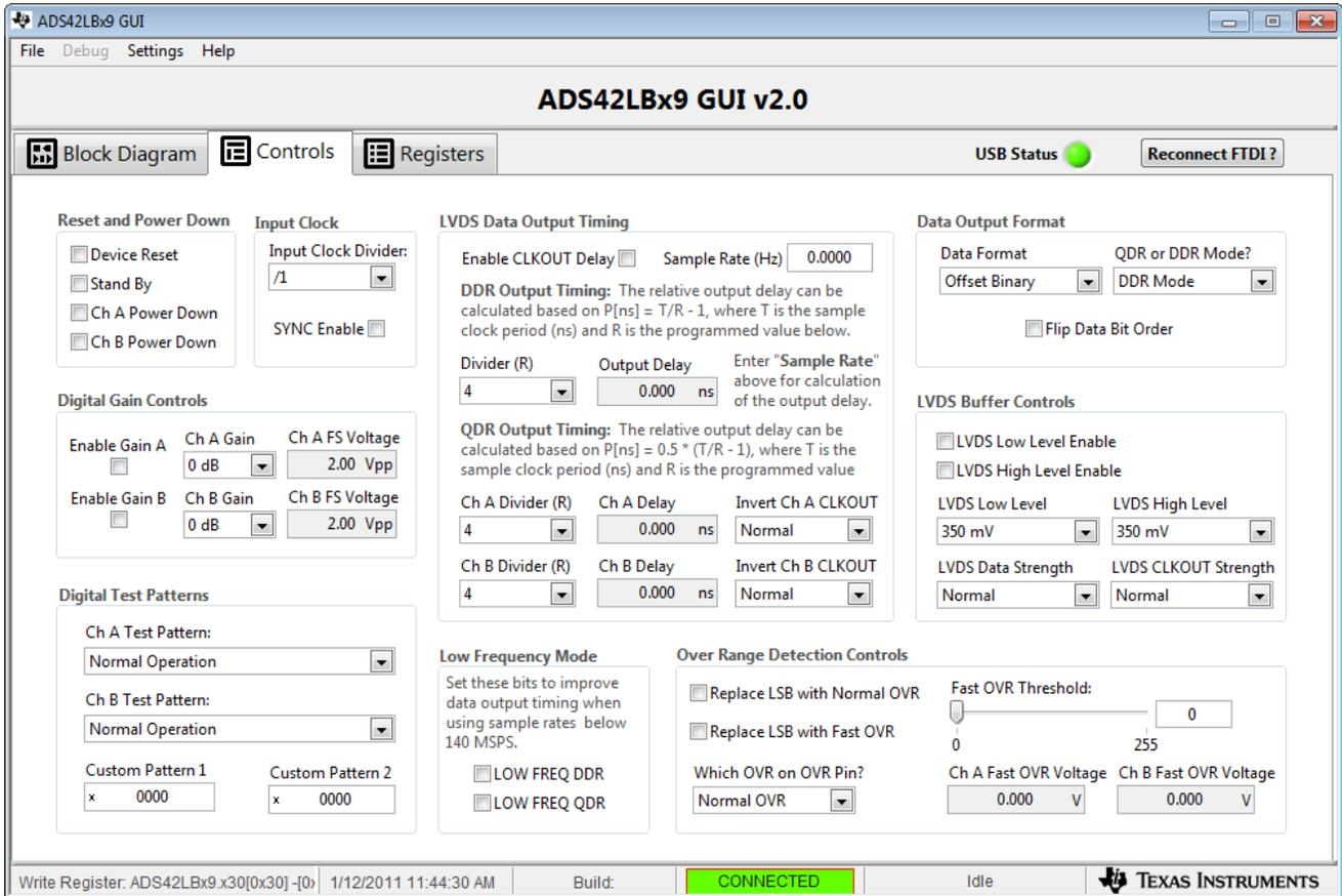
Figure 3. Controls Tab of the ADS42LBx9 GUI v2.0
