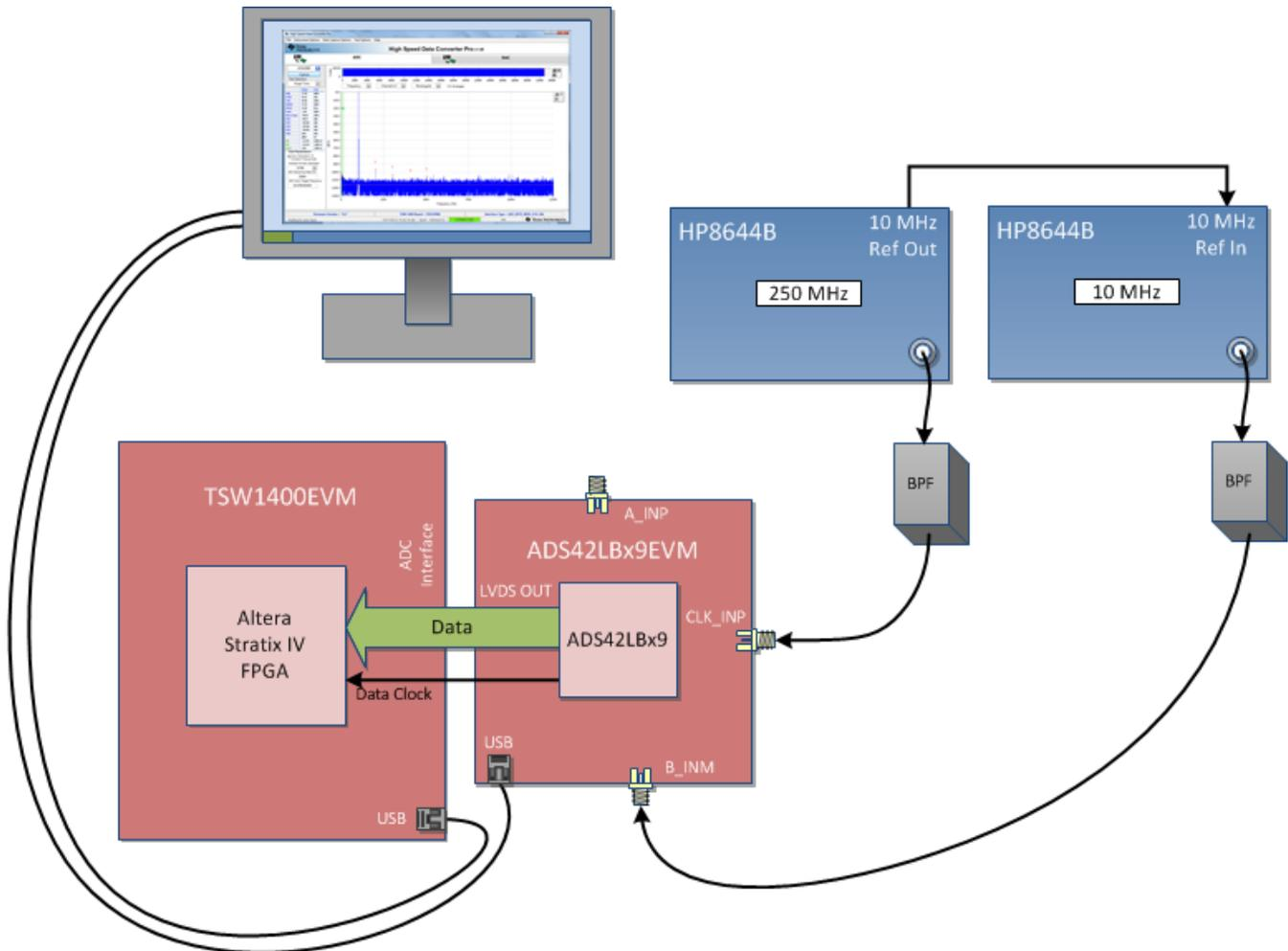
Figure 5. Quick Start Test Setup for the ADS42LBx9EVM
