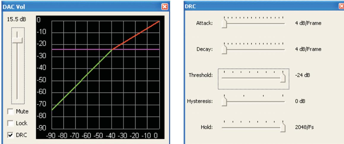
**Figure 11. DRC Transfer Function and DRC Dialog**
