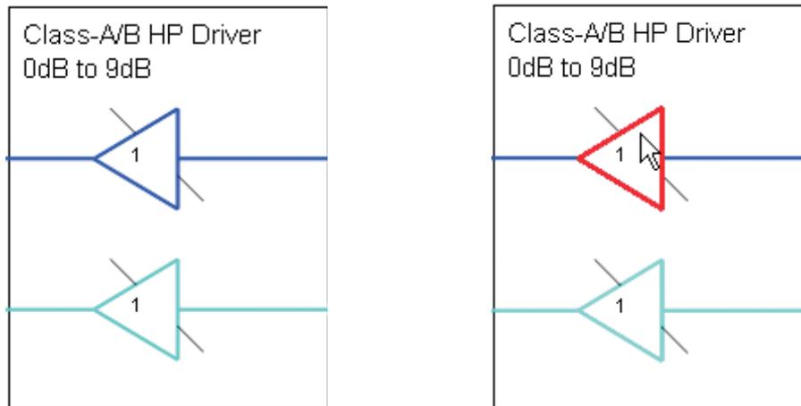
Clicking the activated object will trigger its function. In the case of the amplifier active object, the function is a volume control. Moving the volume control slider changes the volume setting of the amplifier (it is also possible to change the volume by clicking onto the number within the amplifier symbol and typing the new gain setting). The control software updates the appropriate register in the TLV320AIC3111 and as a result the volume on the headphone output will change accordingly.
