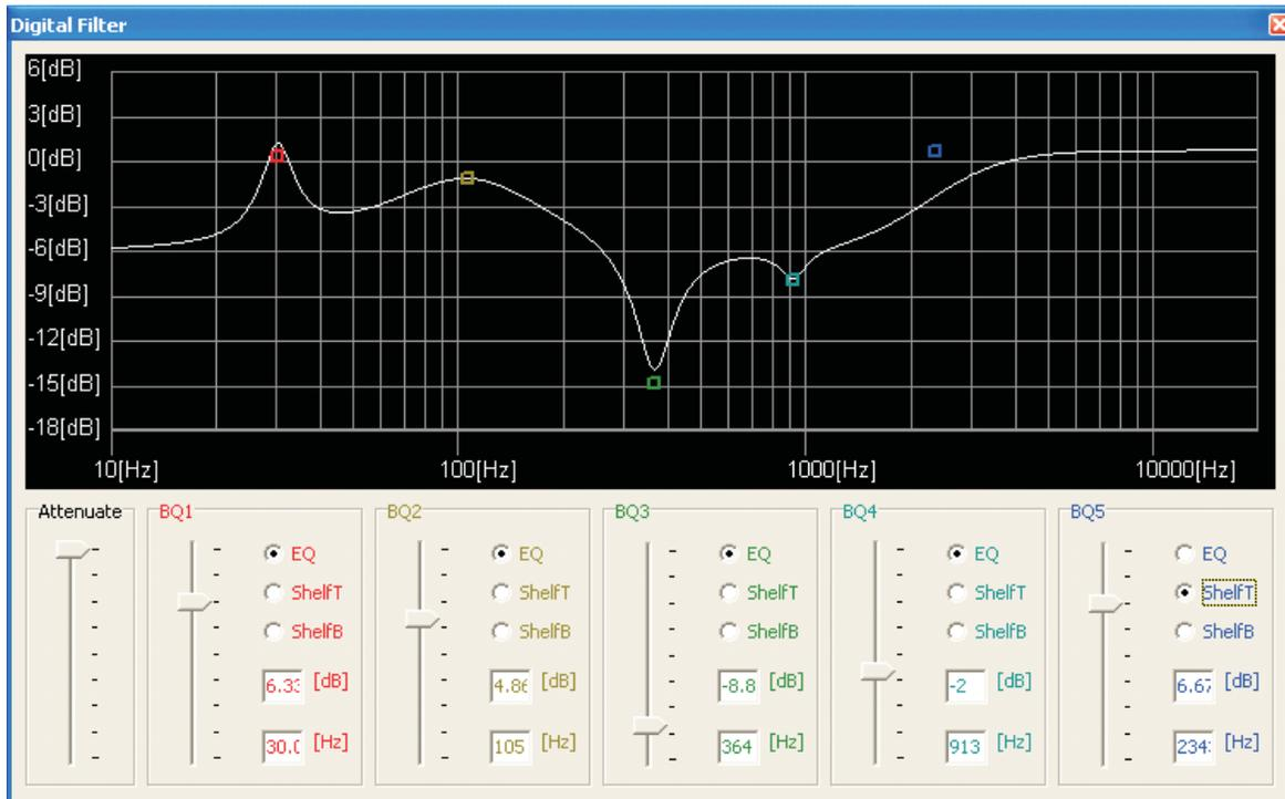
The digital filter dialog limits the range of each digital biquad filter to +/-12[dB] (this is an arbitrary limitation for demonstration purposes).
