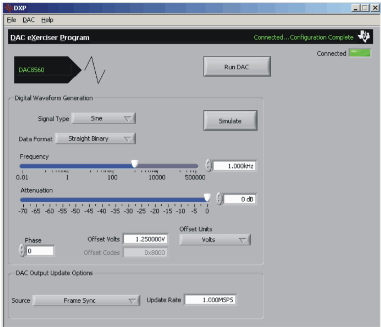
**Figure 13. DAC8560EVM: Frequency/Amplitude and Update Rate Adjustments**
