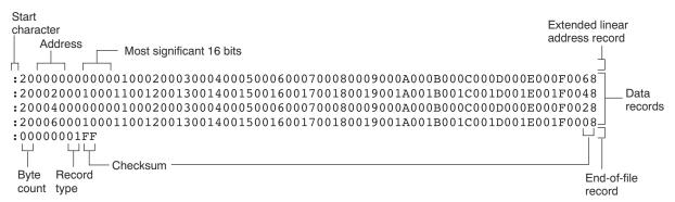
Figure 12-7. Intel Hexadecimal Object Format
