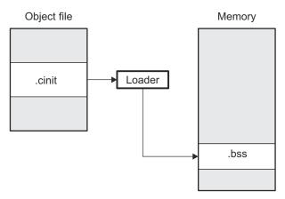
Figure 3-3. Initialization at Load Time
