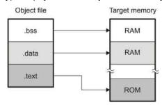
Figure 2-1. Partitioning Memory Into Logical Blocks
