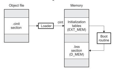
Figure 3-2. Autoinitialization at Run Time
