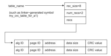
Figure 8-7. CRC\_TABLE Conceptual Model
