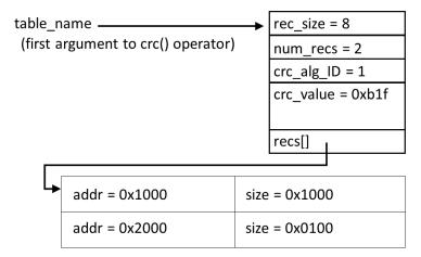
Figure 8-8. CRC Storage Format for Memory Ranges
