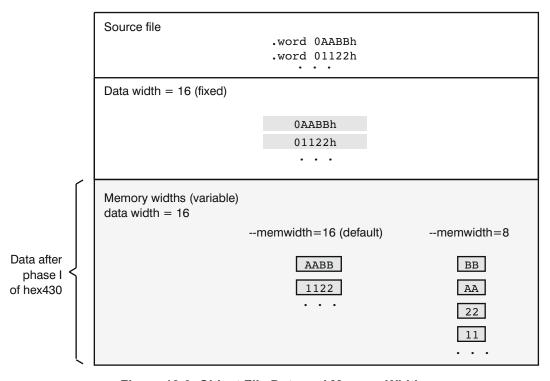
Figure 12-3. Object File Data and Memory Widths
