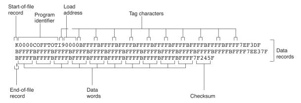
Figure 12-10. TI-Tagged Object Format
