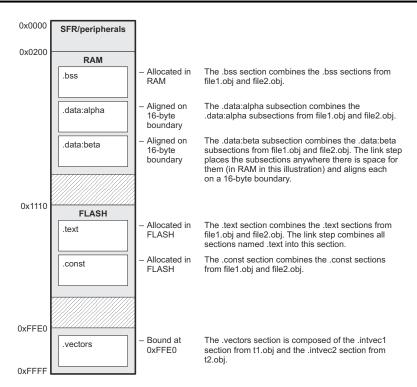
Figure 8-2. Section Placement Defined by The SECTIONS Directive
