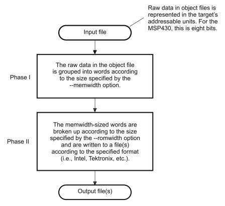
Figure 12-2. Hex Conversion Utility Process Flow
