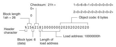
Figure 12-9. Extended Tektronix Object Format
