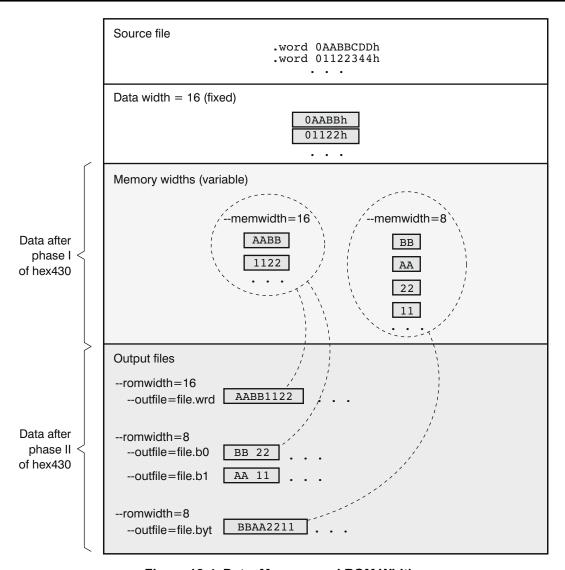
Figure 12-4. Data, Memory, and ROM Widths
