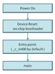
Figure 3-1. Bootloading Sequence (Simplified)
