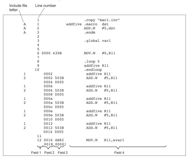
Figure 4-2. Example Assembler Listing
