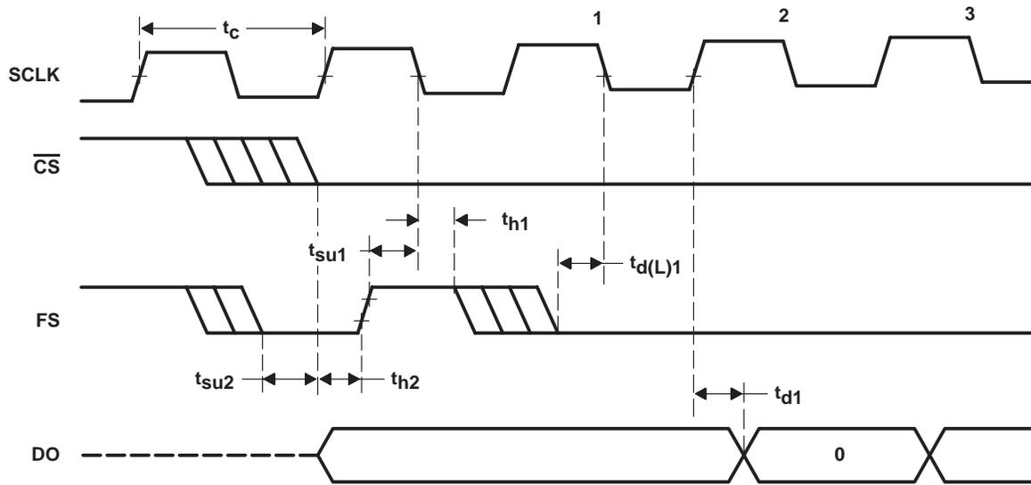
Figure 4–3. Microprocessor Interface Timing (Normal Sample Mode,  $\overline{\text{INV CLK}} = \text{Low}$ )
