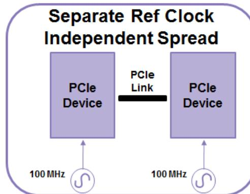
**Figure 2-4. Seperate Clock Architecture**
