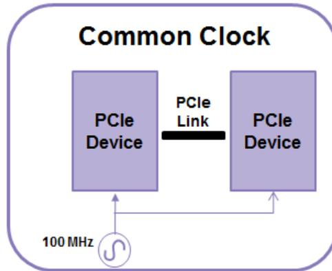
Figure 2-2. Common Clock Architecture
