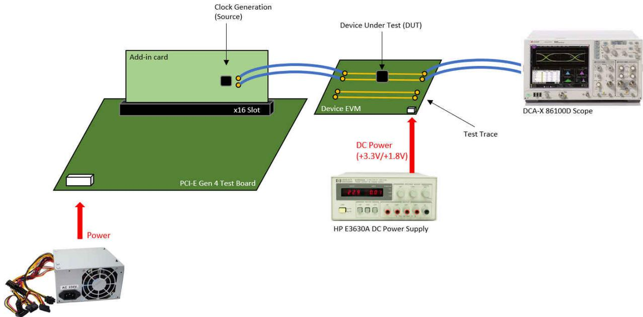
**Figure 3-1. Test Setup for PCIe Reference Clock Measurement**
