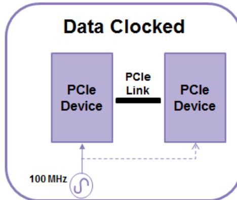
Figure 2-3. Data Clock Architecture
