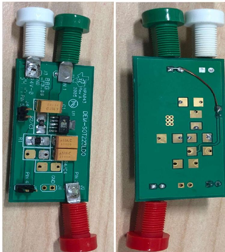
**Figure 3-2. DEM-SOT223LDO Demonstration Fixture Board Top View (Left) and Bottom View (Right)**
