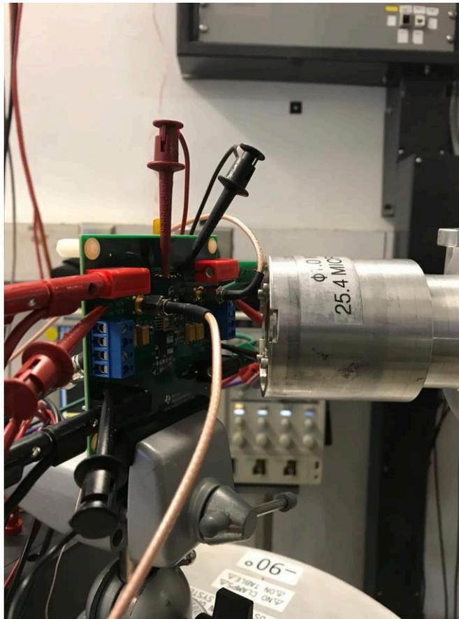
**Figure 4-1. Photograph of the TPS73801-SEP Evaluation Board Mounted in Front of the Heavy-Ion Beam Exit Port**
