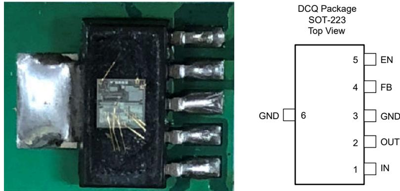
**Figure 3-1. Photograph of Delidded TPS73801-SEP (Left) and Pinout Diagram (Right)**
