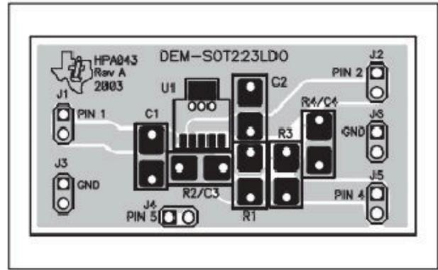
**Figure 3-3. Schematic of the DEM-SOT223LDO Used During SEE Characterization**
