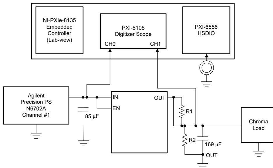
**Figure 5-1. Block Diagram of the Test Setup Used for TPS73801-SEP SEE Characterization**
