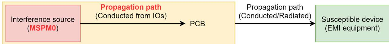
Figure 6-1. Noise Propagation Model for EMI
