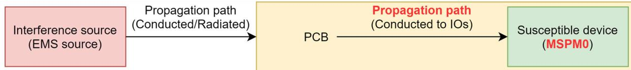
**Figure 5-1. Noise Propagation Model for EMS**
