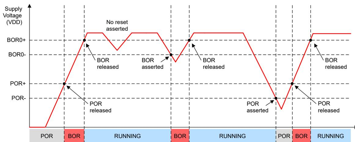
**Figure 4-1. POR, BOR vs. Supply Voltage (VDD)**
