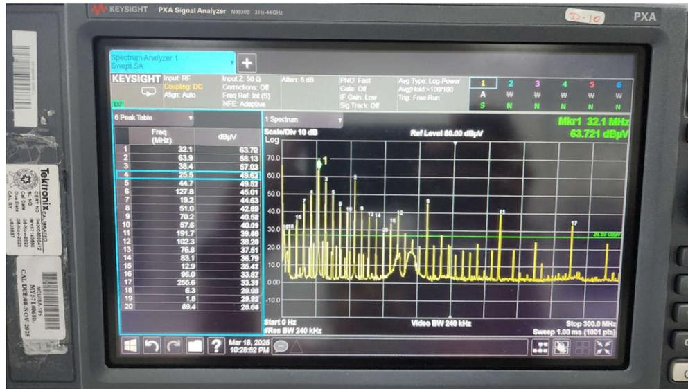
**Figure 6-5. Conducted Noise at Vcore on MSPM0L**
