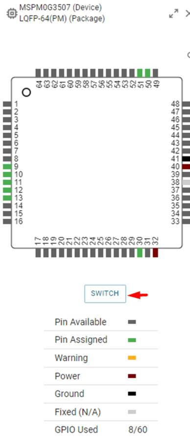
**Figure 9-2. SWITCH Button Location**
