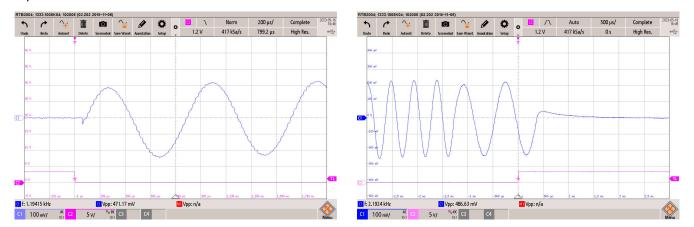
Figure 3-10. HART Carrier Start and Stop Time Test Oscilloscope Results
