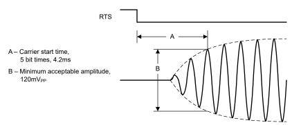
Figure 3-8. Carrier Start Timing
