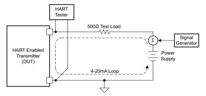
Figure 3-19. Noise Sensitivity Test
