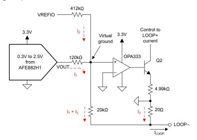
Figure 2-9. Voltage-to-Current Converter Stage for the Transmitter Board
