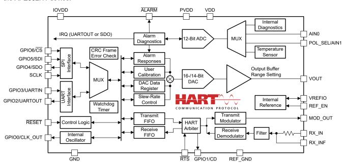
Figure 2-1. AFE882H1 Block Diagram
