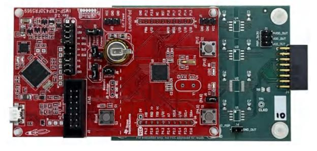
Figure 2-4. MSP-EXP430FR5969 LaunchPad with a LP-DBE Connector Board
