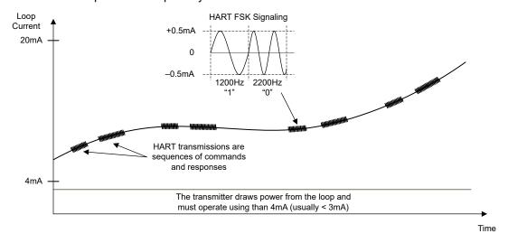
Figure 1-3. The HART FSK Modulated Onto the 4-20mA Current Loop
