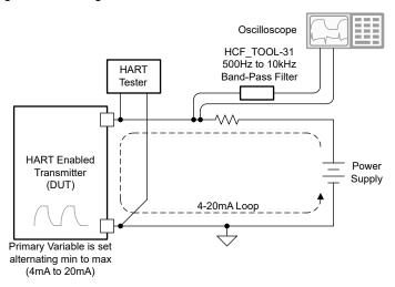
Figure 3-15. HART Analog Rate of Change Test Setup
