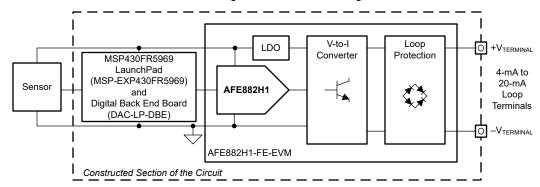
Figure 2-5. Block Diagram of a 2-wire Transmitter Design Using an AFE882H1 Evaluation Module and a Digital-Back-End Board
