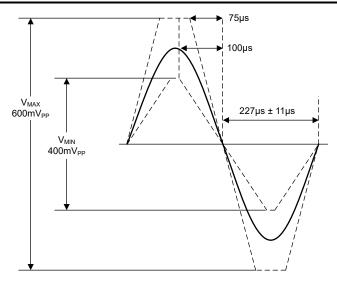
Figure 3-4. HART 2200Hz FSK Waveform Limits
