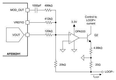
Figure 2-10. Addition of the HART Signal From MOD\_OUT to the V-to-I Stage
