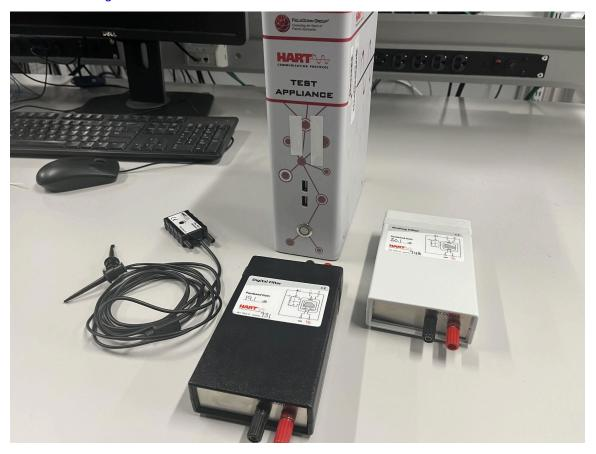
Figure 3-1. HART Test System Shown With an HCF\_TOOL-31, HCF\_TOOL-32, and an FSK Physical Test Interface
