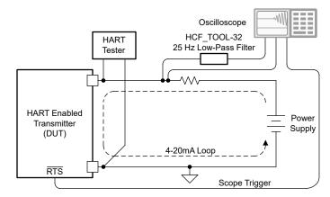
Figure 3-11. HART Carrier Start and Stop Transient Test Setup
