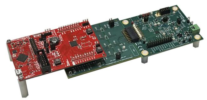
Figure 2-12. HART Transmitter Circuit With AFE882H1-FE-EVM, DAC-LP-DBE, and MSP430 LaunchPad
