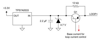
Figure 2-8. Transmitter Board Startup Circuit
