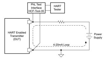
Figure 3-20. HART Carrier Detect Test Setup
