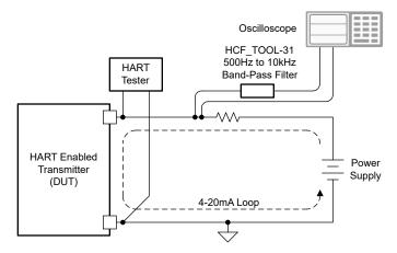
Figure 3-13. HART Output Noise During Silence Test Setup
