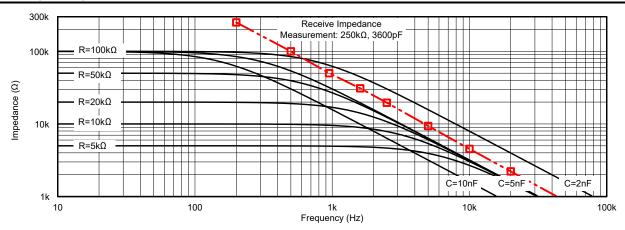
Figure 3-18. Receive Impedance Test Results Plotted Over Frequency
