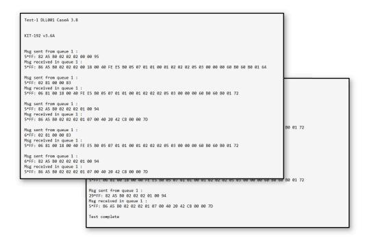
Figure 3-21. HART Sniffer Display From the HART Tester
