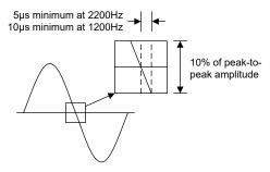
Figure 3-5. HART Sinusoidal Signaling Transition
