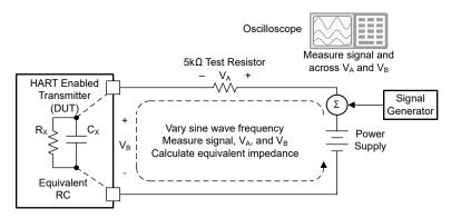
Figure 3-17. HART Receive Impedance Test Setup
