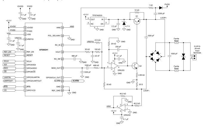
Figure 2-6. 2-Wire Transmitter Design Using an AFE882H1 Circuit Schematic
