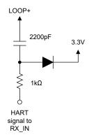
Figure 2-11. RX\_IN Clamp Circuit for Over-Voltage Protection
