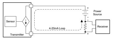
Figure 1-1. Components of the 4-20mA Loop
