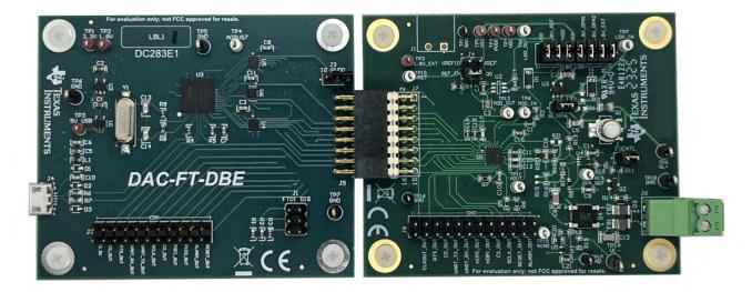
Figure 2-2. AFE882H1 Evaluation Module with an FTDI Digital-Back-End Board
