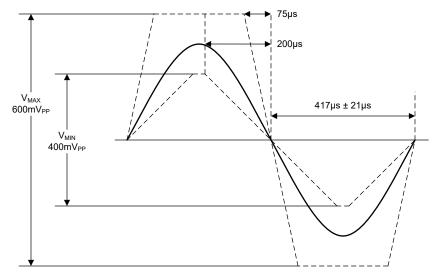
Figure 3-3. HART 1200Hz FSK Waveform Limits
