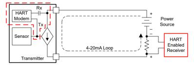
Figure 1-2. Adding HART to the 4-20mA Loop
