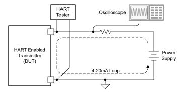
Figure 3-2. HART FSK Sinusoid Test Block Diagram
