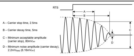
Figure 3-9. Carrier Stop Timing
