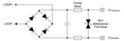
Figure 2-7. Input Protection Circuit at the Input Terminals of the Board
