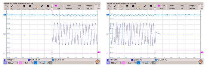
Figure 3-12. HART Carrier Start and Stop Time Transient Test Oscilloscope Results
