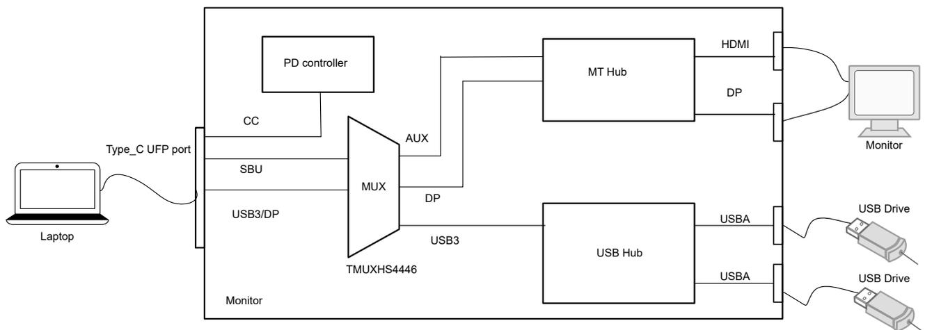
Figure 3-2. Typical Type-C Alt Mode Sink Application
