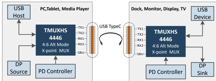
**Figure 2-1. USB Type-C Source and Sink Applications**
