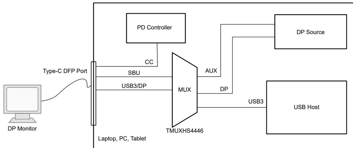
Figure 3-1. Type-C Alt Mode Source Application
