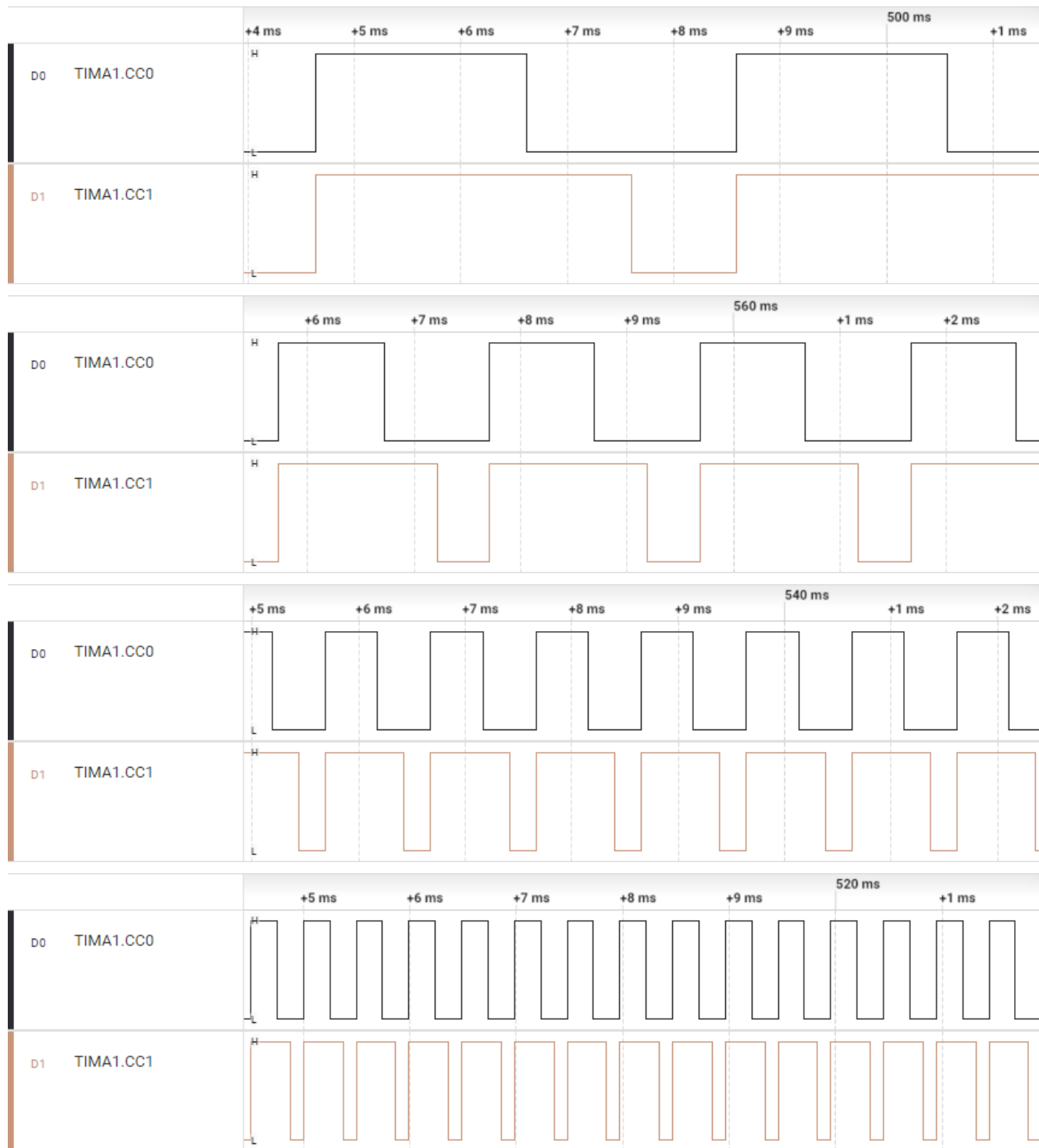
Figure 7-2. 50% Duty Cycle With Frequency Varying Between 250Hz, 500Hz, 1kHz, and 2kHz
