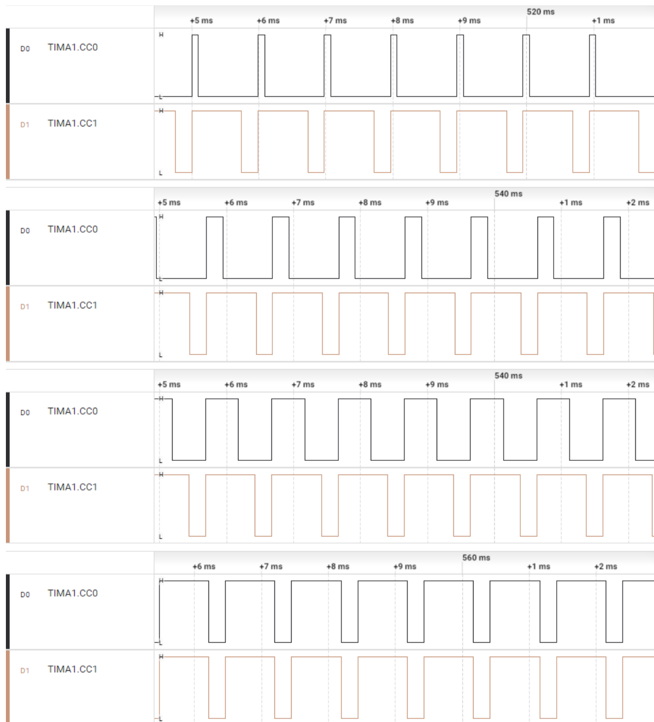
Figure 7-1. 1kHz Frequency With Duty Cycle Varying Between 10%, 25%, 50%, and 75%
