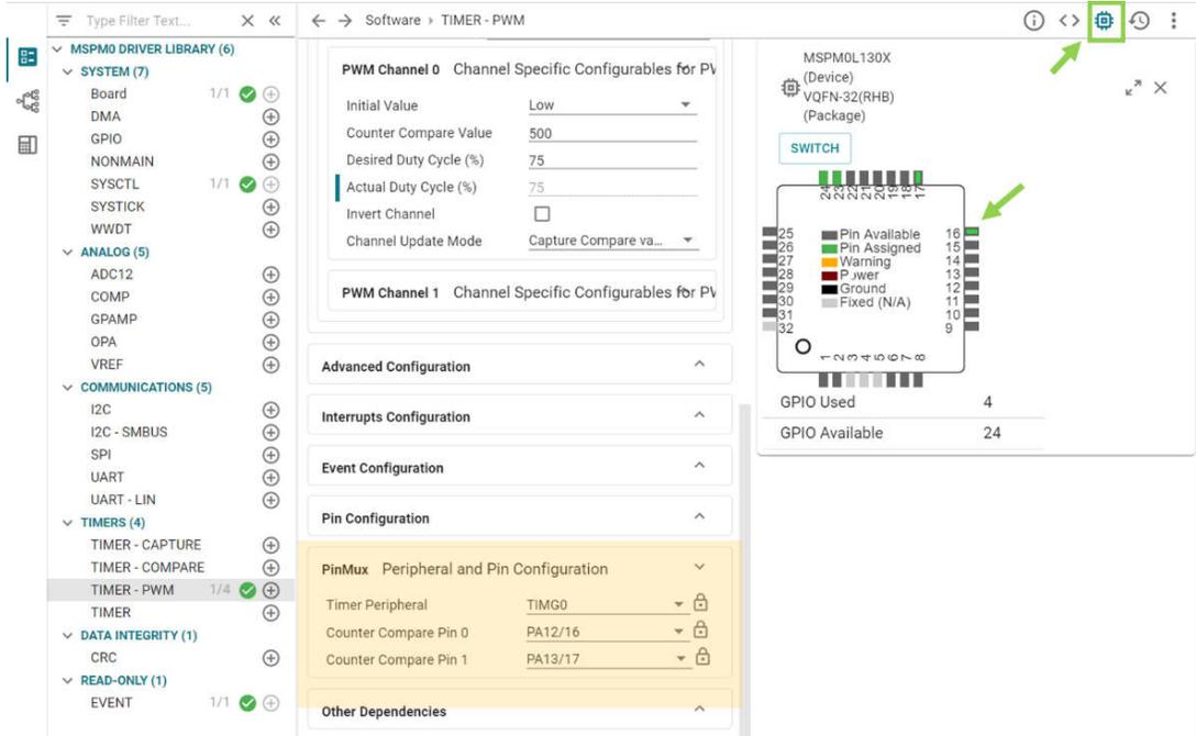
Figure 2-43. Pins Configuration
