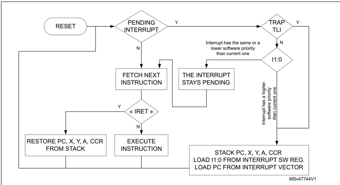
Figure 3-3. Interrupt Processing Flowchart
