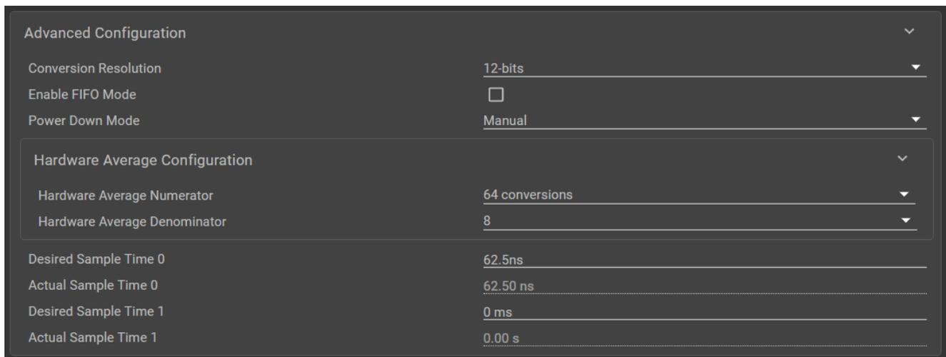
**Figure 3-2. SysConfig ADC Configurations Settings for Oversampling**
