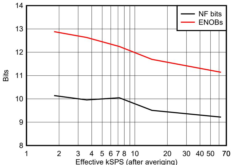
Figure 4-2. Effective Resolution vs the Effective Sampling Rate [kSPS]
