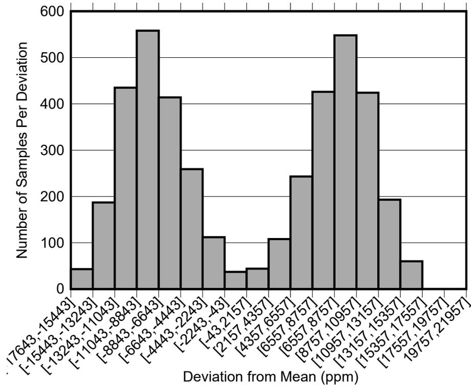
**Figure 4-1. Histogram of ADC Samples When Using Standard Chopping While ADC Averaging**
