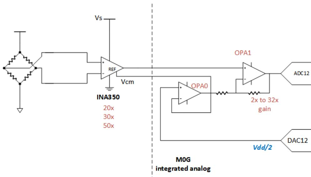
Figure 3-3. Bipolar High-Gain Signal Chain Using the Internal DAC
