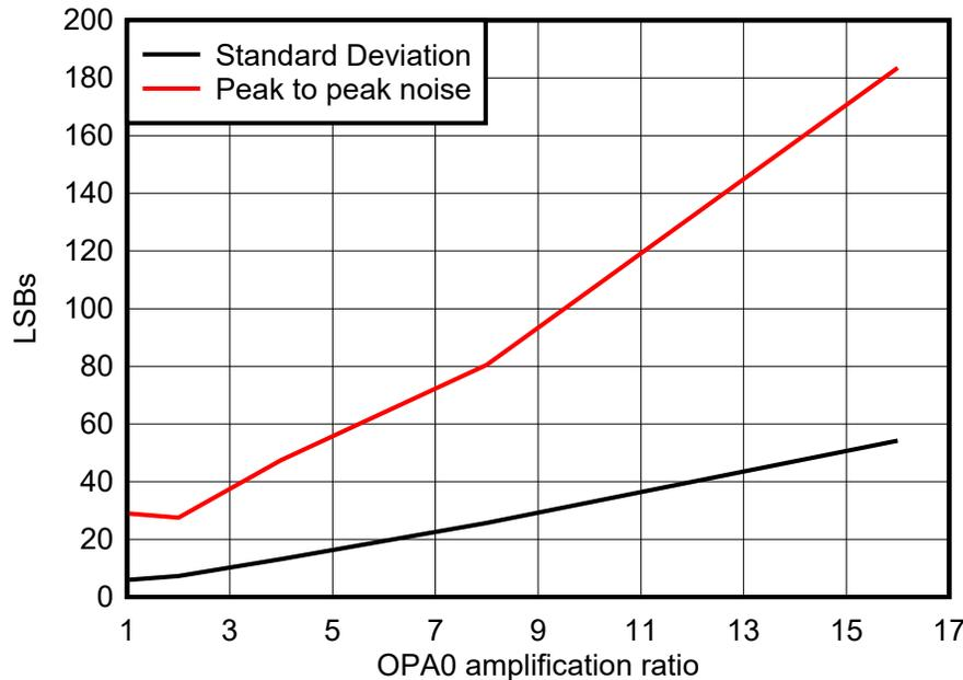
**Figure 4-3. Noise and Effective Resolution vs Amplification Factor of the Internal OPA**
