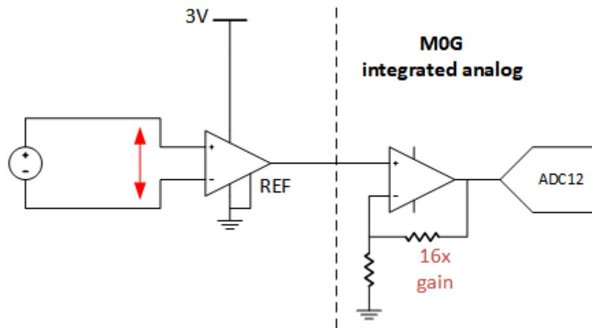
**Figure 3-1. Signal Chain Using INA350 and MSPM0 Internal OPA**
