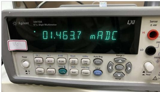
**Figure 4-3. Operating Current of MCU in run0 Mode**
