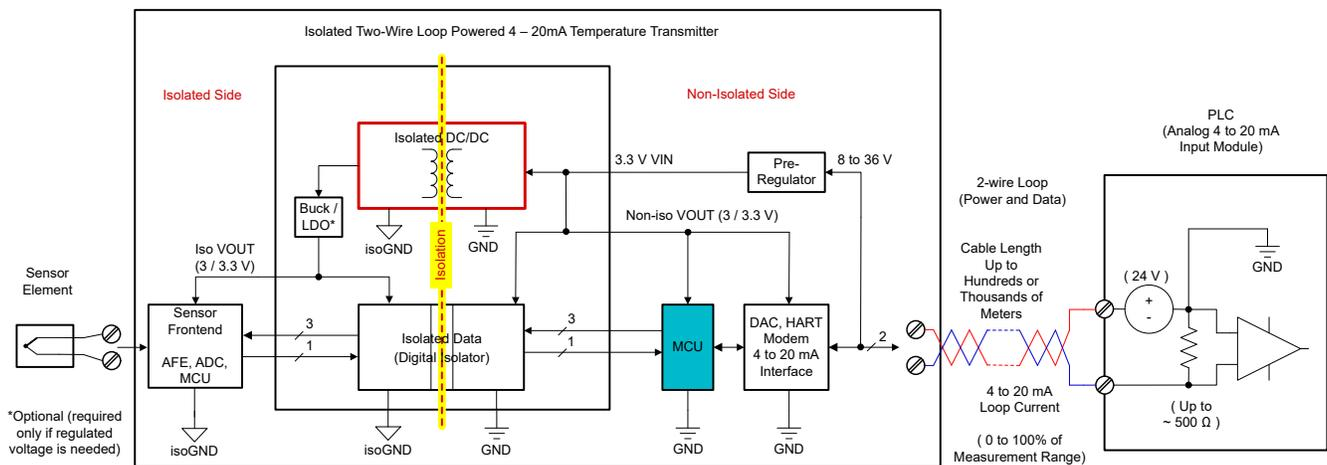
**Figure 1-1. Isolated Two-Wire Loop-Powered 4 to 20mA Temperature Transmitter Control System**
