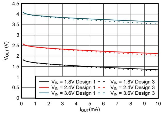
**Figure 1-8. VOUT vs IOU of Design 1 and Design 3 at 50kHz Switching Frequency**
