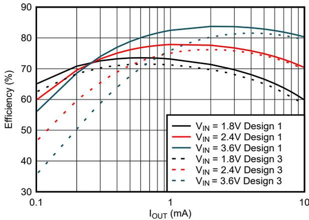
**Figure 1-7. Efficiency Test Results of Design 1 and Design 3 at 50kHz Switching Frequency**
