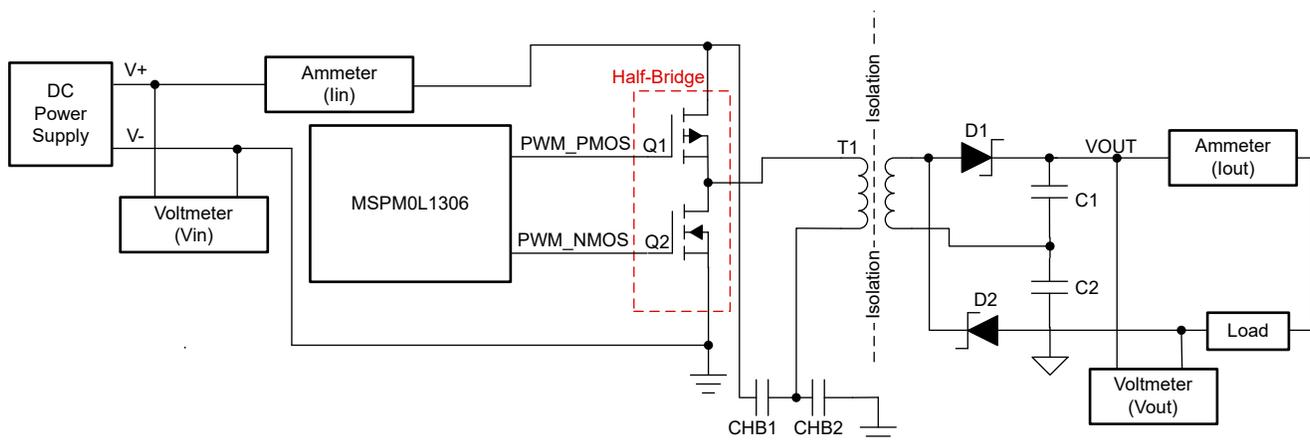
**Figure 1-6. Set Up of Efficiency Test**
