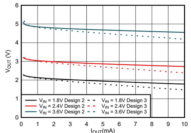
**Figure 1-10. VOUT vs IOU of Design 2 and Design 3 at 250kHz Switching Frequency**
