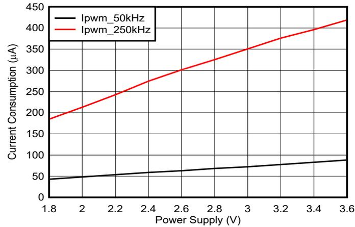
**Figure 1-5. Current Consumption versus Power Supply Voltage at Different PWM Frequency of MSPM0L1306**
