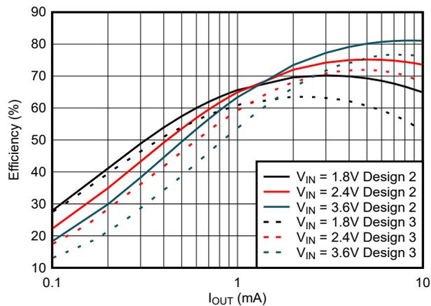
**Figure 1-9. Efficiency Test Results of Design 2 and Design 3 at 250kHz Switching Frequency**
