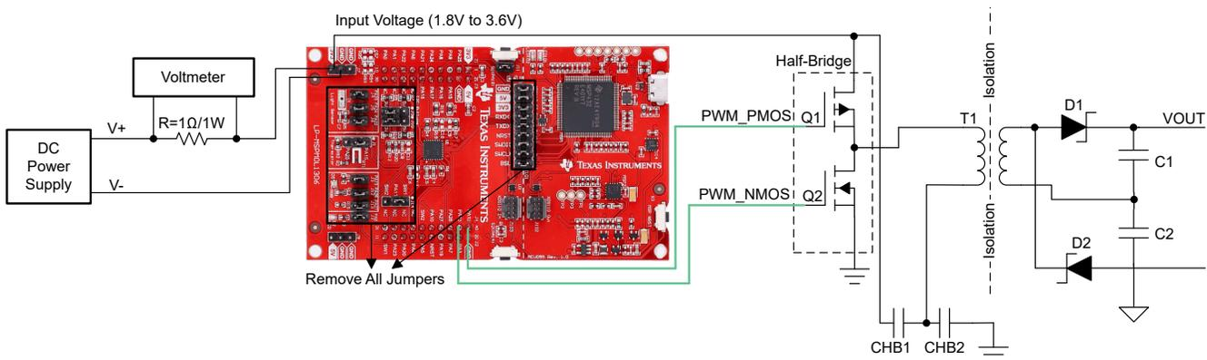
**Figure 1-4. Set Up of Current Consumption Test on MSPM0L1306 EVM Board**
