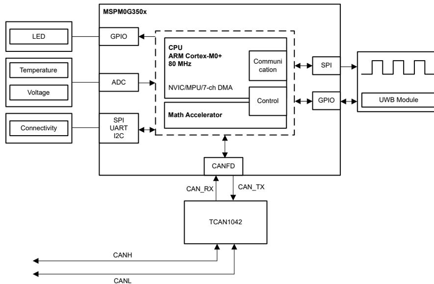
**Figure 3. Block Diagram of UWB PEPS System Based on MSPM0G350x**
