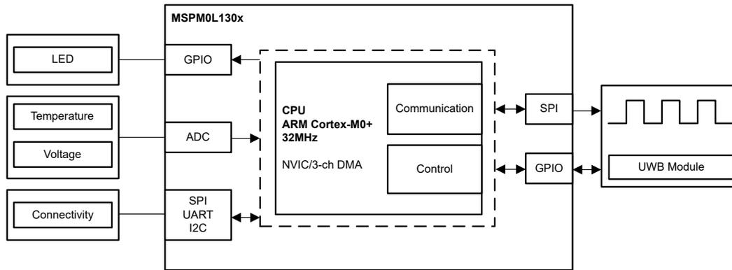
**Figure 2. Block Diagram of UWB PEPS System Based on MSPM0L130x**
