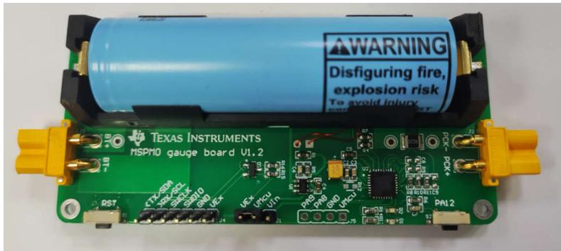
**Figure 1-1. MSPM0 Current Detection Hardware Board**
